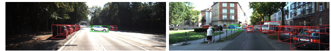
Fig. 12: Example synthetic images generated by [58]. Red bounding boxes show original ground truths, while green boxes illustrate the rendered meshes from CAD models.
