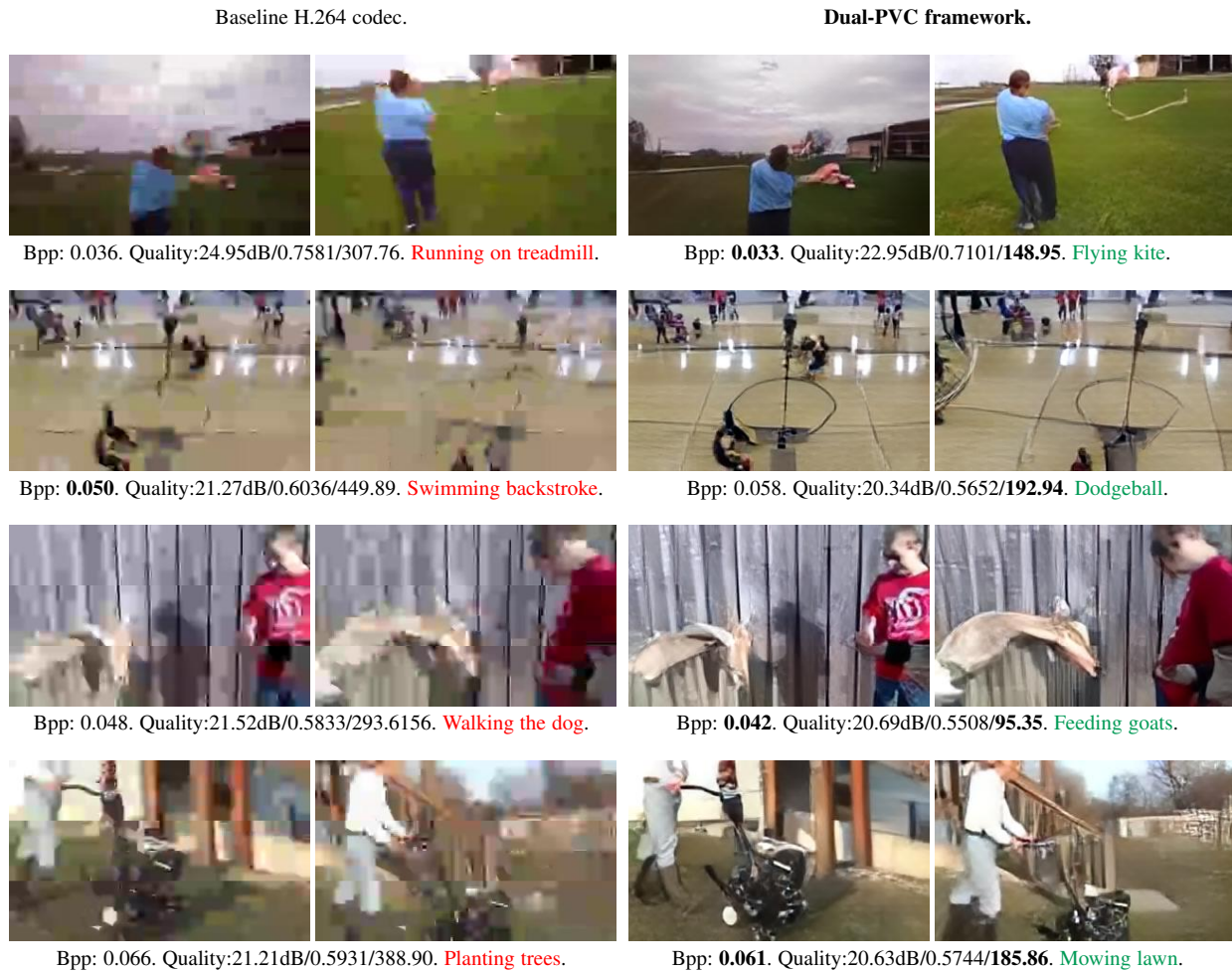
Fig. 7: Restored frames by our Dual-PVC framework. We report the bit cost (in bpp), the quality (in PSNR/SSIM/FID) and the recognition result, respectively. The wrongly recognized action category is in red color, while the correct one is in green color. Higher PSNR/SSIM or lower FID denote better video quality. Lower bpp denotes more bit cost saved. Best to view by zooming-in.
