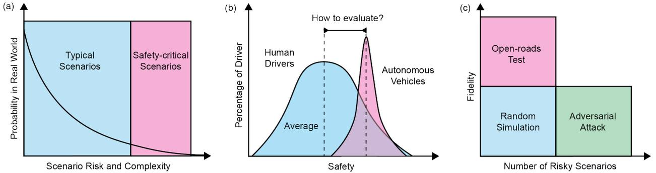
Fig. 1. The overview of autonomous vehicle evaluation. (a) Most of the scenarios that happen in the real world are typical scenarios; safety-critical scenarios are extremely rare. (b) AVs are supposed to have higher average safety than human drivers, but the gap is not easy to be evaluated and measured. (c) Comparison between different generation methods. Most existing methods cannot satisfy the fidelity and safety-critic metrics simultaneously.
