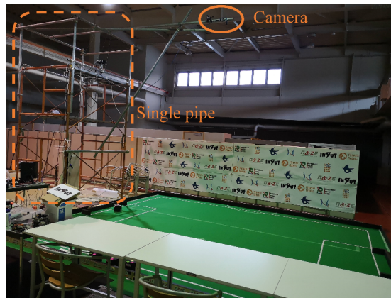
Fig. 16: Camera mounted using single pipe.
