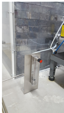
Figure 23: ATEKO-Air Rotameter with valve to measure and regulate air flow rate.
