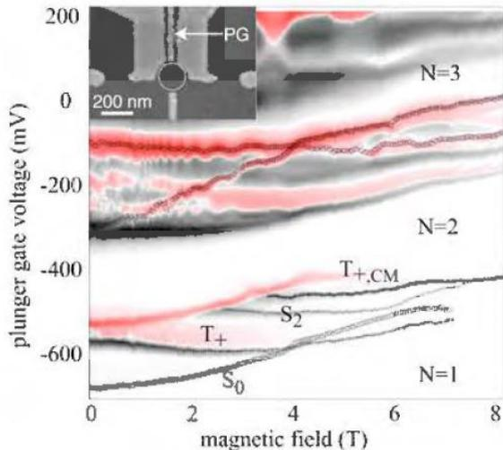
FIG. 1. Measured excited state spectra as a function of magnetic field and plunger gate voltage. Inset: sample geometry.
