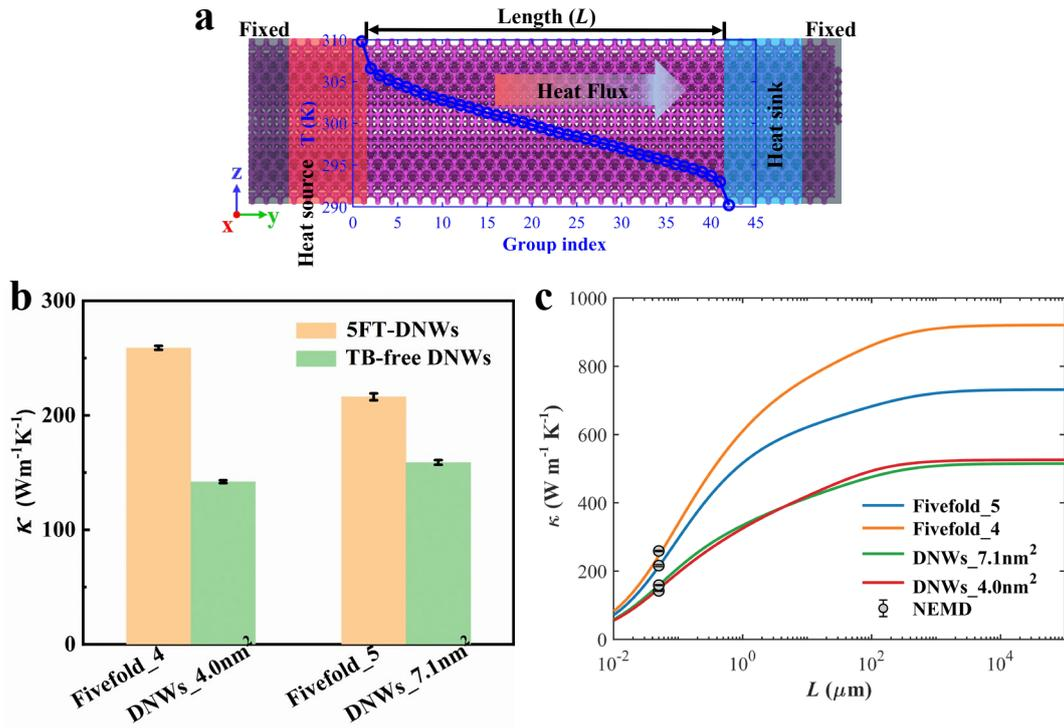
**Figure S4.** (a) Schematic illustration of the setups for the NEMD simulations. The blue inset shows the temperature profile at a steady state. The effective length  $L$  between the heat source and the heat sink is divided into 40 groupings. (b) The thermal conductivity of different DNWs calculated by the NEMD method at 300 K. For each simulation system, we perform four
