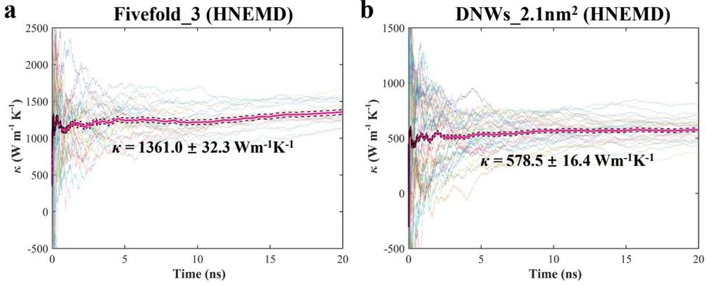
**Figure S2.** Cumulative average of the thermal conductivity as a function of time for different DNWs structures from the HNEMD simulations. In each panel, the thin transparent lines are from multiple independent runs (see Table S1), and the thick magenta solid and black dashed lines represent the average and error bounds from the individual runs.
