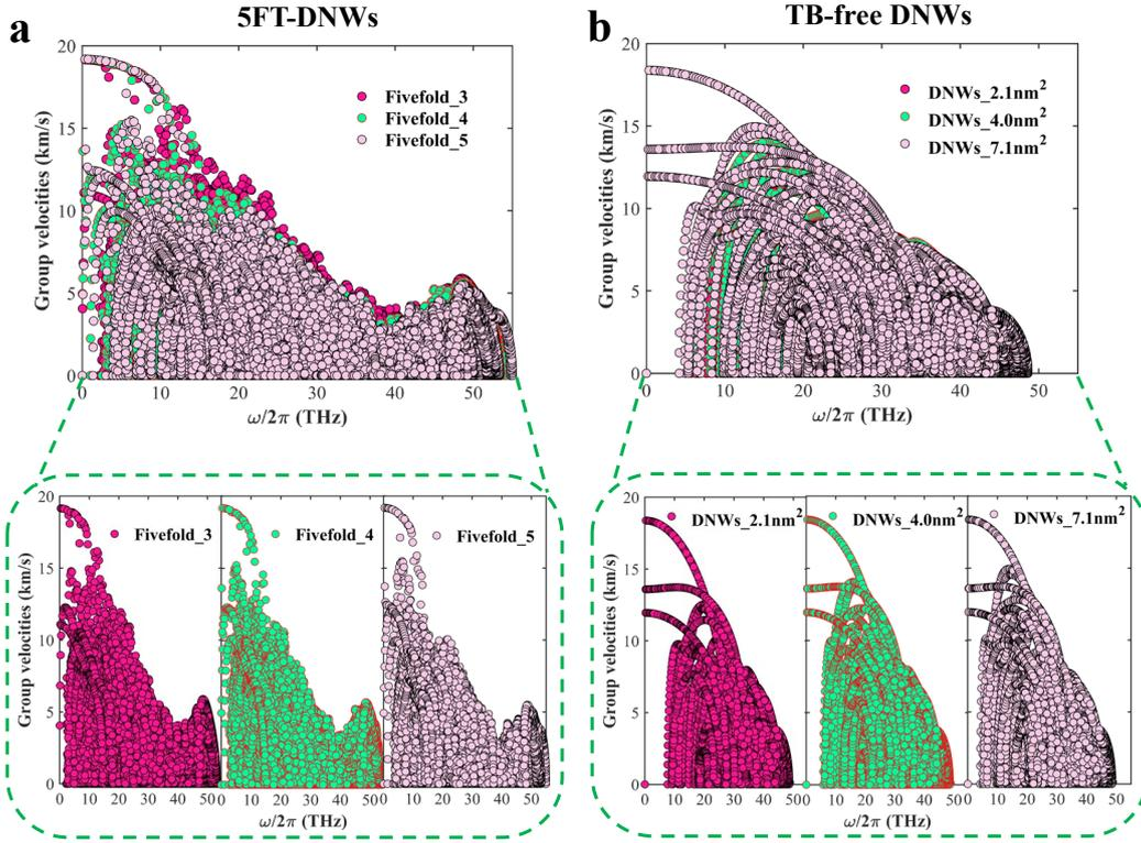
**Figure S8.** Phonon group velocities as a function of phonon frequencies for (a) 5FT-DNWs and (b) TB-free DNWs. Since the group velocities of different  $S$  in TB-free DNWs have slight variation, they are covered by each other at low frequencies ( $< 10$  THz) and high frequencies ( $> 20$  THz), resulting in the eye not being able to distinguish them from the diagram. To better show the physical picture of the phonon group velocities, they are unwrapped in the local images.
