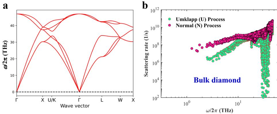
**Figure S9.** (a) The phonon dispersion curve and (b) the three-phonon scattering rates for bulk diamond.
