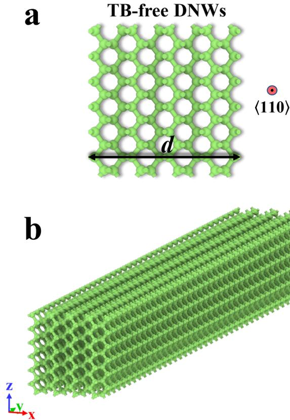
**Figure S1.** The schematic model of TB-free DNWs. (a) Front view for the atomic model of TB-free DNWs constructed along  $[110]$  crystallographic orientation. Since the constructed TB-free DNWs model is approximately square, its cross-sectional area is evaluated as  $d^2$ . (b) Perspective view for the atomic model of TB-free DNWs.
