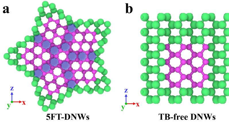
**Figure S5.** A schematic diagram of the surface/core region of different DNWs selected to calculate the phonon MFP spectrum. (a) and (b) are snapshots of the typical structures of 5FT-DNWs and TB-free DNWs, respectively. The smaller diameter purple atoms represent the core region, while the thicker green atoms indicate the surface region.
