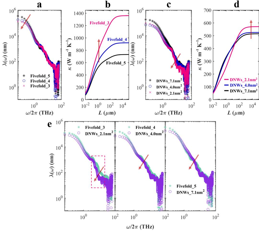
**Figure 2.** The phonon MFP  $\lambda(\omega)$  and the length-dependent thermal conductivity  $\kappa(L)$  for different DNWs. (a-b) for the 5FT-DNWs, while (c-d) for the TB-free DNWs. (e) A comparison of MFP between 5FT-DNWs and TB-free DNWs at the equivalent  $S$ . The arrows in the figure serve as an eye guide, and the magenta dashed boxes indicate that phonon eigenvectors in that frequency interval are used for visualization (see [Figure 3](#)).
