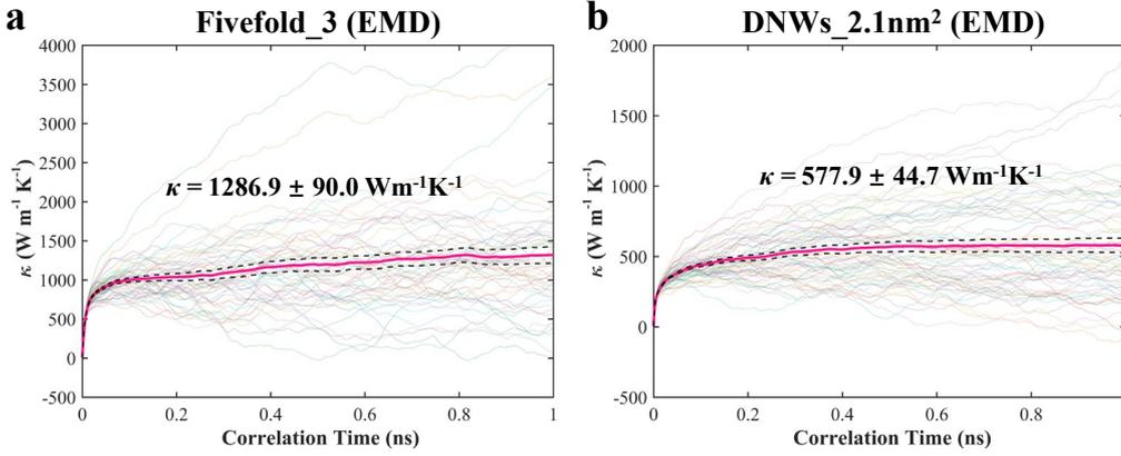
**Figure S3.** Running thermal conductivity  $\kappa(\tau)$  for different DNWs structures at 300 K and zero pressure as a function of correlation time. The meanings of the different line shapes are the same as in [Figure S2](#).
