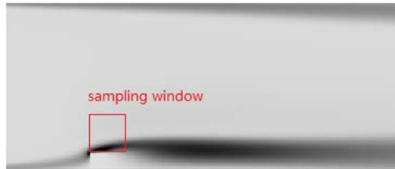
Figure 7 Plot of the target  $k$  field acquired for the standard  $k - \varepsilon$  model, where the red box is the sampling window. Test data were sampled within the window only, independent of import/export boundary conditions.
