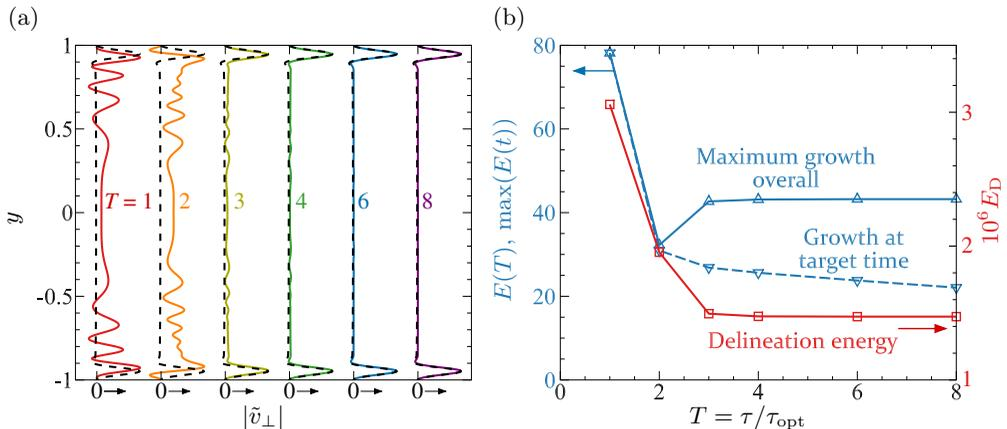
Figure 4: (a) Comparison between linear transient growth initial conditions with various  $\tau = T\tau_{\text{opt}}$  (solid lines) and the leading adjoint mode (dashed lines), horizontally shifted for clarity. (b) Delineation energies from DNS and energy growth ratios from linear analysis for each  $T$ .
