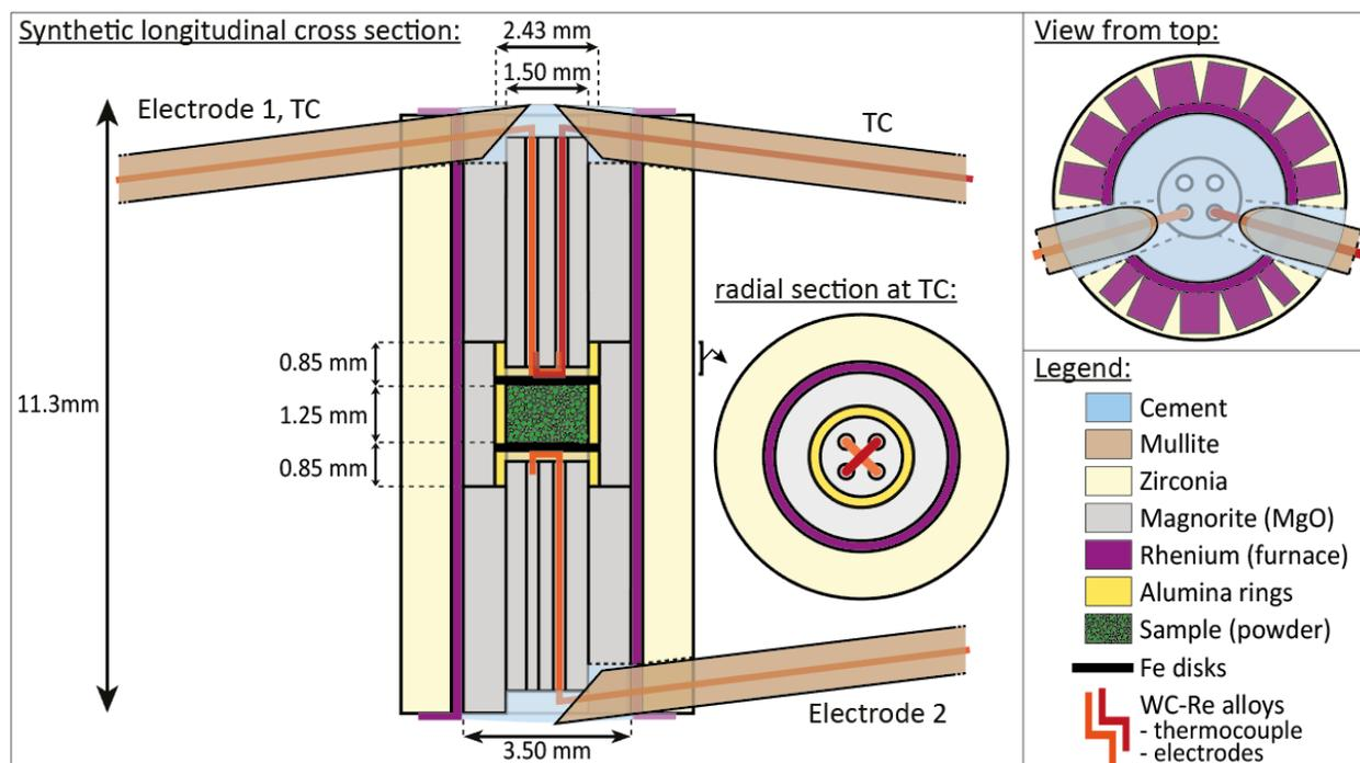
**Figure S2: Experimental assembly.** Synthetic sketch of the 14/8 COMPRES electrical assembly. Experiment BB-238 was performed using a 4-electrodes assembly (4 wires), which consist of a “symmetrical” assembly with 2 thermocouples.
