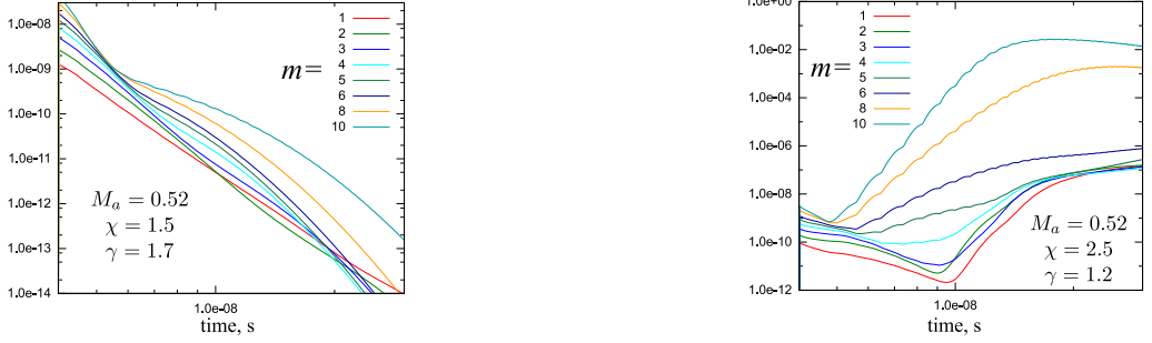
Figure 6: Relative perturbation energies for different azimuthal mode numbers m for one stable and one unstable solution of magnetized Noh.
