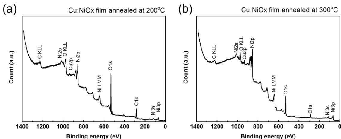
**Figure S1.** XPS survey spectra of the Cu:NiOx films fabricated from precursor containing 0.1 Acac and annealed at (a) 200 °C and (b) 300 °C.
