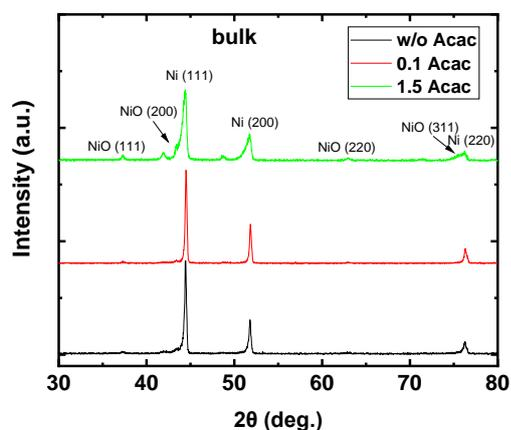
**Figure 5.** XRD patterns of combustion-synthesized samples (bulk) prepared from precursors containing w/o, 0.1 and 1.5 molar ratio of fuel (Acac) to oxidizer (Cu, Ni nitrates) annealed at 200 °C.
