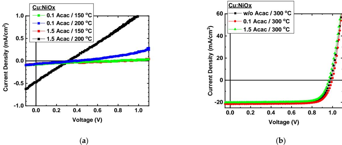
**Figure 10.** J-V curves of ITO/Cu:NiO<sub>x</sub>/perovskite/PC<sub>60</sub>BM/BCP/Ag devices under 1 sun simulated light for Cu:NiO<sub>x</sub> films fabricated from precursor containing (a) 0.1 and 1.5 molar ratio of fuel (Acac) to oxidizer (Cu, Ni nitrates) annealed at 150 and 200 °C, and from precursor containing (b) w/o Acac, 0.1 and 1.5 molar ratio of fuel (Acac) to oxidizer (Cu, Ni nitrates) annealed at 300 °C.
