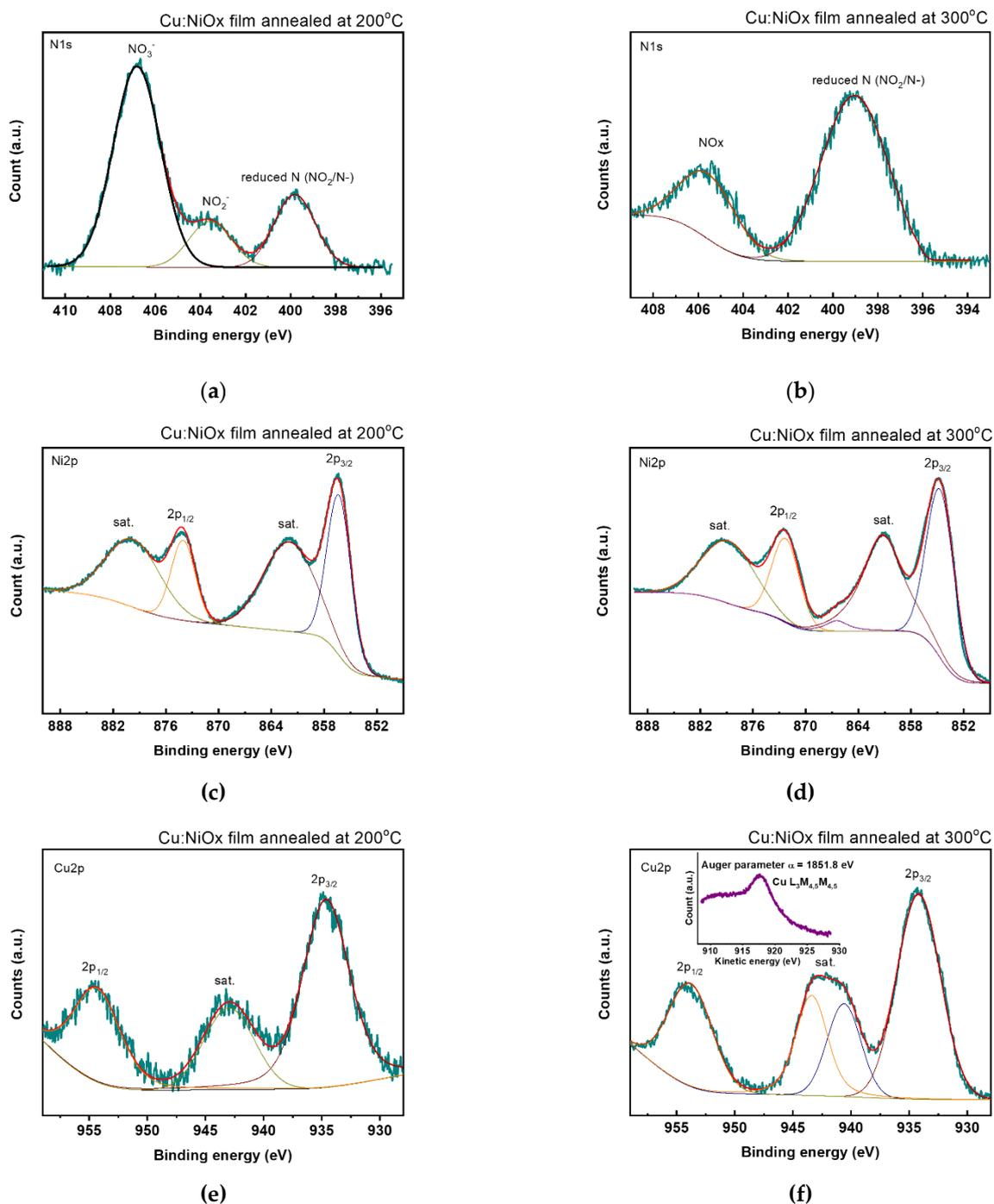
**Figure 6.** XPS spectra of the (a),(b) N 1s, (c),(d) Ni 2p and (e),(f) Cu 2p region of the Cu:NiO<sub>x</sub> films fabricated from precursor containing 0.1 Acac and annealed at 200°C and 300 °C. Inset of panel (f): the Cu L<sub>3</sub>M<sub>4,5</sub>M<sub>4,5</sub> Auger XPS spectrum
