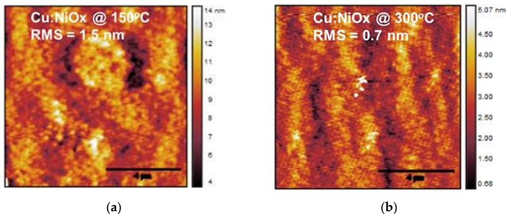
**Figure 7.** AFM images of Cu:NiO<sub>x</sub> films fabricated on quartz substrates from precursor containing 0.1 molar ratio of fuel (Acac) to oxidizer (Cu, Ni nitrates) annealed at (a) 150 and (b) 300 °C.
