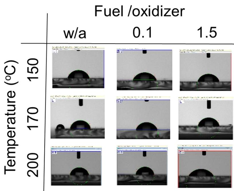
**Figure S2.** contact angle picture of water on films prepared using precursor containing w/o, 0.1 and 1.5 molar ratio of fuel (Acac) to oxidizer (Cu, Ni nitrates) annealed at 150, 170 and 200 °C, respectively.
