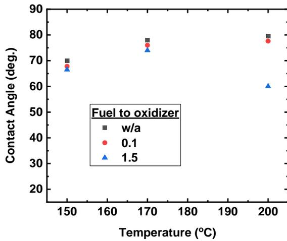
**Figure 9.** A graph presenting the contact angles of water on films prepared using precursor containing w/o Acac, 0.1 and 1.5 molar ratio of fuel (Acac) to oxidizer (Cu, Ni nitrates) annealed at 150, 170 and 200 °C.
