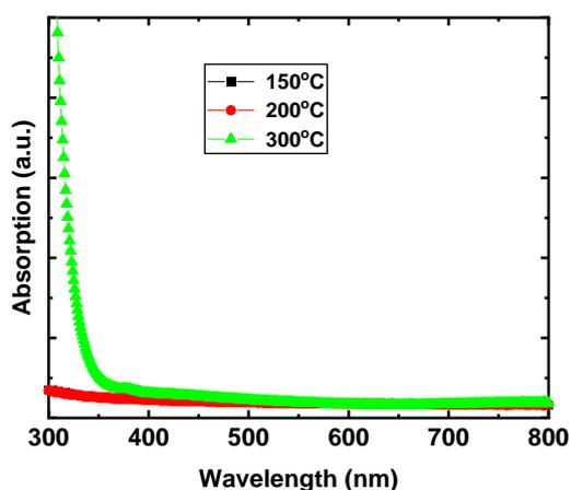
**Figure 8.** UV-Vis absorption of Cu:NiO<sub>x</sub> films fabricated on quartz substrates from precursor containing 0.1 molar ratio of fuel (Acac) to oxidizer (Cu, Ni nitrates) annealed at 150, 200 and 300 °C.
