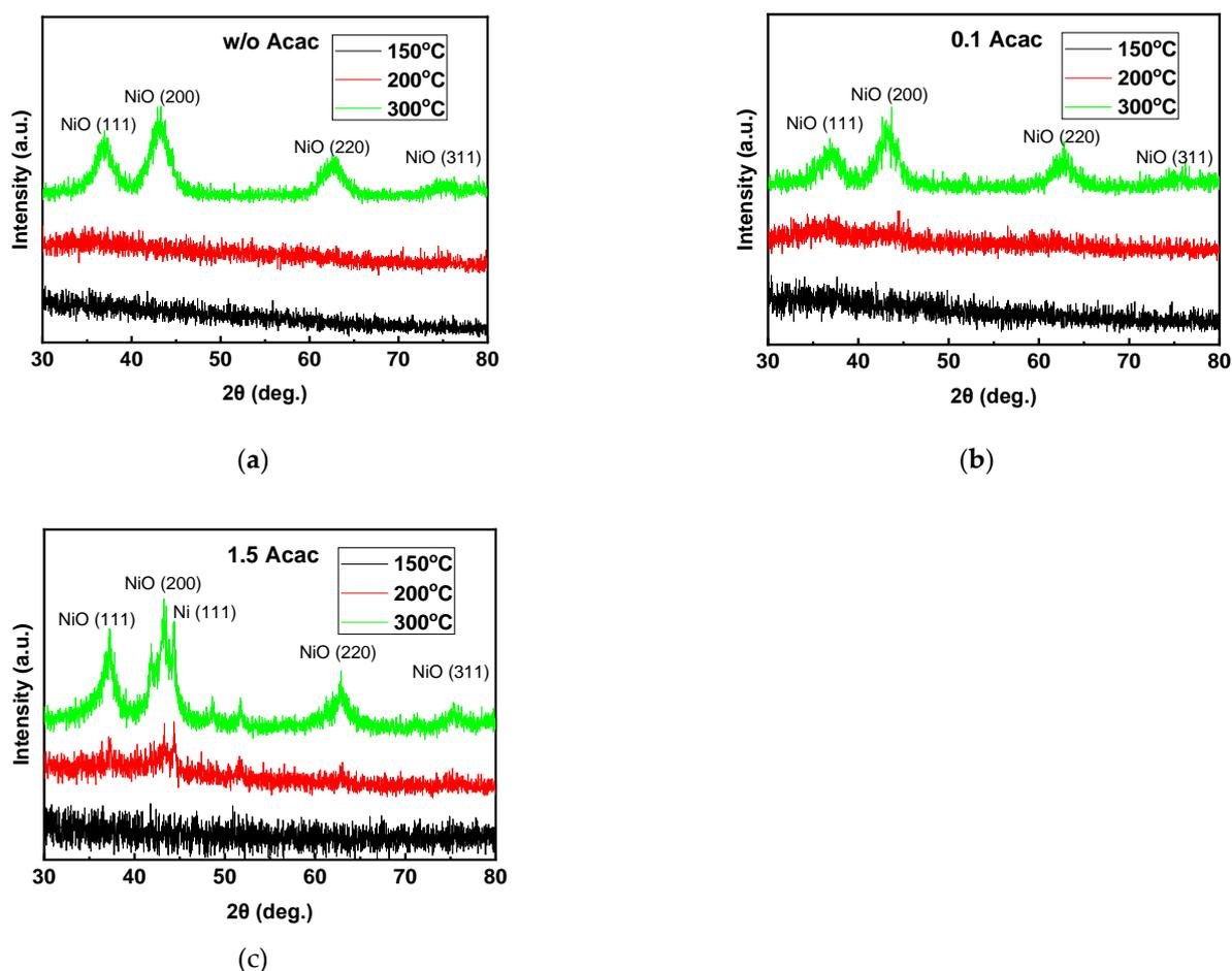
**Figure 4.** XRD patterns of the combustion synthesis of precursor films containing (a) w/o fuel (Acac), (b) 0.1 and (c) 1.5 molar ratio of fuel (Acac) to oxidizer (Cu, Ni nitrates) annealed at 150, 200 and 300 °C .
