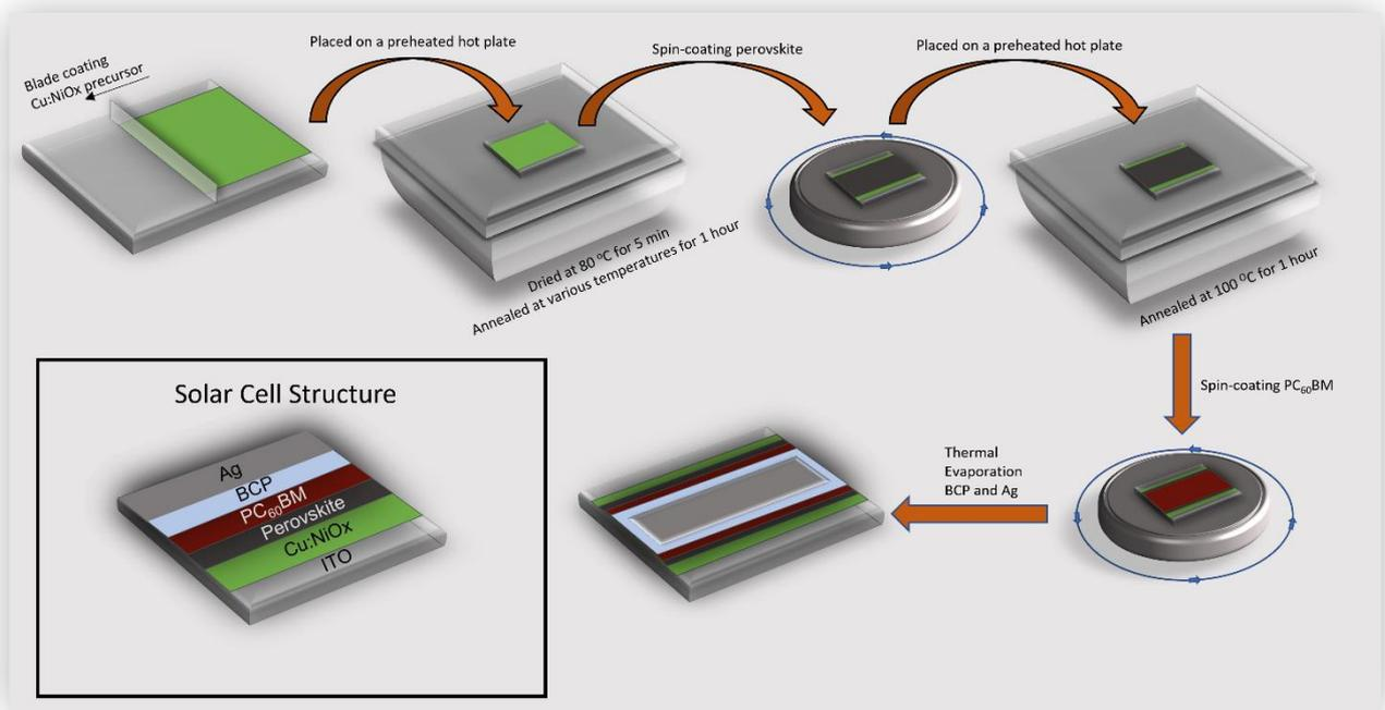
**Figure 1.** Schematic illustration of SCS based Cu:NiO<sub>x</sub> HTL and perovskite device fabrication process and the layer structuring.
