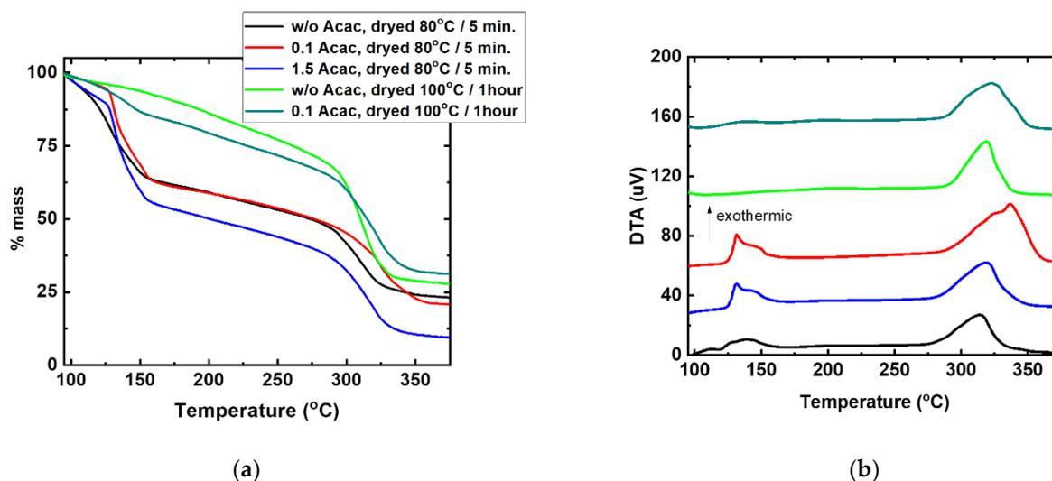
**Figure 2.** (a) TGA curves of precursor films without (w/o) fuel and containing 0.1 and 1.5 molar ratio of fuel (Acac) to oxidizer (Cu, Ni nitrates) in 2-methoxy ethanol dried at 80 and 100 °C, and (b) the respective DTA curves.
