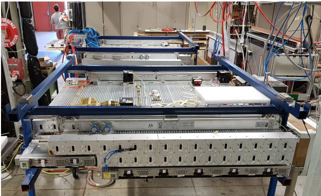
Fig. 5. Final BIS78 muon station with installed B-field and Axial-Praxial, CCC alignment sensors.
