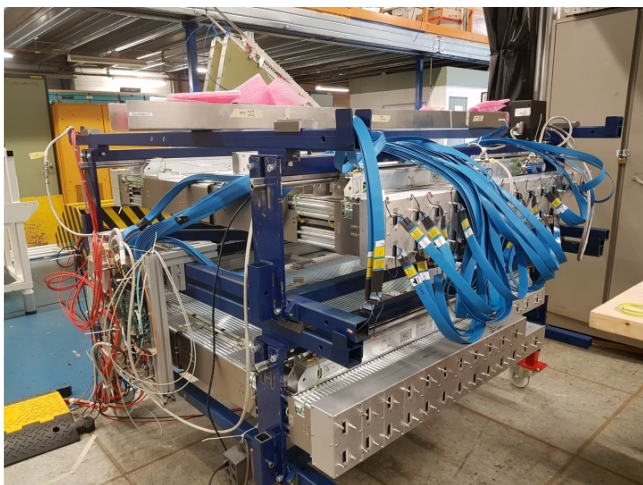
Fig. 2. Picture of the new sMDT chamber during the commissioning campaign at CERN BB5 facility.
