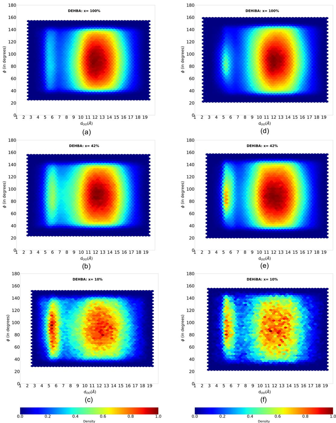
Figure S15: Analysis of the relative orientations of the NCO planes,  $\phi(r_{OO})$ , as a function of the distance between the oxygen of the carbonyl group for DEHBA/dodecane (left column) and DEHiBA/dodecane mixtures (right column). The color bar indicates the normalized count density. 100% DEHBA, (b) 42% DEHBA, (c) 10% DEHBA, (d) 100% DEHiBA, (e) 42% DEHiBA and (f) 10% DEHiBA. The color bar indicates the normalized count density.
