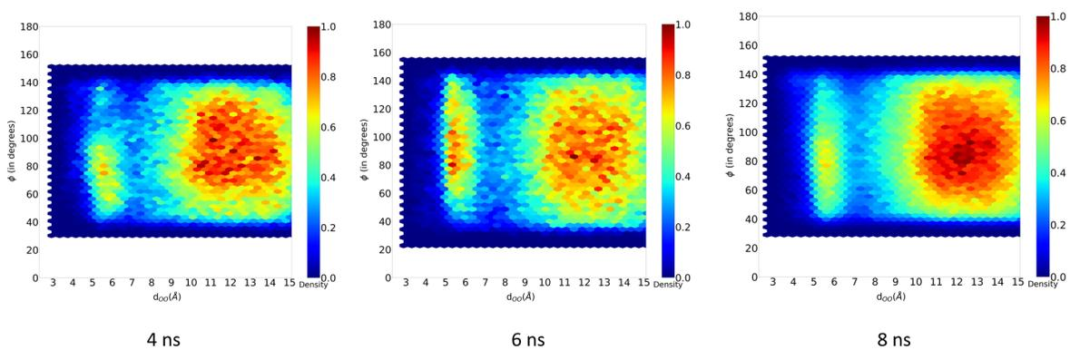
Figure S16: Analysis of the relative orientations of the NCO planes,  $\phi(r_{OO})$ , as a function of the distance between the oxygen of the carbonyl group for 26% DEHBA in dodecane averaged for 4 ns, 6 ns and 8 ns of the equilibration phase. The color bar indicates the normalized count density. The color bar indicates the normalized count density.
