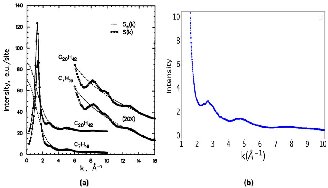
Figure S7: Structure factors for heptane, (a) Experimental data from Habenschuss *et al.*,<sup>S4</sup> (b) simulations using Debye code.<sup>S5</sup>
