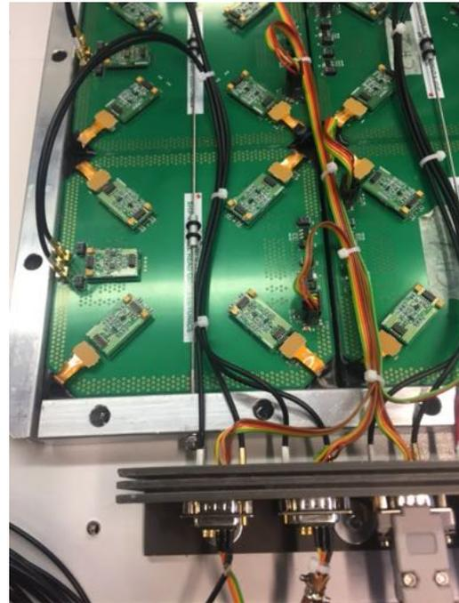
**Fig. 22** Scintillating tile read out of the muon system by four SiPMs at the corner and instrumented with the front-end electronics.
