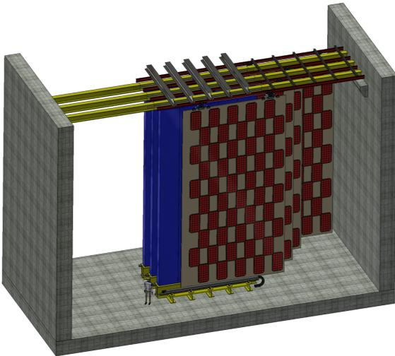
**Fig. 21** Conceptual layout of the HSDS muon system made of four stations. Each station is made of 100 modules, 32 tiles each, organised in a chess structure on both sides of a supporting wall. The stations are interleaved by iron filters.
