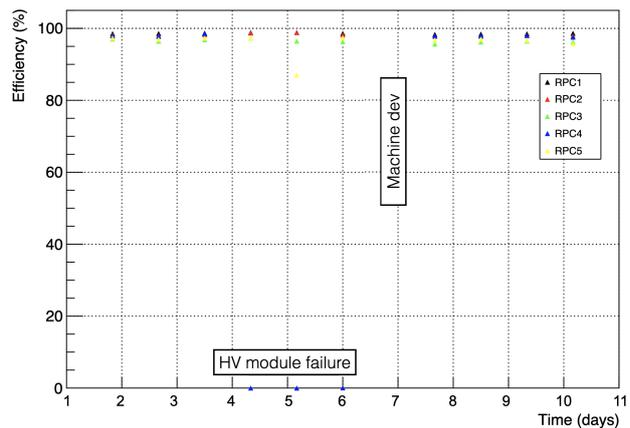
**Fig. 8** Efficiency of the five RPC stations used in the muon-flux and charm-production measurement. During the run, RPC chamber 4 suffered a problem with the high-voltage module during three days and SPS had a day of machine development studies.
