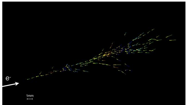
**Fig. 5** Simulated electromagnetic shower induced in an ECC by a 6 GeV/c electron. The picture shows the  $e^+e^-$ -track segments reconstructed in the emulsion films.
