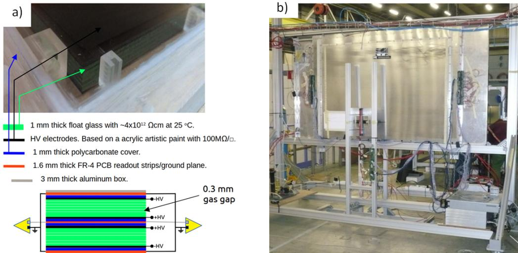
**Fig. 17** a) Detailed photograph of one of the MRPCs together with a sketch of the internal structure of the module. b) Experimental setup at the T9 beam line (CERN East Area), where the MRPC was exposed to negative pions of 8 GeV/c.
