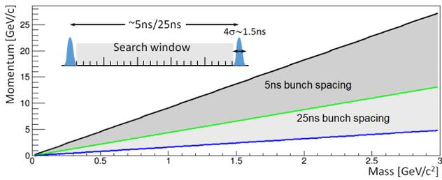
**Fig. 25** Mass-momentum region in which it is possible to discriminate an LDM scattering signature from a neutrino interaction using slow extraction of bunched beam in the SPS and a time-of-flight measurement. The figures assumes a bunch structure with 5 ns respectively 25 ns bunch spacing and 1.5 ns ( $4\sigma$ ) bunch length, and a distance of 40 m between the target and the detector.
