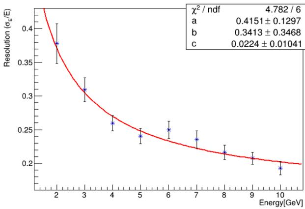
**Fig. 6** Energy resolution for electrons using the ECC as sampling calorimeter, as estimated with MC simulations. The function  $\sigma_E/E = \sqrt{(a/\sqrt{E})^2 + (b/E)^2 + c^2}$  was used for the fit.
