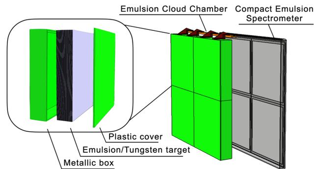
**Fig. 4** Layout of the emulsion target and closeup view of one emulsion brick wall of four cells, each containing an ECC and a CES.
