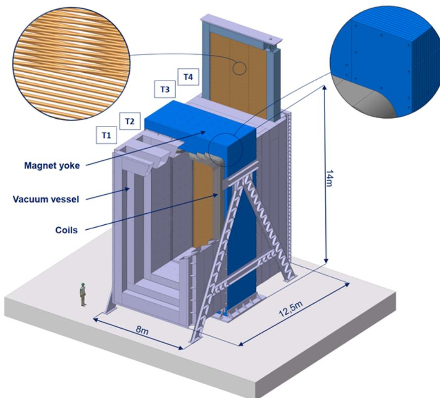
**Fig. 10** Layout of the spectrometer section, with the four top openings in the vacuum vessel for the insertion of the straw tracker stations (T1 – T4), and the surrounding spectrometer magnet. The top-left magnified view illustrates the orientation of the tracker straw tubes, and the top right zooms on the magnet yoke plates with through-holes for assembling with rods.
