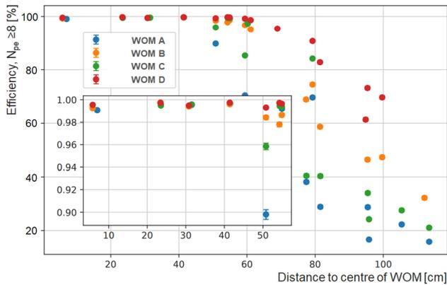
**Fig. 13** Detection efficiency by single SBT WOM for muons as a function of the distance between the muon beam and the WOM. A, B, C, D refer to the four WOMs positioned as indicated in Fig. 12. The insert shows the relevant region magnified.
