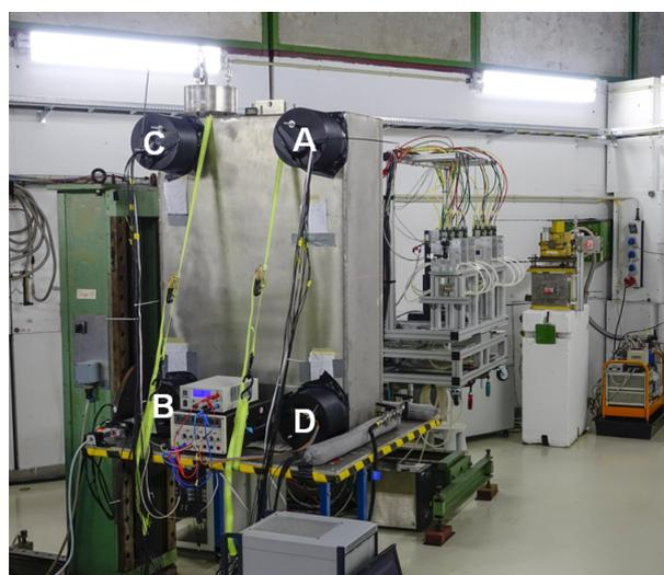
**Fig. 12** Experimental setup of the SBT liquid-scintillator cell prototype, equipped with four WOMs (at positions labelled A, B, C, D) at a DESY electron test beam in 2019.
