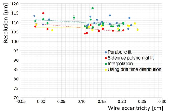
**Fig. 15** Measured spatial resolution for the 20 mm diameter straw tube prototype as a function of the artificially induced wire eccentricity. Four different analysis methods of the spatial resolution are compared (see CERN-THESIS-2020-218). The lines are the results of linear fits.
