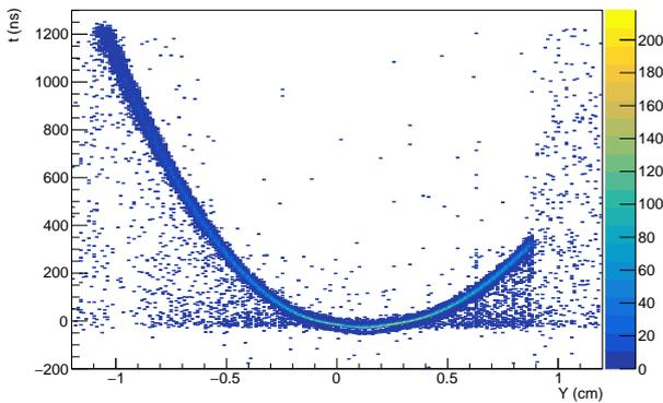
**Fig. 14** Measured drift time versus Y position of the reconstructed particle trajectory with the 20 mm diameter straw-tube prototype with a large wire eccentricity (2.05 mm). The Y axis is vertical, perpendicular to the wire axis X and to the particle beam axis Z.
