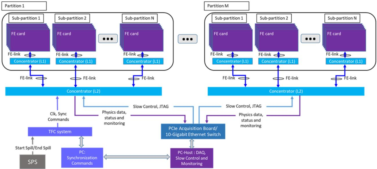
Fig. 23 Global scheme of the SHiP electronics and readout system.
