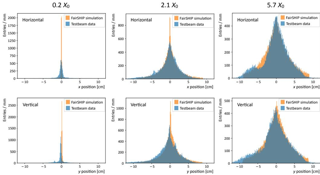
**Fig. 20** Measured and simulated transverse electromagnetic-shower distribution with 5 GeV electrons from the CERN PS at different calorimeter depths.
