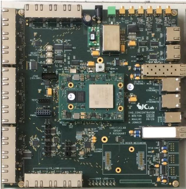
Fig. 24 Prototype of the SHiP FE concentrator board.
