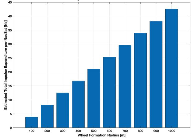
**Figure 3.** The simulated fuel expenditure of initial formation is shown for varying wheel radius. The transfer time limit of 15 min (roughly 1/6 of orbital period) was imposed throughout the simulation with spacecraft mass of 10 kg assumed. The estimated fuel cost linearly increases as the desired wheel radius enlarges.
