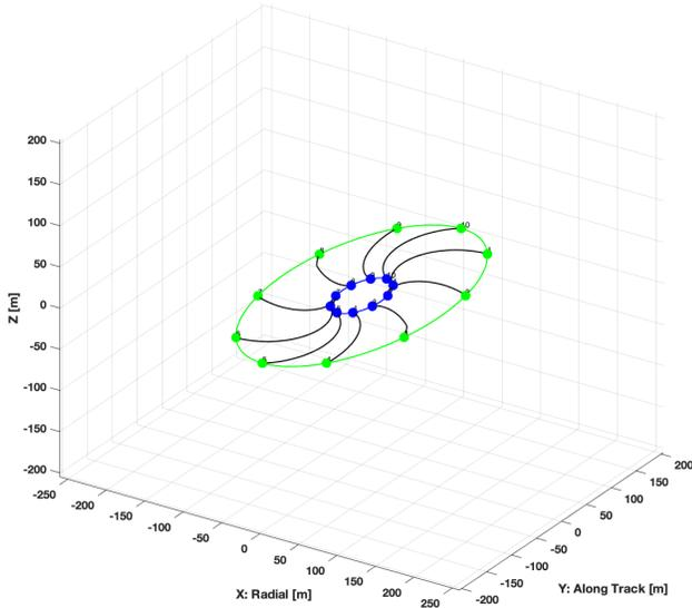
**Figure 2.** Each fleet in the GEOSCAN constellation will go through initialization to a wheel formation after deployment. On-board optimization-based algorithm will autonomously compute minimum fuel trajectories for this maneuver without ground-in-the-loop intervention.
