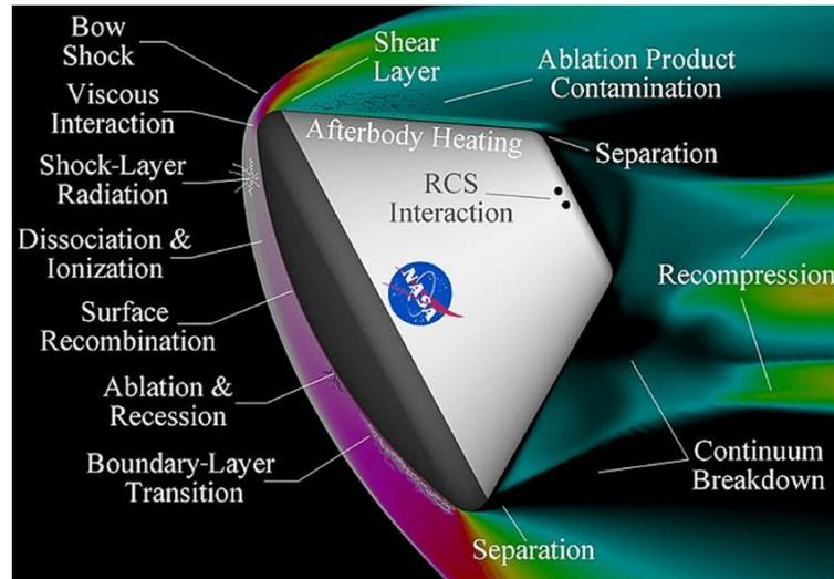
**Fig. 1 Schematic view of a typical planetary re-entry phenomena**
