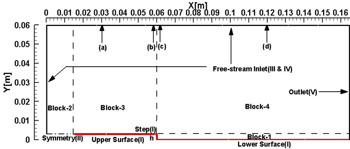
Fig. 2 Schematic of the 2D BFS.
