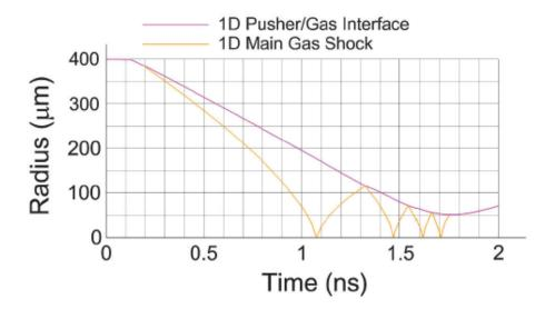
Fig. 2 R-T plot from 1D RAGE simulation of the simplified ICF. Reproduced with permission from Thomas et.al. Phys. Rev. Lett. **109**, 075004 (2012). Copyright 2012 American Physical Society (Fig. 1a in Ref. [5]). RNP/22/Jan/049531
