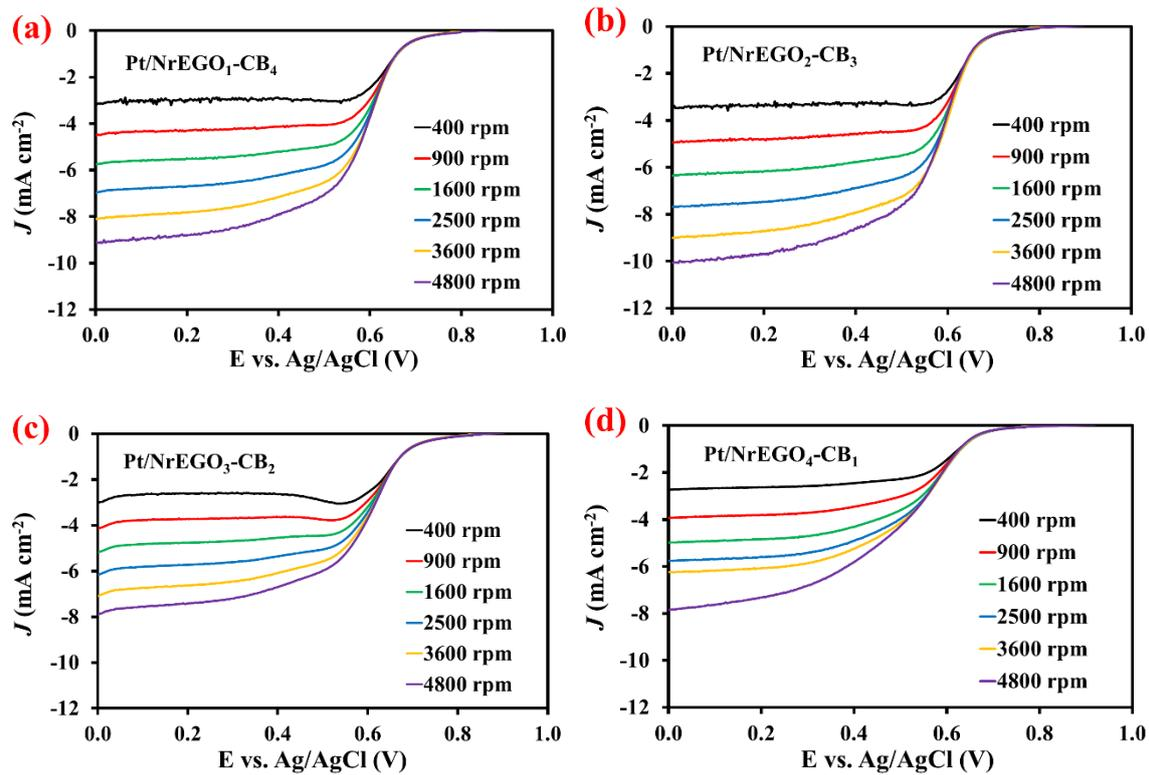
**Fig. S6** Linear sweep voltammetry of all nitrogen doped catalysts at different rotation speed for the evaluation of ORR activity.
