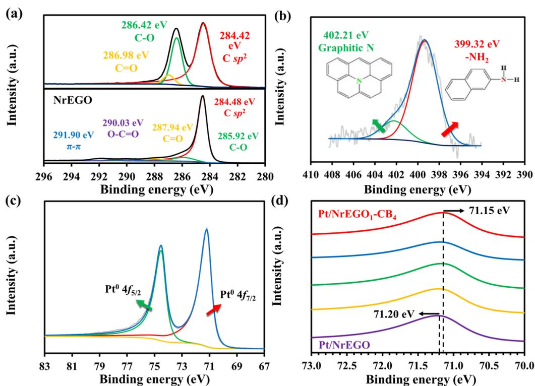
**Fig 3.** High-resolution XPS spectra of (a) C 1s and (b) N 1s in NrEGO, (c) N 1s and (d) Pt 4f in Pt/NrEGO<sub>2</sub>-CB<sub>3</sub>.
