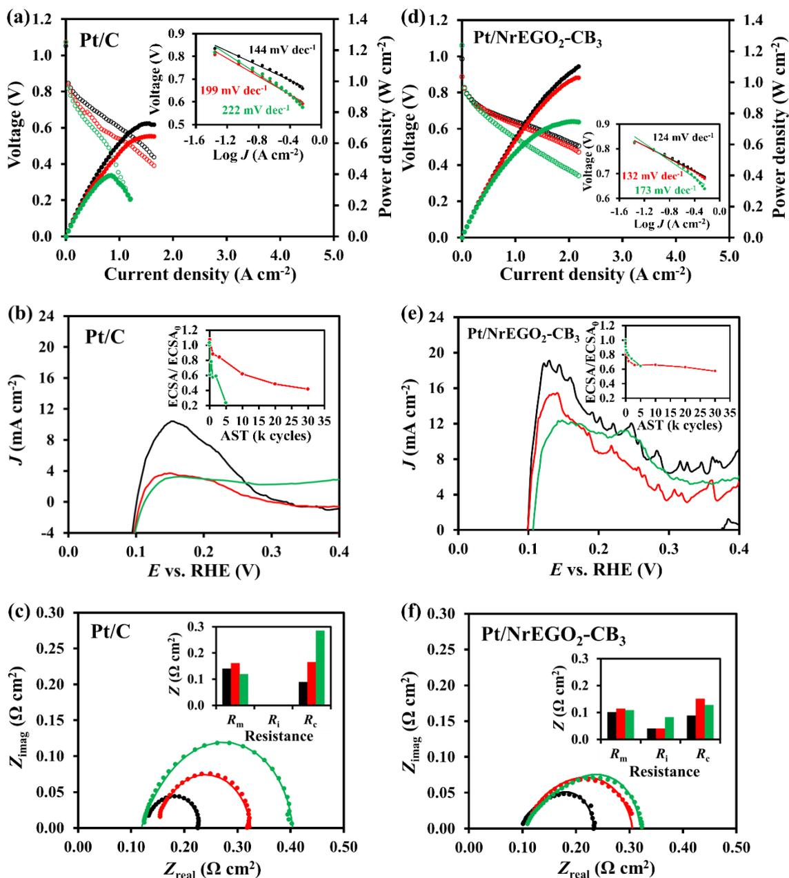
**Fig 8.** Electrochemical performance of catalysts before and after catalyst degradation and carbon corrosion ASTs. The measurements of Pt/C in (a) polarization curves with Tafel slopes, (b) ECSA and (c) EIS before and after ASTs. The measurement of Pt/NrEGO<sub>2</sub>-CB<sub>3</sub> in (d) polarization curves with Tafel slopes, (e) ECSA and (f) EIS before and after ASTs. • fresh catalysts. • after 30k cycles catalysts degradation ASTs. • after 5k cycles support corrosion ASTs.
