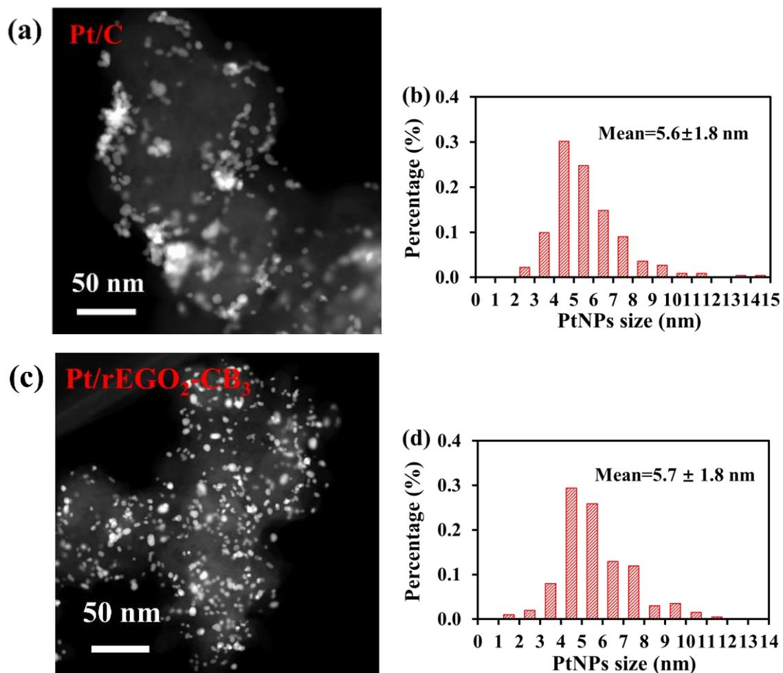
**Fig. S4** Typical HAADF STEM images of (a) Pt/C and (c) Pt/rEGO<sub>2</sub>-CB<sub>3</sub>. Statistical analysis of PtNPs size distribution of (b) Pt/C by counting 222 particles and (d) Pt/rEGO<sub>2</sub>-CB<sub>3</sub> by counting 201 particles.
