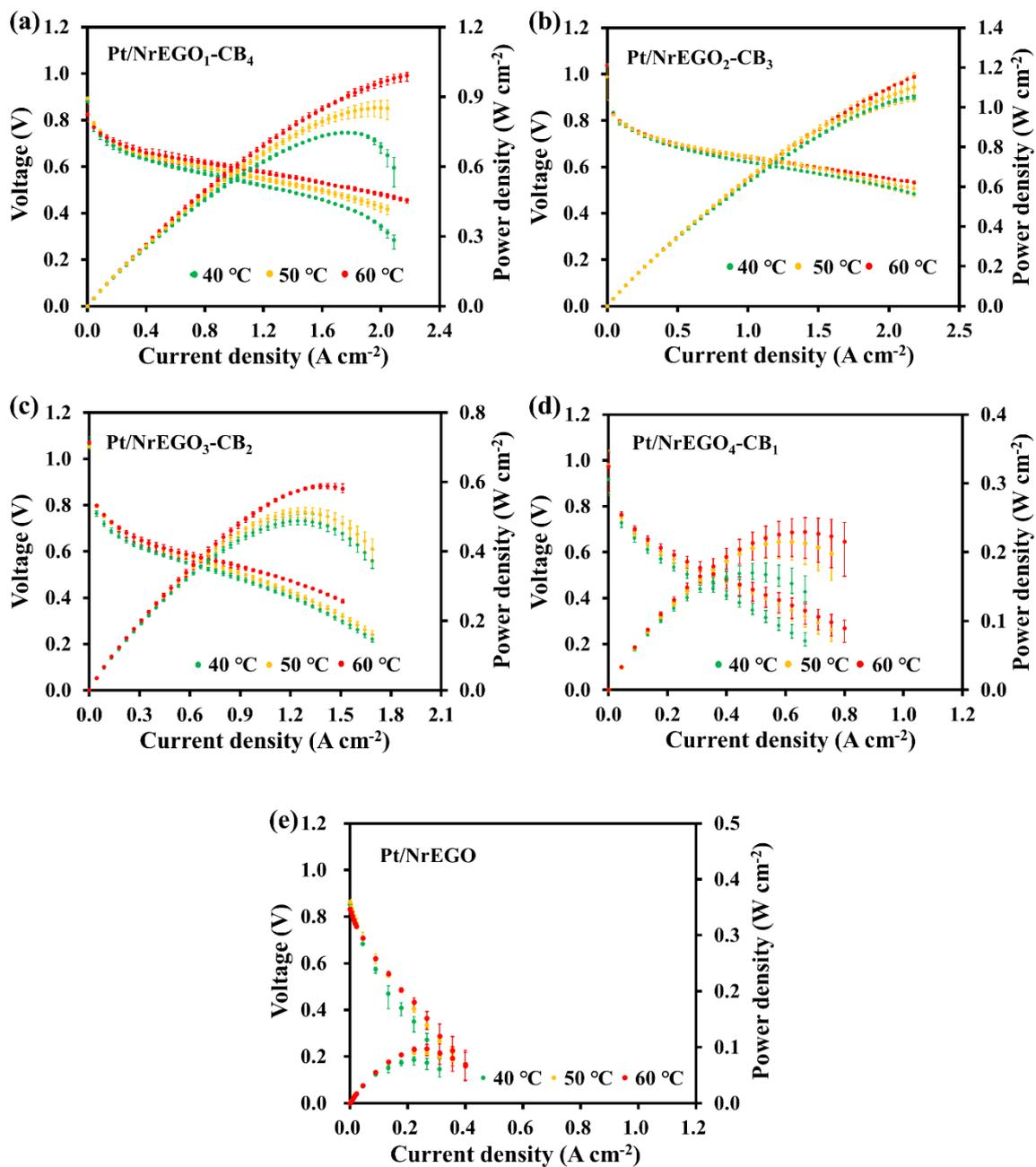
Fig. S7 All nitrogen doped catalyst performance at 40 °C, 50 °C and 60 °C.
