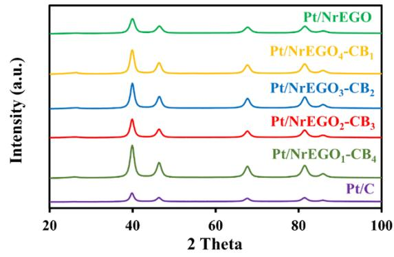
**Fig. S5** The XRD spectra comparing Pt/C with different ratios of hybrid catalyst support Pt/NrEGO<sub>x</sub>-CB<sub>y</sub> and Pt/NrEGO.
