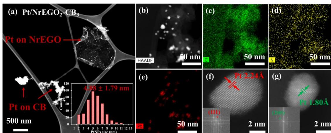
**Fig 5.** Typical HAADF STEM images of (a) Pt/NrEGO<sub>2</sub>-CB<sub>3</sub> and the statistics on Pt particle size distribution by counting 421 particles. (b-e) HAADF STEM images of Pt/NrEGO<sub>2</sub>-CB<sub>3</sub> and its corresponding EDS elemental maps of C, N, and Pt. (f and g) High resolution HAADF images of Pt/NrEGO<sub>2</sub>-CB<sub>3</sub> showing lattice fringes of selected specific Pt particles with corresponding FFT patterns.
