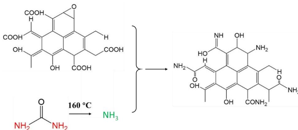
**Scheme 1.** A reaction route from the electrochemically exfoliated graphene oxide (EGO) to the nitrogen-doped reduced EGO (NrEGO).
