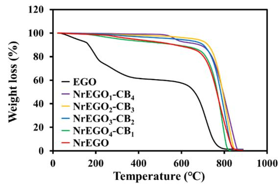
**Fig. S2** TGA analysis for the thermal stability of all N-doped catalysts support.
