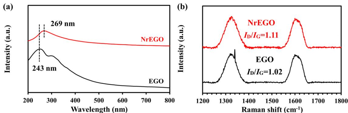
**Fig 2.** Characterization of EGO and NrEGO by (a) the whole wavelength analysis of UV-vis and (b) Raman spectra under 785 nm.
