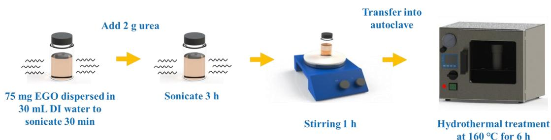
**Fig 1.** Synthesis routes of nitrogen-doped reduced electrochemically exfoliated graphene oxide (NrEGO).
