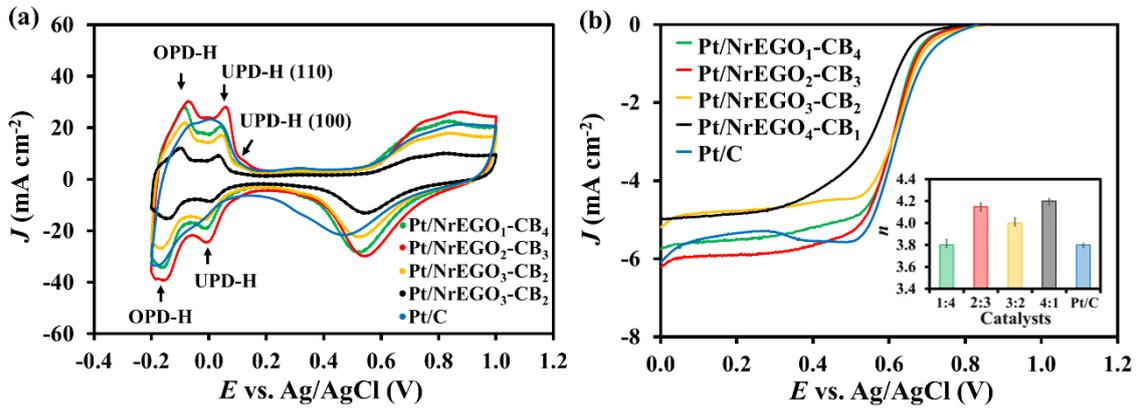
**Fig 6.** Electrochemical characterization of all catalysts: (a) ECSAs measured by cyclic voltammetry and (b) ORR activity and electron transfer number (inset) as measured by linear sweep voltammetry on all electrocatalysts.
