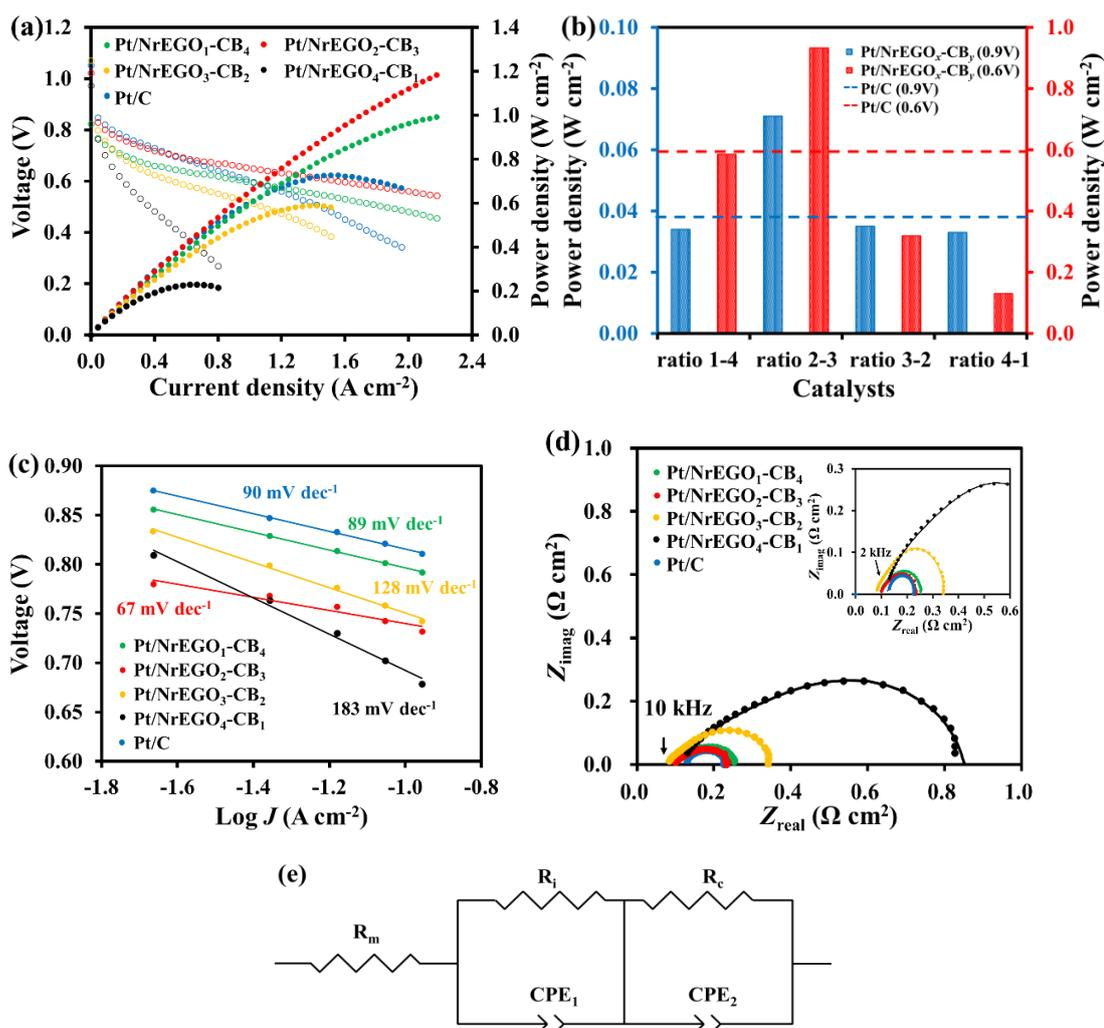
**Fig 7.** (a) Polarization curves of different ratio of N-doped hybrid support catalysts in MEAs and (b) comparison power density with same ratio of no N doped hybrid support catalysts (Pt/rEGO<sub>x</sub>-CB<sub>y</sub>) at 0.60 V. (c) Tafel slopes of Pt/NrEGO<sub>x</sub>-CB<sub>y</sub> and Pt/C, respectively. (d) EIS of all catalysts and (e) the equivalent circuit diagram of a single cell.
