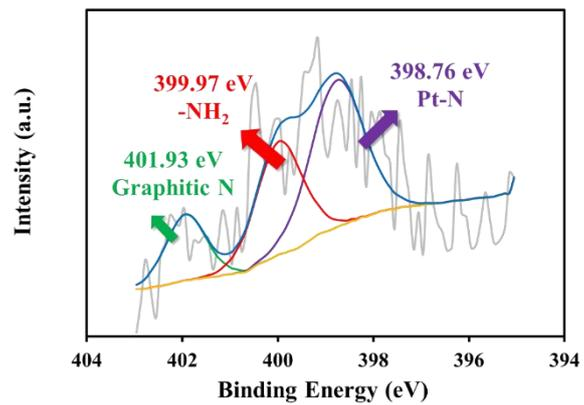
**Fig. S3** High-resolution XPS spectra of N 1s in Pt/NrEGO<sub>2</sub>-CB<sub>3</sub>.
