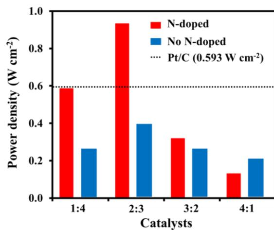
**Fig. S8** The comparison of Pt/NrEGO<sub>x</sub>-CB<sub>y</sub> and Pt/rEGO<sub>x</sub>-CB<sub>y</sub> performance at 0.60 V.
