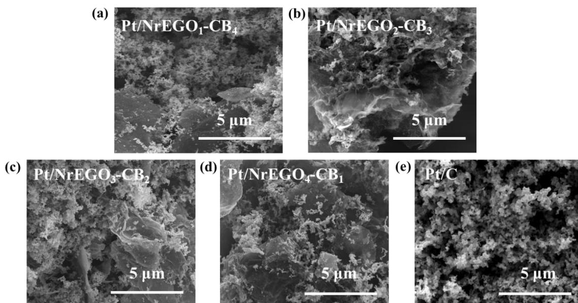
**Fig 4.** SEM images for the catalyst structure of (a) Pt/NrEGO<sub>1</sub>-CB<sub>4</sub>, (b) Pt/NrEGO<sub>2</sub>-CB<sub>3</sub>, (c) Pt/NrEGO<sub>3</sub>-CB<sub>2</sub>, (d) Pt/NrEGO<sub>4</sub>-CB<sub>1</sub> and (e) commercial Pt/C.
