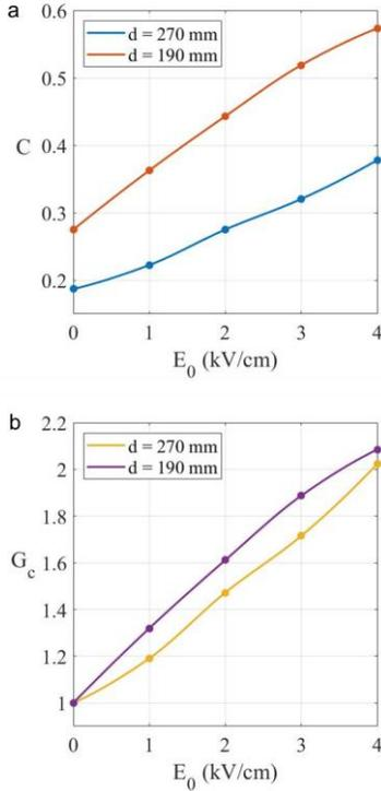
Fig. 4. (a) Cross-correlation coefficient and (b) cross-correlation gain vs applied electric field corresponding to the images in Figs. 3(b–f) and (g–k).
