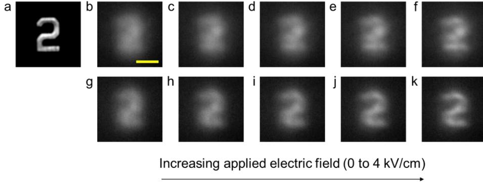
Fig. 3. Experimental results for reconstructed ‘2’ images. Optical intensity,  $I_0 = 6.1 \text{ W/cm}^2$ . (a) Original image. Scattered images at the output face with (b)  $d = 270 \text{ mm}$  and (g)  $d = 190 \text{ mm}$ . (c–f) and (h–k) are reconstructed from (b) and (g) respectively with applied electric fields of (c, h) 1 kV/cm, (d, i) 2 kV/cm, (e, j) 3 kV/cm, and (f, k) 4 kV/cm. Scale bar,  $150 \mu\text{m}$ .
