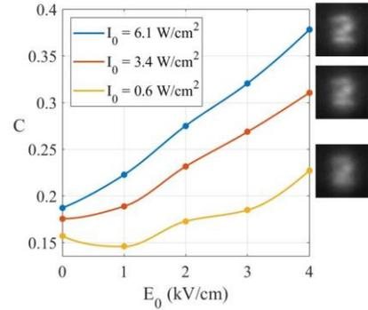
Fig. 5. Cross-correlation coefficient vs applied electric field for different values of the incident intensity. Other experimental conditions for  $I_0 = 3.4 \text{ W/cm}^2$  and  $0.6 \text{ W/cm}^2$  remain the same as  $I_0 = 6.1 \text{ W/cm}^2$ .
