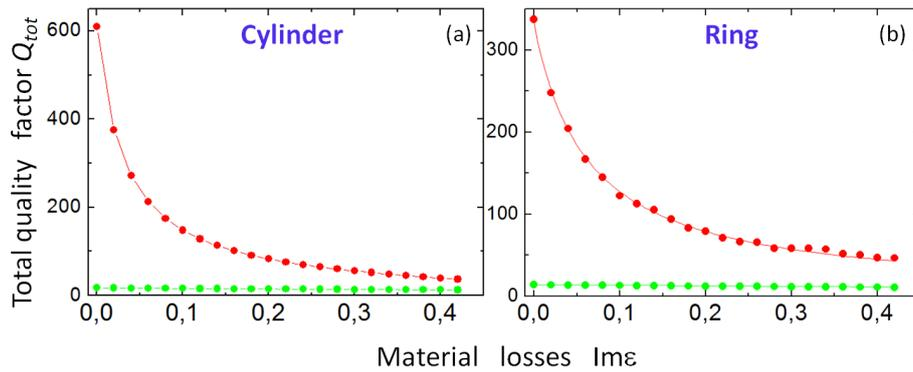
**Figure 5.** Dependences of the total quality factor  $Q_{tot}$  of the high-frequency branch (red) and low-frequency branch (green) on the material losses for the cylinder (a) and ring (b).
