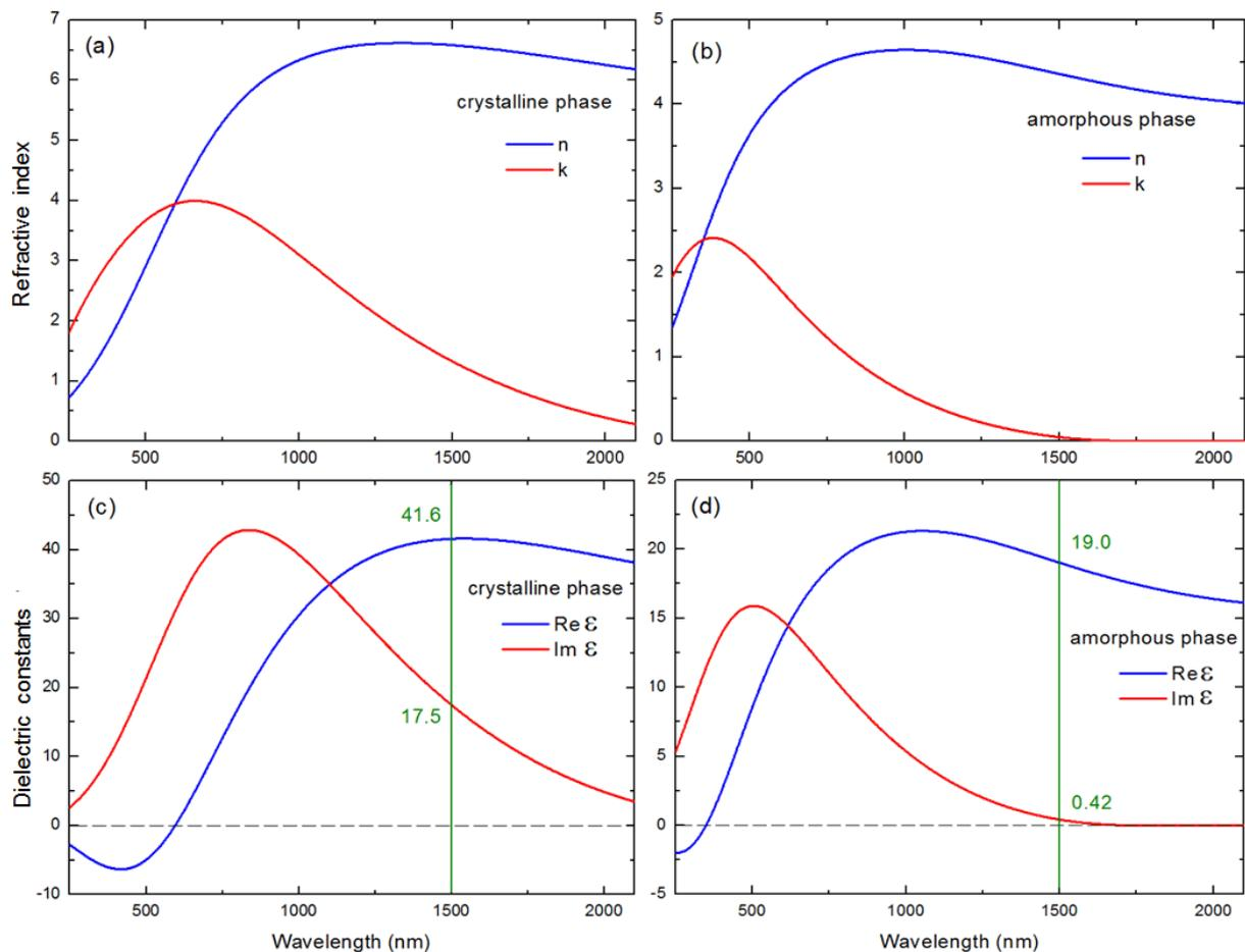
**Figure 1.** Experimentally measured complex refractive index  $N = n + ik$ ,  $n$  – refractive index,  $k$  – extinction coefficient) of the GST film in crystalline (a) and amorphous (b) phases. Calculated complex permittivity  $\varepsilon = \varepsilon' + i\varepsilon''$  of the GST film in crystalline (c) and amorphous (d) phases.
