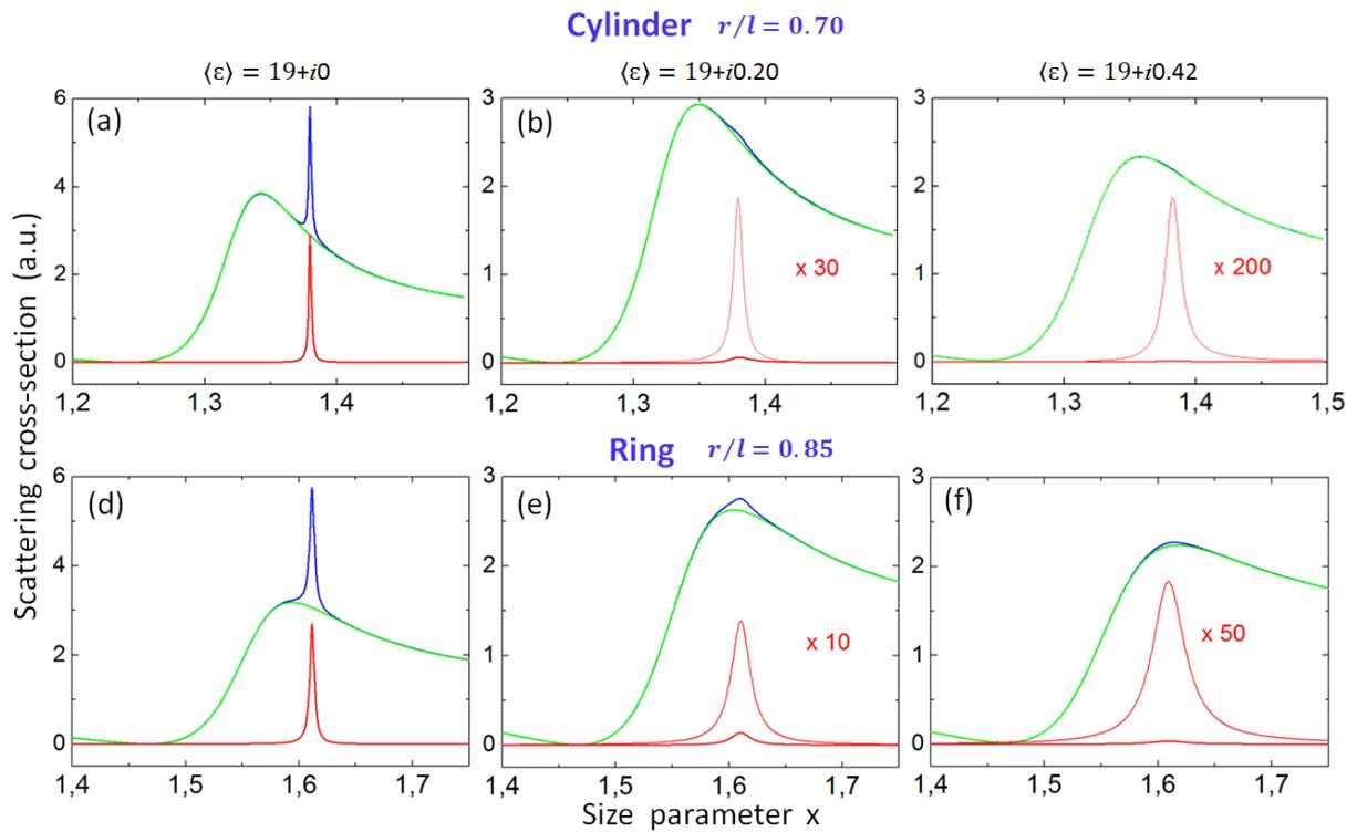
**Figure 3.** SCS spectra of the cylinder and ring for the aspect ratios  $r/l$  corresponding to quasi-BIC (blue line) (Figure 2), and their decomposition into two contours corresponding to the low-frequency (green line) and high-frequency (red line) branches. Normalized size parameter  $x = r\omega/c$ . TE-polarized incident wave.
