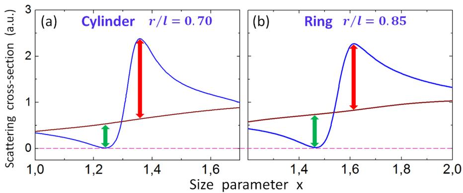
**Figure 7.** SCS spectra of the cylinder (a) and ring (b) in the amorphous (blue line) and crystalline (brown line) GST phases in the avoided crossing spectral region of the  $TE_{0,2,0}$  and  $TE_{0,1,2}$  modes. The lilac dotted line indicates zero scattering intensity. Normalized size parameter  $x = r\omega/c$ . TE-polarized incident wave.
