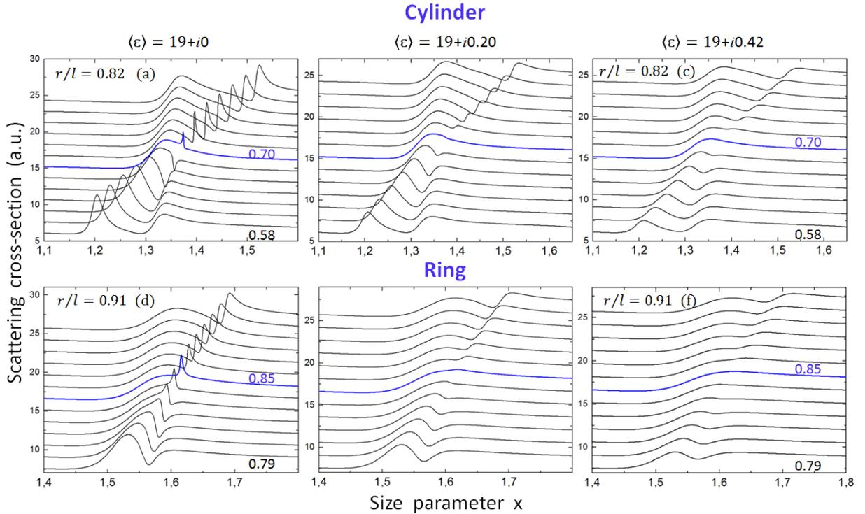
**Figure 2.** Spectra of the normalized SCS (for harmonic  $m=0$ ) for cylindrical (a-c) and ring (d-f) of GST in amorphous phase as a function of their aspect ratio  $r/l$  in the regions of avoided crossing regime between the Mie-type  $\text{TE}_{0,2,0}$  and Fabry-Perot-type  $\text{TE}_{0,1,2}$  modes. The spectra
