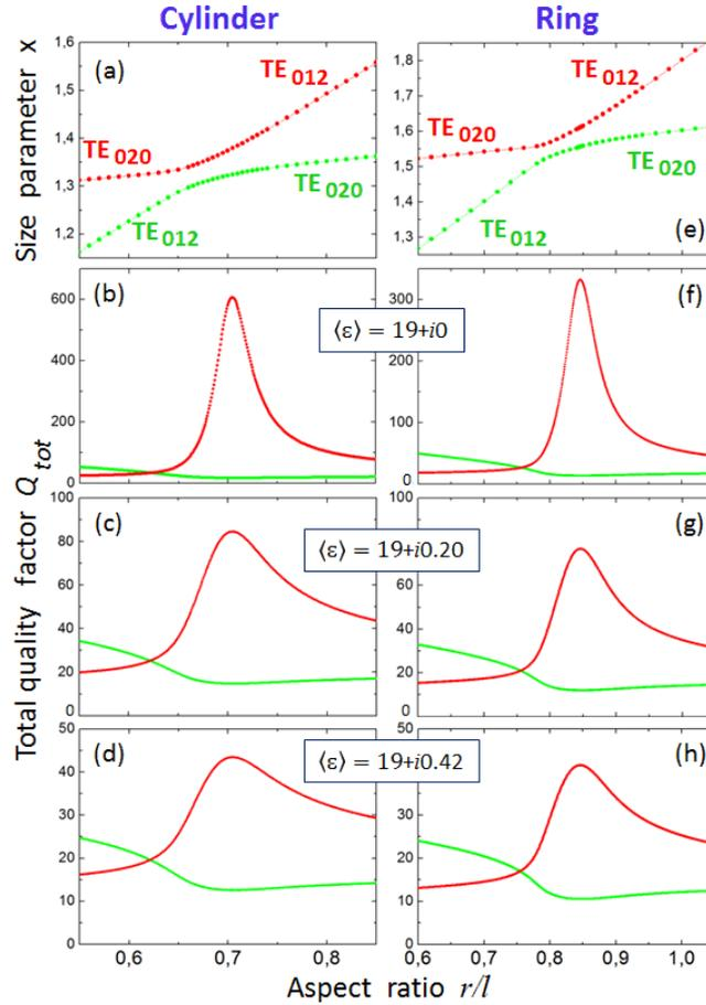
**Figure 4.** a, e) Calculated frequencies of the  $TE_{0,1,2}$  and  $TE_{0,2,0}$  modes in the avoided crossing regions for the cylinder and the ring as a function of its aspect ratio. Dependences of the total quality factor  $Q_{tot}$  of the high-frequency branch (red) and low-frequency branch (green) on the aspect ratio for the cylinder (b-d) and ring (f-h) for three values of the dielectric permittivity. TE-polarized incident wave, normalized size parameter  $x = r\omega/c$ .
