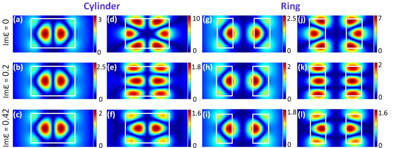
**Figure 6.** Distribution of the electric field amplitude  $|E|$  in the  $(x, z)$  cross-sections (resonator side view) for the cylinder (a-f) and ring (g-l) for the low-frequency (a-c and g-i) and high-
