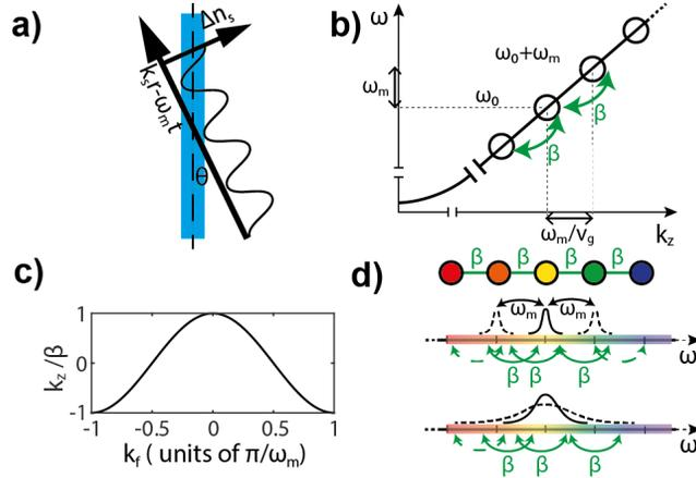
Fig. 1. a) concept of the travelling sound wave used to modulate a single optical waveguide. b) Induced 1D spectral lattice in the dispersion relation of the fundamental waveguide mode. c) Dispersion relation in the frequency lattice, that is the longitudinal wavevector  $k_z$  plotted as a function of the frequency momentum  $k_f$ . d) top(bottom) Illustration of the qualitatively different dynamics for narrowband(broadband) light beam compared to the modulation frequency  $\omega_m$
