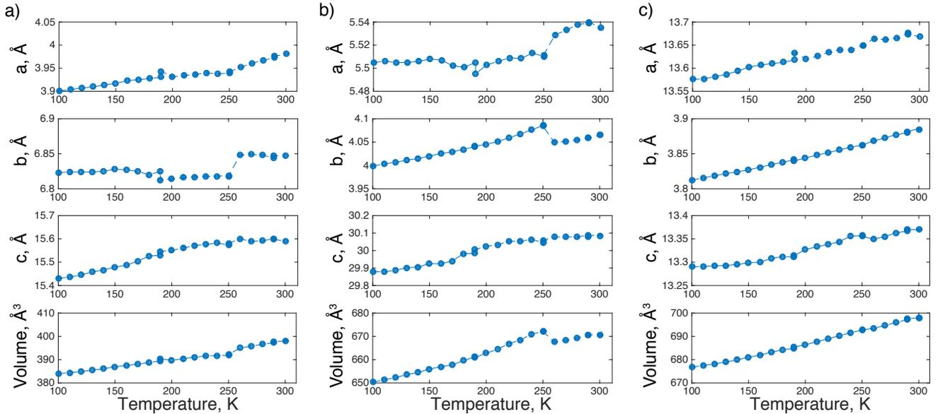
Figure S3: Unit-cell parameters change with temperature respectively for  $\alpha$ - (a),  $\beta$ - (b) and  $\gamma$ - (c) phase in a multi-phase QNC sample.
