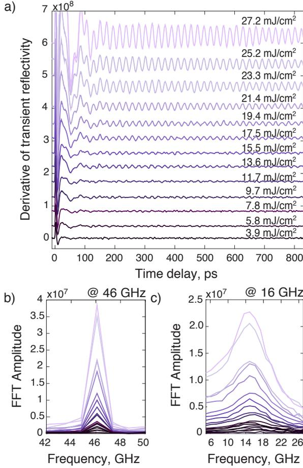
Figure 2: (Color online) (a) Time derivative of the recorded transient reflectivity signals obtained at different pump fluences. (b) Fourier amplitudes of the 46 GHz Brillouin oscillations in glass. (c) Fourier amplitudes of the 16 GHz acoustic resonance.
