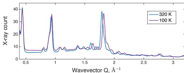
Figure S4: Powder x-ray diffraction patterns of a multi-phase QNC sample taken at 320 K and 100 K respectively. The shift in wavevector  $Q$  ( $\text{\AA}^{-1}$ ) indicates the system response to temperature.
