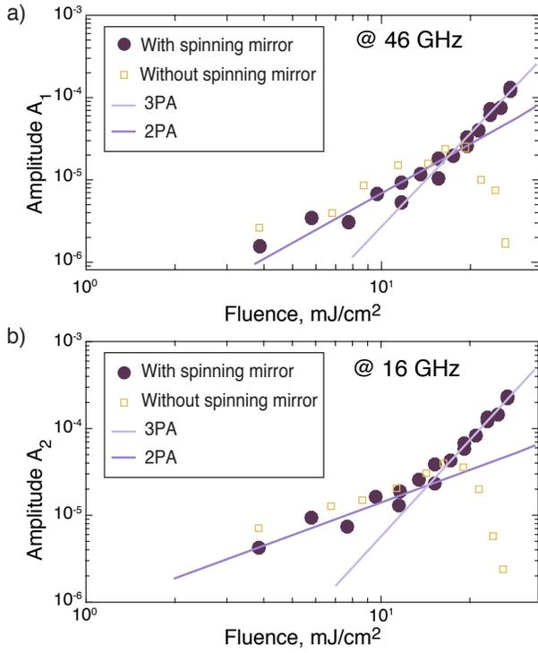
Figure 3: (Color online) Fluence dependence of (a) the 46 GHz Brillouin oscillations in glass and (b) 16 GHz oscillations. Note that the fluence  $F_0$  displayed on the graphs is the fluence measured in air.
