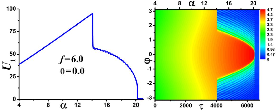
**Fig. 2.** Evolution of the intracavity power (left panel) and field distribution (right panel) upon pump frequency scan at  $\theta = 0.0$ ,  $d_{21} = -0.02$ ,  $f = 6.0$ ,  $\varepsilon = 0.4$ ,  $\delta_1 = 0.0$ ,  $\nu = 0.0025$ . All quantities are plotted in dimensionless units.
