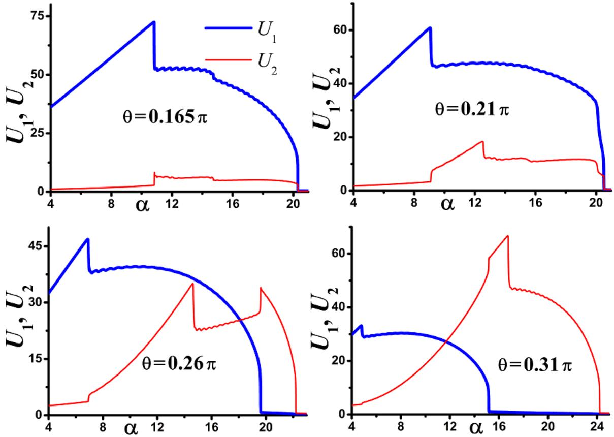
**Fig. 7.** Evolution of the intracavity powers for both polarization states upon pump frequency scan for different values of the polarization angle  $\theta$  at  $\Delta = 7.0$ ,  $d_{21} = d_{22} = -0.02$ ,  $f = 6.0$ ,  $\varepsilon = 0.4$ ,  $\nu = 0.0025$ ,  $\delta_{1,2} = 0$ . All quantities are plotted in dimensionless units.
