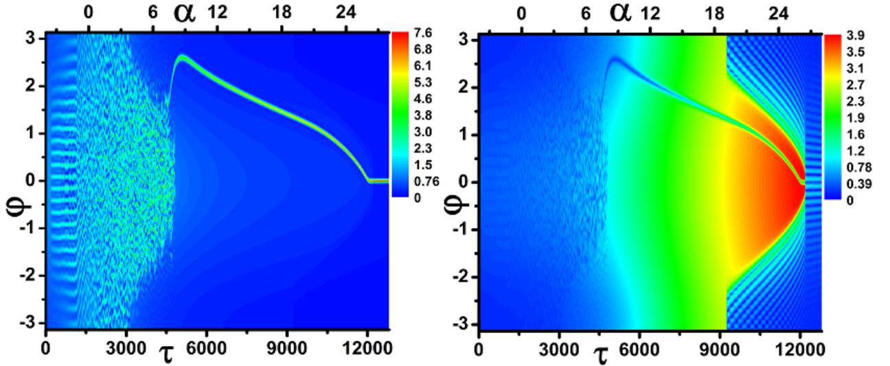
**Fig. 13.** Field distribution evolution upon pump frequency scan for the first (left panel) and second component (right panel) at  $d_{21} = 0.02$ ,  $d_{22} = -0.02$ ,  $f = 6$ ,  $\varepsilon = 0.4$ ,  $\nu = 0.0025$ ,  $\delta_{1,2} = 0$ ,  $\theta = \pi/4$ ,  $\Delta = 12.0$ . All quantities are plotted in dimensionless units.
