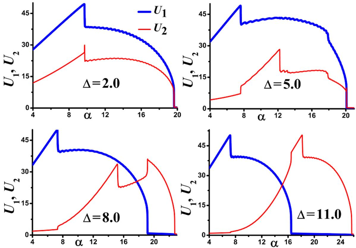
**Fig. 3.** Evolution of the intracavity powers for both polarization states upon pump frequency scan for different values of the interval between pumped modes  $\Delta$  at  $\theta = 0.25\pi$ ,  $d_{21} = d_{22} = -0.02$ ,  $f = 6.0$ ,  $\varepsilon = 0.4$ ,  $\nu = 0.0025$ ,  $\delta_{1,2} = 0$ . All quantities are plotted in dimensionless units.
