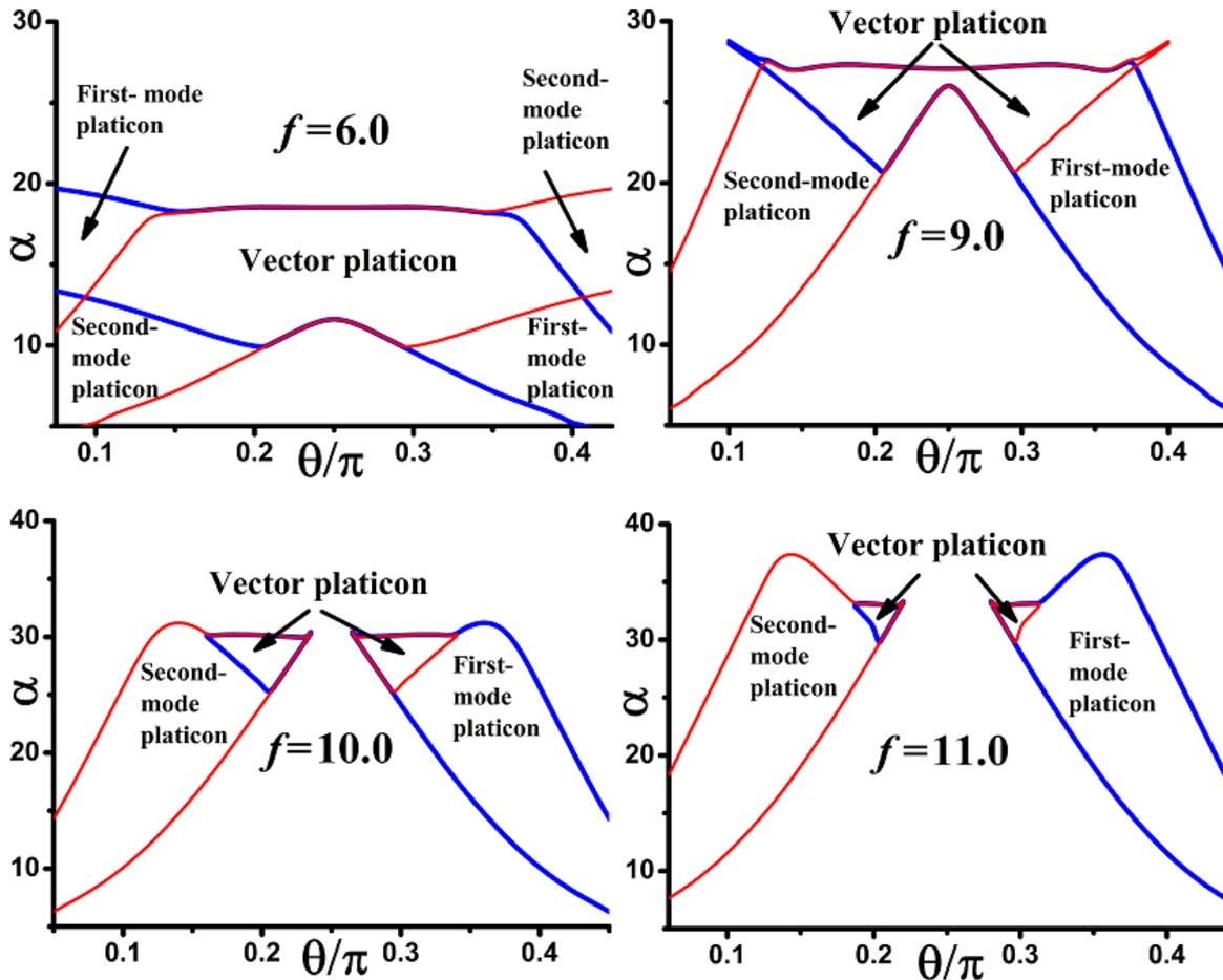
**Fig. 11.** Vector platicon generation domains for different pump amplitudes at  $d_{21} = d_{22} = -0.02$ ,  $\varepsilon = 0.4$ ,  $\nu = 0.0025$ ,  $\Delta = 0$ ,  $\delta_{1,2} = 0$ . All quantities are plotted in dimensionless units.
