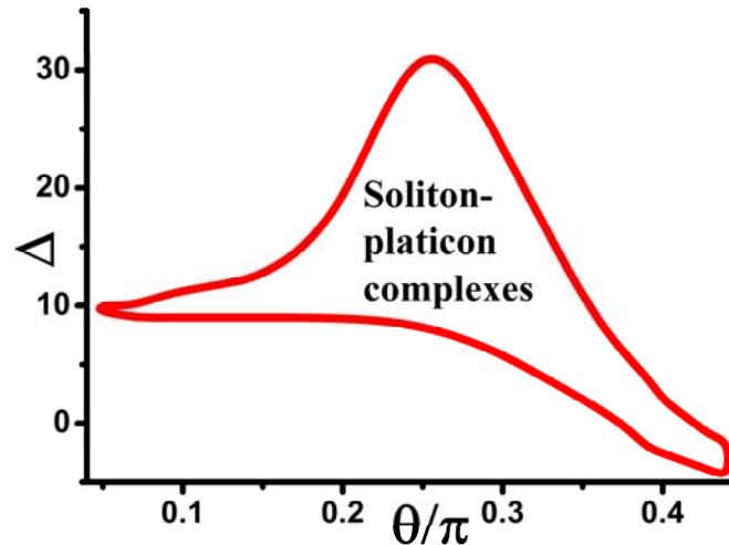
**Fig. 15.** Parameter range providing generation of soliton-platicon complexes at  $d_{21} = 0.02$ ,  $d_{22} = -0.02$ ,  $f = 6$ ,  $\varepsilon = 0.4$ ,  $\nu = 0.0025$ ,  $\delta_{1,2} = 0$  (the inner area between thick red curves). All quantities are plotted in dimensionless units.
