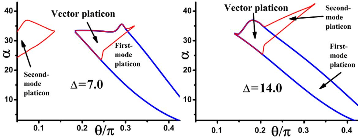
**Fig. 12.** Vector platicon generation domains for different intervals between pumped modes at  $d_{21} = d_{22} = -0.02$ ,  $f = 10$ ,  $\varepsilon = 0.4$ ,  $\nu = 0.0025$ ,  $\delta_{1,2} = 0$ . All quantities are plotted in dimensionless units.
