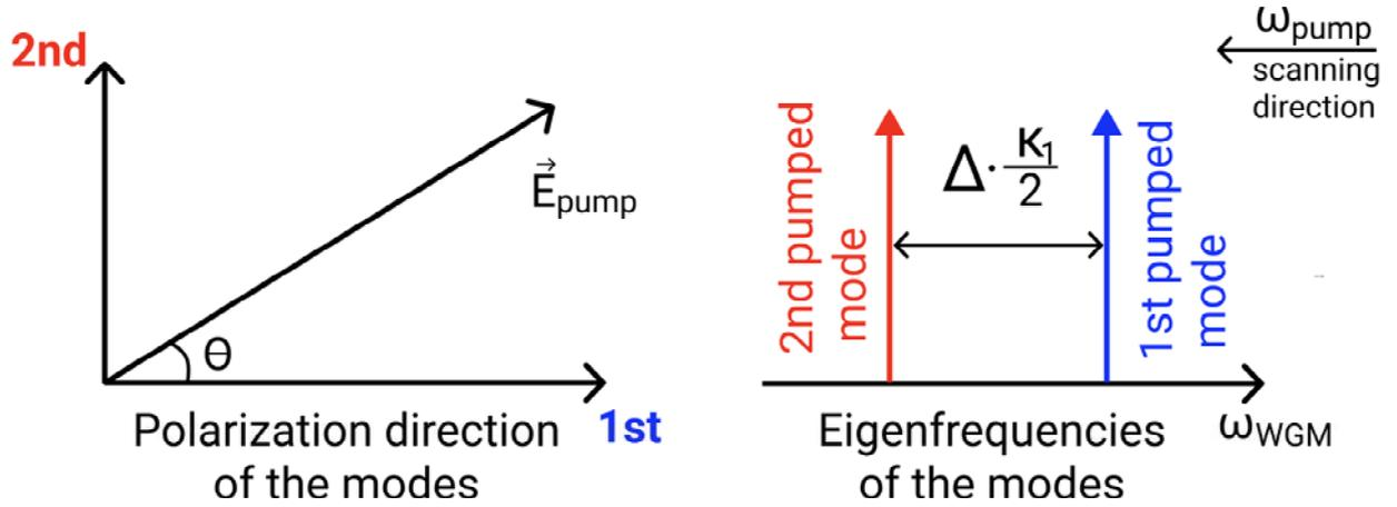
**Fig. 1.** Scheme of the process of the vector platicon generation by the simultaneous pump of the spectrally separated orthogonally polarized modes by the amplitude-modulated pump beam with linear-in-time decrease of the pump frequency.  $\theta$  is the polarization angle of the pump beam, defined relatively to the polarization directions of the pumped modes.  $\Delta$  is the spectral interval between orthogonally polarized pumped modes, normalized to  $\kappa_1/2$ .
