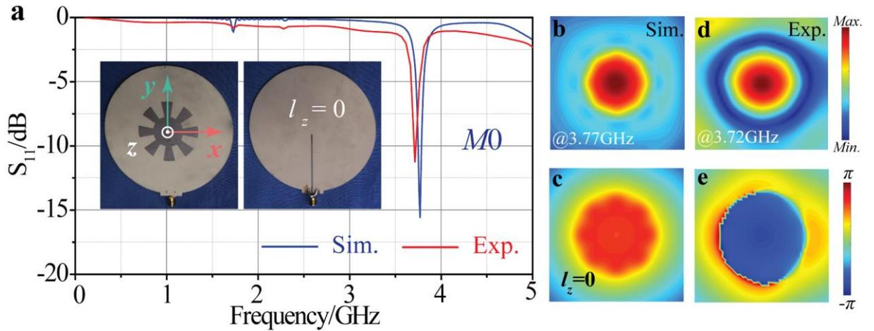
**Figure 3.** Comparison of experimental and simulation results: (a) reflection coefficient  $S_{11}$ , (b) magnitude and (c) phase distributions of the simulated  $E_z$ , and (d) magnitude and (e) phase distributions of the measured  $E_z$ . In (a), the top and bottom views of the fabricated sample are shown. Both the simulated and measured  $E_z$  show a trivial scalar vortex mode with topological charge of 0, i.e.,  $l_z = 0$ .
