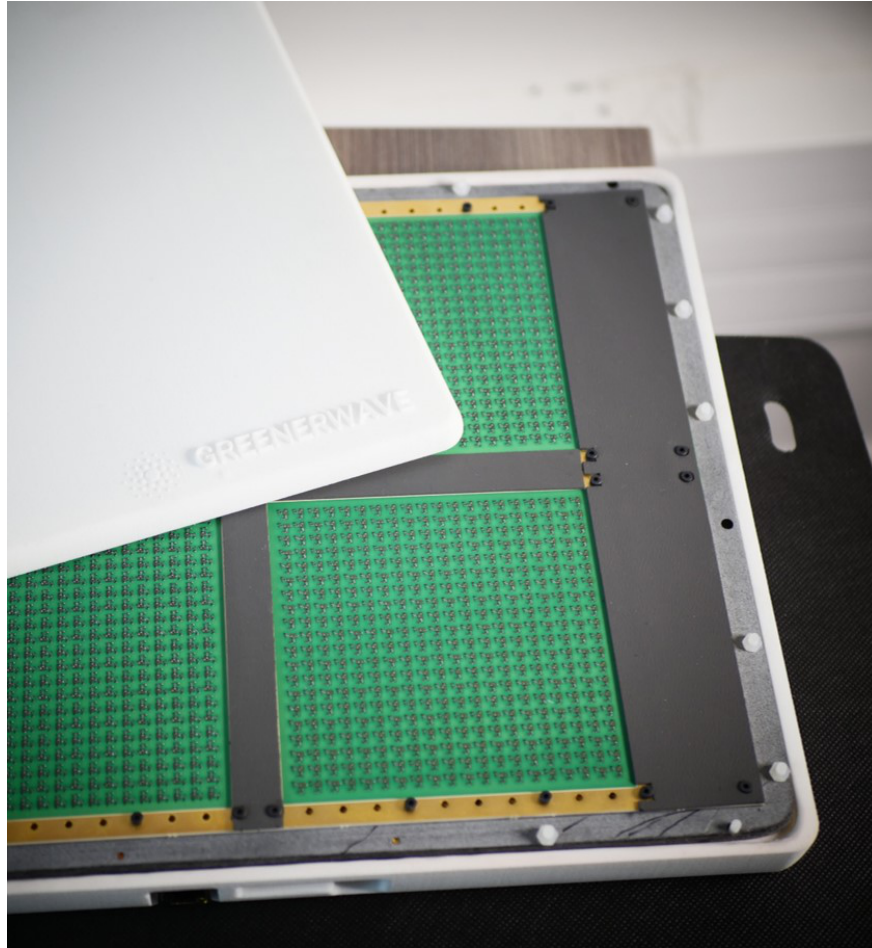
Figure 8: A 20cm*20cm dual polarized tunable metasurface at 26-30GHz, developed by Greenerwave for 5G mmWave access point extender (2021).
