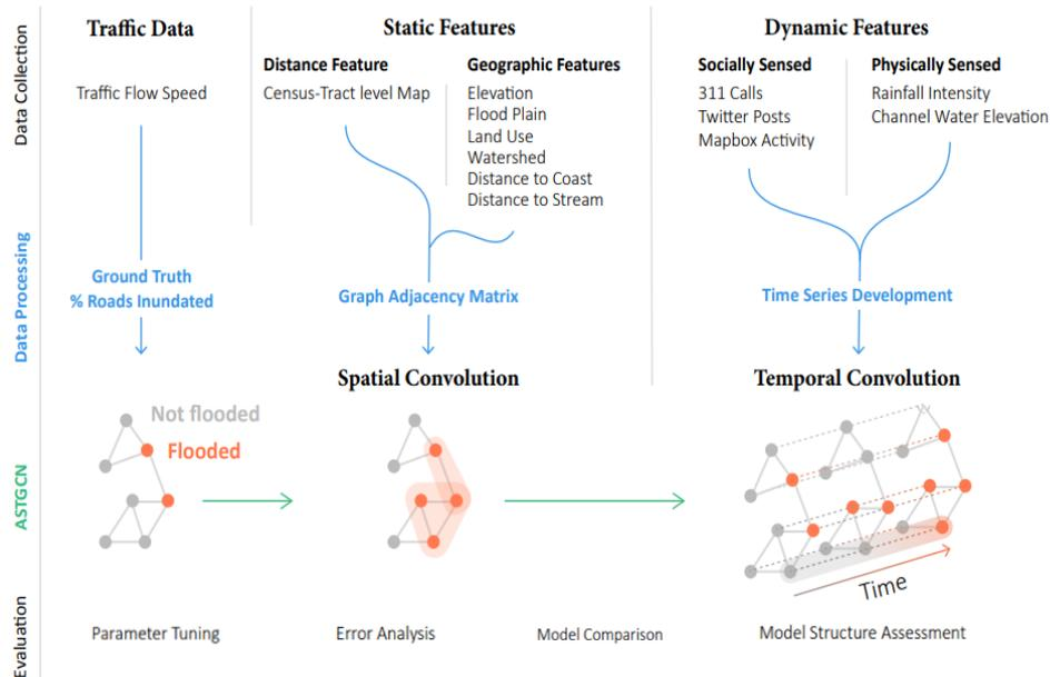
**Figure 2. Overview of the model framework, including steps for collecting and preprocessing ground truth and features, developing the ASTGCN model architecture, and evaluating the performance of the model and model performance.**
