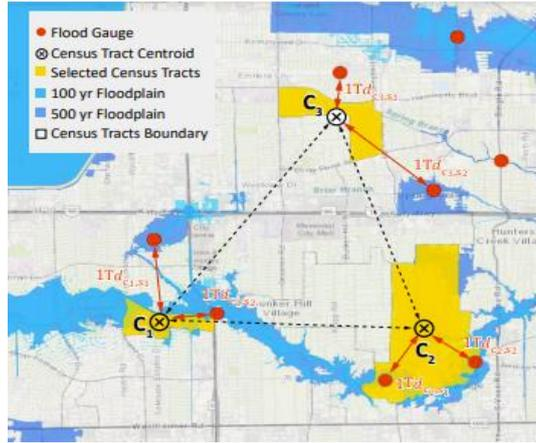
**Figure 3. Schematic illustration of calculating census tracts' distances and weights of two closest flood gauges as inputs to the census tract physics-based features.**
