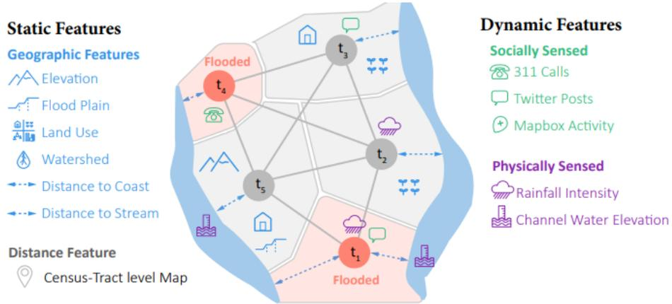
**Figure 1. Schematic representation of the problem abstraction; the study area is modeled as a graph; static features and distance are used to determine weights, and physics-based and human-sensed dynamic features are used for predicting the extent of flooding.**
