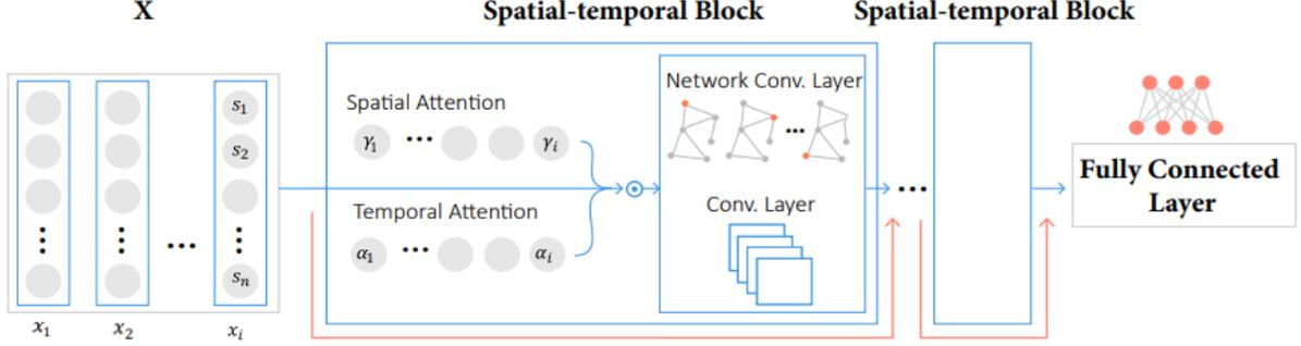
**Figure 4. Model architecture, including model input, spatial-temporal blocks, attention layers, and the fully connected layer at the end.**
