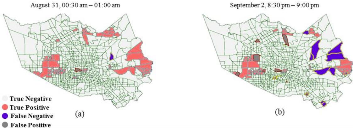
*Figure 6. An example of model flood nowcasting performance; (a) a proper prediction (August 31, 00:30 a.m.–01:00 a.m.) versus (b) model prediction with more misclassification (September 2, 8:30 p.m.–9:00 p.m.)*
