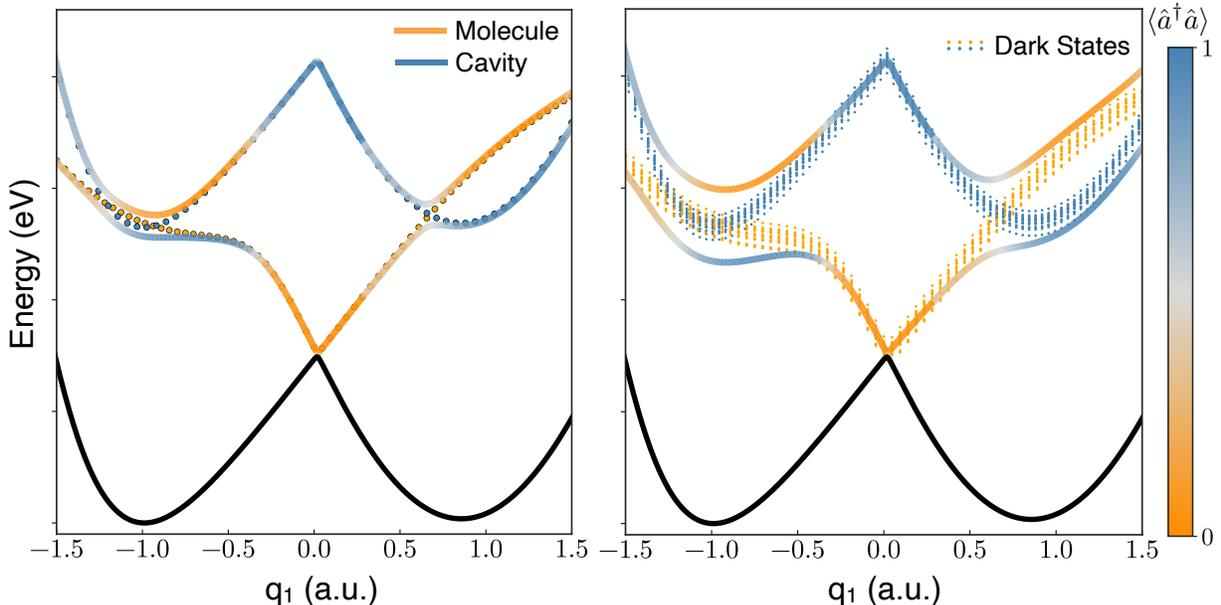
Figure 2: **Polaritonic Potential Energy Surfaces** (a) Case of a single molecule strongly coupled with light, where coupling between the cavity (blue dotted) and the molecule (orange dotted) states couple to originate polaritons. (b) Case of a molecular ensemble ( $N=50$ ), where a manifold of dark states emerges.
