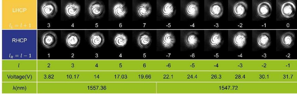
Fig. S3. The interference patterns of OAM modes whose topological charges are switched by the driving voltages. The incident wavelength is fixed at 1557.36nm for  $l=2\sim 6$  and 1547.72nm for  $l=-6\sim -1$ .
