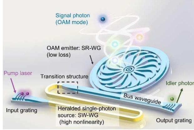
**Fig.1 The schematic of integrated heralded single-photon source with switchable OAM modes.** SW-WG: silicon wire waveguide; SR-WG: shallow ridge waveguide. Such two types of waveguides are utilized due to the features of the low transmission loss and high nonlinearity, respectively. The device is based on the silicon platform and the different colors are used to distinguish different waveguides (SW-WG and SR-WG).
