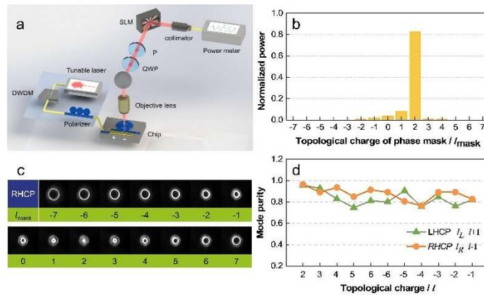
Fig.S5 a. The experimental scheme for measuring the mode purities of generated OAM modes. b. A typical result of OAM mode with  $l_R=-2$ . There are 15 values of normalized power and the value corresponding to  $l_{mask}=2$  is the required mode purity. c. The transverse intensity profiles of OAM mode after different masks which are marked below. d. The measured mode purities of both LHCP and RHCP components corresponding to 11 OAM modes.
