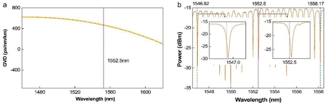
Fig.S4 a. The simulation result of the SW-WG's group velocity dispersion (GVD) versus wavelengths. b. The relation between pump/signal/idler and the transmission spectrum of OAM emitter when the operating wavelength of  $l=2$  is aligned with  $\lambda_s=1558.17$ nm.
