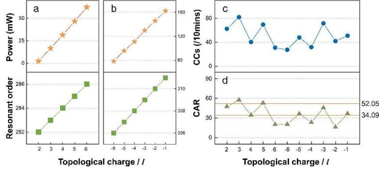
**Fig.6. The characteristics of heralded single-photon source with switchable OAM modes.** a. and b. The driving power (orange stars) and the corresponding resonant order (green squares) versus topological charge ranging within  $l=2\sim6$  and  $l=-6\sim-1$ , respectively; c. The CCs of the heralded single photons with switchable OAM modes; d. The CAR of single photons with OAM compared to that of SW-WG alone (marked as the two orange lines with values of 34.09 and 52.05, respectively).
