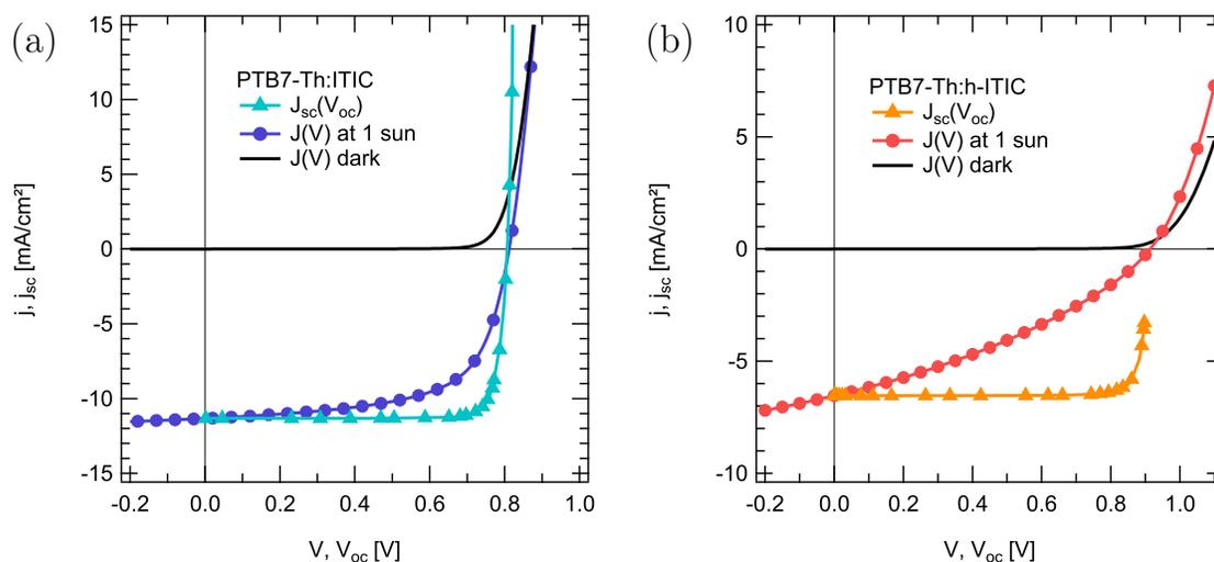
Figure S17: Pseudo- $J(V)$  curves of (a) PTB7-Th:ITIC and (b) PTB7-Th:h-ITIC constructed by shifting down the  $J_{sc}(V_{oc})$ , compared to  $J(V)$  under 1 sun illumination.
