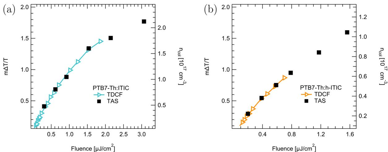
Figure S15: Transient absorption signal  $\Delta T/T$  at 5 ns (full squares) and charge carrier density  $n_{\text{col}}$  extracted from time delayed collection field at delay time of 5 ns (open triangles) for (a) PTB7-Th:ITIC and (b) PTB7-Th:h-ITIC upon excitation at 532 nm.  $n_{\text{col}}$  from TDCF is used to estimate the initial charge carrier density  $n_0$  in the global fit to the charge carrier density kinetics extracted from TAS.
