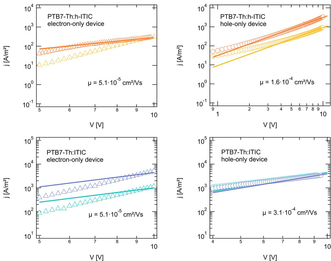
Figure S16: Charge carrier mobilities  $\mu$  of PTB7-Th:ITIC and PTB7-Th:h-ITIC solar cells determined from the fits to SCLC data of the hole-only and electron-only devices according to  $j_{\text{sclc}} = 9\epsilon\epsilon_0\mu V^2/(8L^3)$ , where  $\epsilon\epsilon_0$  is the permittivity of the organic semiconductor material,  $V$  is the applied voltage and  $L$  is the active layer thickness.
