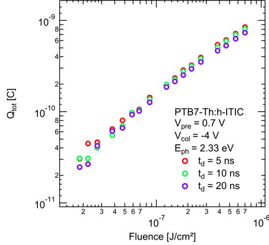
Figure S20: Total extracted charge  $Q_{tot}$  from TDCF as a function of laser pulse fluence for PTB7-Th:h-ITIC at excitation energy of 2.33 eV.  $Q_{tot}$  and its fluence dependence changes little with  $t_d$  between 5 ns and 20 ns, which confirms that the chosen delay time of 5 ns for photogeneration measurements is adequate.
