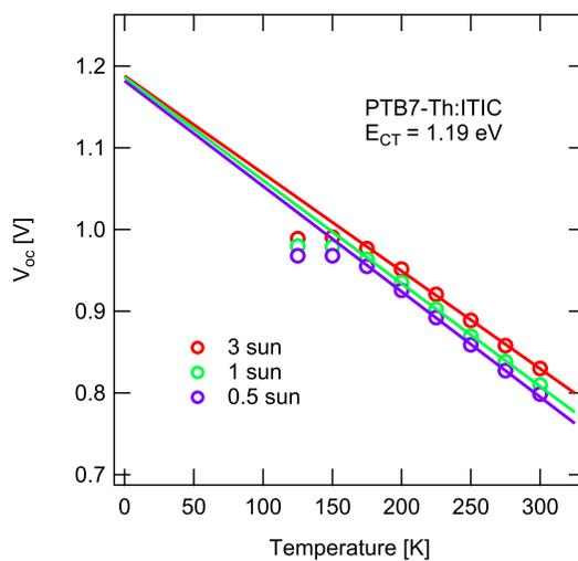
Figure S18:  $V_{oc}$  of PTB7-Th:ITIC vs temperature. Extrapolation of linear fit to 0 K gives the lower limit of charge transfer state energy  $E_{CT}$ .
