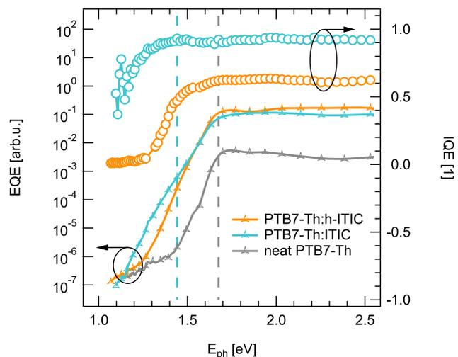
Figure 4. Sensitive EQE and IQE of PTB7-Th:ITIC and PTB7-Th:h-ITIC. EQE of neat PTB7-Th is plotted for comparison. IQE is calculated from the photocurrent normalised to the value at high reverse bias as in ref.<sup>43</sup>. IQE of h-ITIC blend is photon energy dependent below the optical gap of the donor 1.68 eV (grey dashed line), IQE of ITIC blend is energy dependent below 1.44 eV (cyan dashed line).
