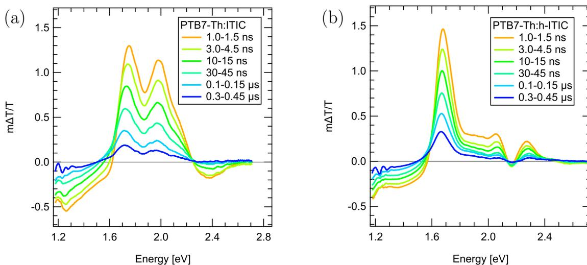
Figure S14: ns- $\mu$ s transient absorption spectra of (a) PTB7-Th:ITIC film and (b) PTB7-Th:h-ITIC film upon excitation at 532 nm with  $2.1 \mu\text{J}/\text{cm}^2$  and  $1.6 \mu\text{J}/\text{cm}^2$  fluence, respectively. The charge carrier density kinetics is monitored in the probe range of 1.6 - 2.2 eV for the ITIC and 1.6 - 1.8 eV for the h-ITIC blend film.
