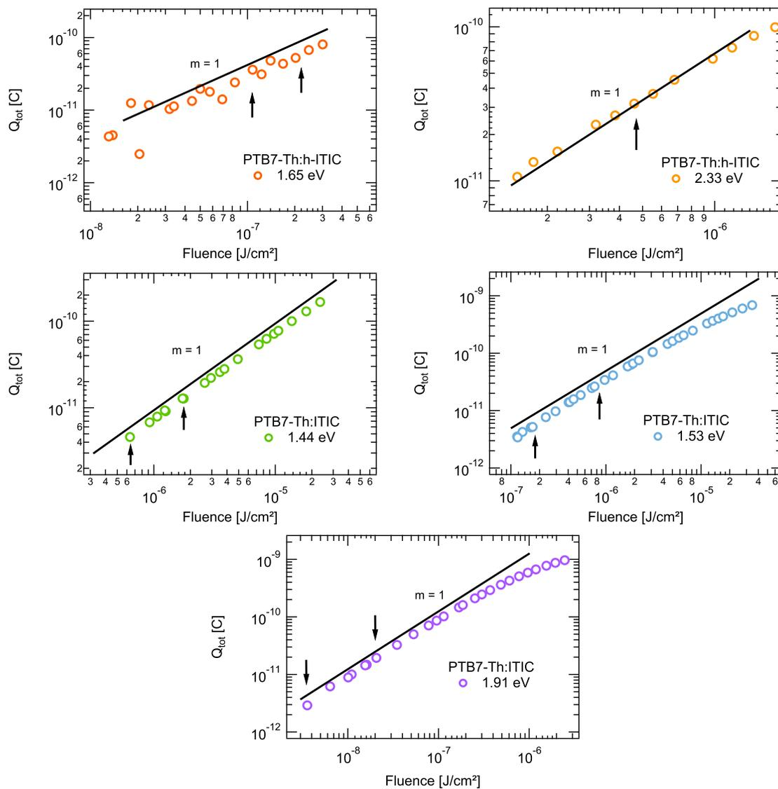
Figure S19: Total extracted charge  $Q_{\text{tot}}$  from TDCF as a function of laser pulse fluence at excitation energies of 1.65 eV and 2.33 eV for the h-ITIC blend, and 1.44 eV, 1.53 eV and 1.91 eV for the ITIC blend. Slope 1 is indicative of the absence of dominant 2<sup>nd</sup> order recombination losses during extraction. Chosen fluences for photogeneration measurements are indicated by arrows.
