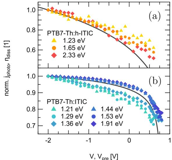
Figure 3. Dissociation yield  $\eta_{\text{diss}}$  from TDCF (symbols) as a function of prebias voltage  $V_{\text{pre}}$  for different excitation photon energies for (a) PTB7-Th:h-ITIC and (b) PTB7-Th:ITIC, compared to  $j_{\text{photo}}$  at one sun illumination intensity, normalised to the value at -2.0 V (black solid lines).
