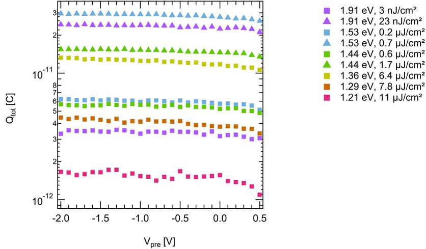
Figure S21: Total extracted charge  $Q_{tot}$  from TDCF as a function of prebias voltage  $V_{pre}$  for PTB7-Th:ITIC. Similar charge carrier density ensures that the recombination mechanisms in the device are comparable at various excitation energies.
