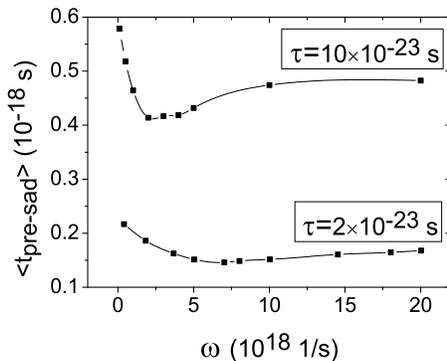
FIG. 5: The mean pre-saddle time  $\langle t_{\text{pre-sad}} \rangle$  of the non-Markovian diffusion process (71), (42) is given as a function of the frequency  $\omega$  of the harmonic time perturbation at two values of the correlation time  $\tau = 2 \times 10^{-23}$  s (lower curve) and  $\tau = 10 \times 10^{-23}$  s (upper curve).
