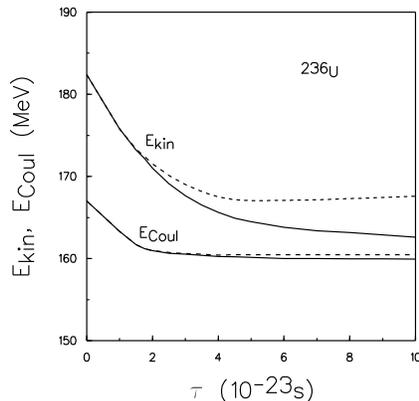
FIG. 8: Fission-fragment kinetic energy,  $E_{\text{kin}}$ , (curves 1) and the Coulomb repulsive energy at the scission point,  $E_{\text{Coul}}$ , (curves 2) versus the relaxation time  $\tau$  for the nucleus  $^{236}\text{U}$ . Solid lines represent the result of the calculation in presence of the memory effects and dashed lines are for the case of Markovian (no memory) motion with the friction forces. The initial kinetic energy is  $E_{\text{kin},0} = 1 \text{ MeV}$ .
