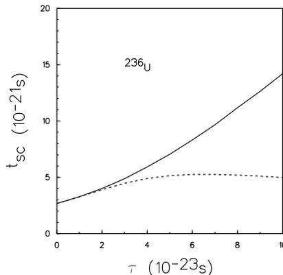
FIG. 9: Dependence upon relaxation time  $\tau$  of the saddle-to-fission time,  $t_{\text{sc}}$ , for the descent from the barrier in the case of two-dimension  $(\zeta_0, \zeta_2)$  parametrization for the nucleus  $^{236}\text{U}$ . Solid line represents the result of the calculation in presence of the memory effects and dashed line is for the case of Markovian (no memory) motion with the friction forces. The initial kinetic energy is  $E_{\text{kin}} = 1$  MeV.
