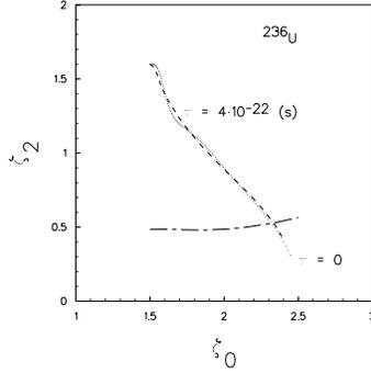
FIG. 7: Trajectories of descent from the saddle point of the nucleus  $^{236}\text{U}$  in the  $\zeta_0, \zeta_2$  plane. Dashed line represents the result of the calculation in presence of the memory effects and dotted line is for the case of Markovian (no memory) motion with the friction forces. We have used the relaxation time  $\tau = 4 \times 10^{-22}$  s and the initial kinetic energy  $E_{\text{kin}} = 1$  MeV. Dot-dashed line is the scission line derived from the condition (38).
