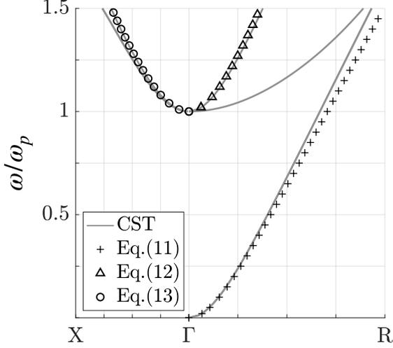
FIG. 5. Dispersion diagram for the  $X\Gamma R$  path. The grey solid lines are numerically obtained dispersion curves. The curves marked by pluses, triangles and squares are dependencies of  $D_1^{(+)}$ ,  $D_1^{(-)}$  and  $A_x^{(+)}$  calculated analytically by Eqs. (11), (12) and (13), respectively. The points in the Brillouin zone have coordinates:  $\Gamma = (0, 0, 0)^T$ ,  $X = (\pi/a, 0, 0)^T$ ,  $R = (\pi/a, \pi/a, \pi/a)^T$ .
