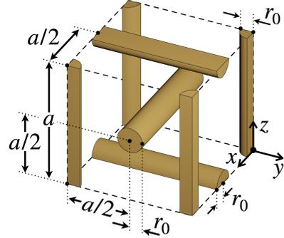
FIG. 1. A unit cell of the triple non-connected wire medium.
