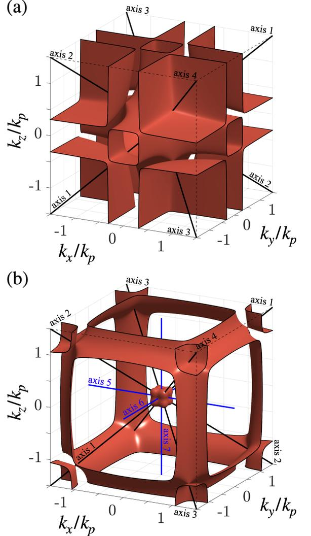
FIG. 2. Isofrequency surfaces of metamaterial with permittivity tensor  $\bar{\bar{\epsilon}}(\omega, \mathbf{k})$  described by Eq. (1) obtained by numerical solution of Eq. (7) for frequencies (a)  $\omega = 0.3\omega_p$  and (b)  $\omega = 1.01\omega_p$ : below and right above the plasma frequency, respectively.
