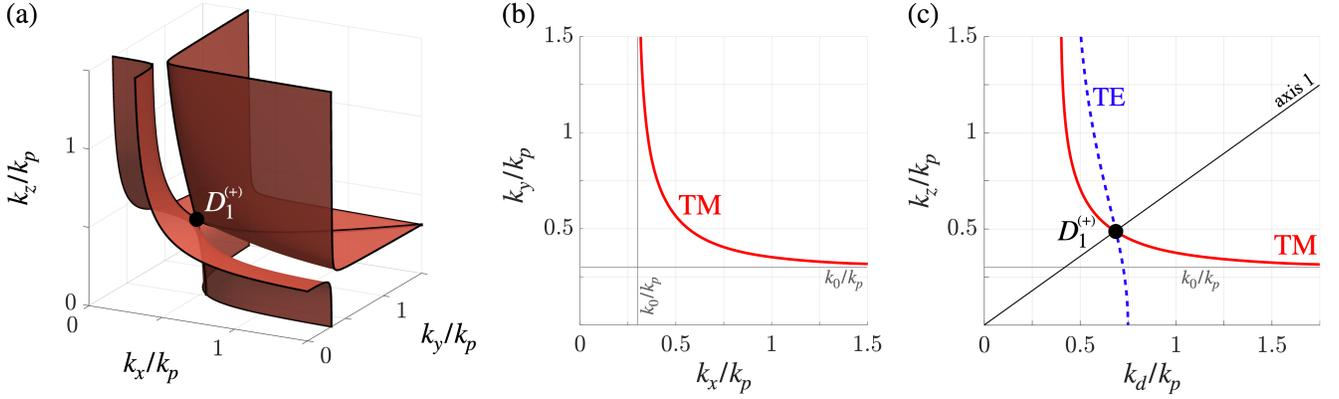
FIG. 3. (a) Isofrequency surface within the first octant for  $\omega = 0.3\omega_p$  and isofrequency contours (b) in  $kz = 0$  plane and (c) in  $kx = ky$  plane ( $k_d^2 = k_x^2 + k_y^2$ ). The conical point in this octant is marked by  $D_1^{(+)}$ .
