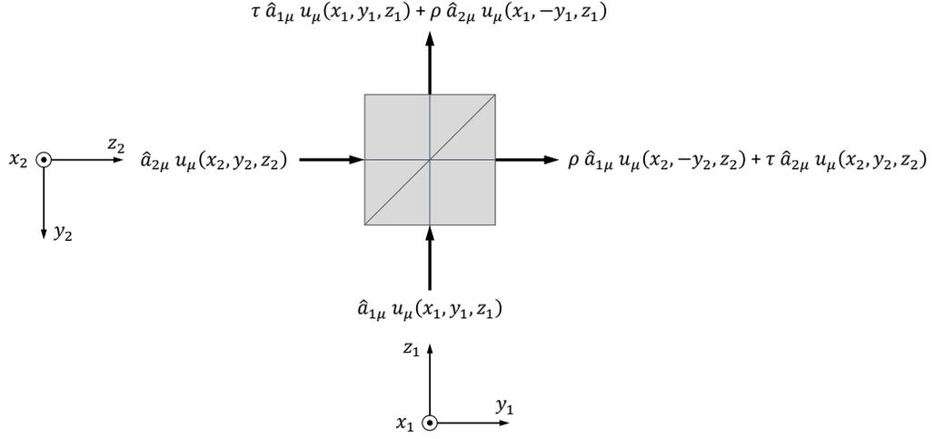
FIG. 1. Schematic illustration of a beam splitter. In this figure the Cartesian coordinate systems  $\mathbf{r}_1 = (\mathbf{x}_1, z_1)$  and  $\mathbf{r}_2 = (\mathbf{x}_2, z_2)$  are attached to the two input ports of the device. The coordinate axes  $x_1$  and  $x_2$  are shown directed towards the viewer. Note that under reflection  $u_{\mu}(x_1, y_1, z_1) \rightarrow u_{\mu}(x_2, -y_2, z_2)$  and  $u_{\mu}(x_2, y_2, z_2) \rightarrow u_{\mu}(x_1, -y_1, z_1)$ .
