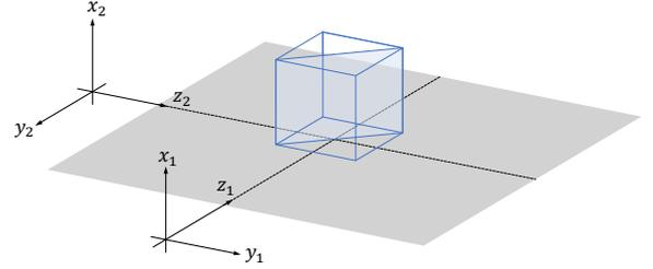
FIG. 1. Schematic illustration of a cube beam splitter. This figure shows the distinct Cartesian coordinate systems  $\mathbf{r}_1 = (x_1, y_1, z_1)$  and  $\mathbf{r}_2 = (x_2, y_2, z_2)$  attached to the two input ports of the device.
