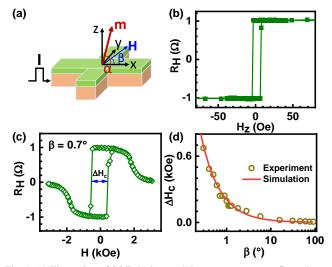
Fig. 1. (a) Illustration of SOT-devices and the measurement configurations. (b) The perpendicularly magnetized hysteresis loop. (c)  $R_H$  as a function of in-plane field when  $\beta = 0.7^{\circ}$ , where  $\Delta H_c$  is defined. (d) The extracted  $\Delta H_c$  as a function of  $\beta$ . The solid line is the simulated result based on the coherent switching.
