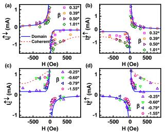
Fig. 4. The extracted I<sub>c</sub> for (a, c)  $\uparrow \downarrow$  and (b, d)  $\downarrow \uparrow$  switching with (a, b) positive and (c, d) negative  $\beta$ . The solid and dash lines represent the predicted values for the domain expansion switching and coherent switching, respectively. The parameters are  $\varepsilon H_k = 0.15$  T,  $\beta = 0.3^\circ$ ,  $\delta M_s = 5 \times 10^4$  A/m, and  $\theta_{SH} = 0.2$ . the CoFeB layer and then the sensing current was applied to
