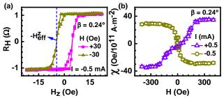
Fig. 3. (a) Perpendicularly magnetized  $R_H$  loops under an in-plane field  $H = \pm 30$ Oe with  $\beta = 0.24^\circ$ . The shift of  $R_H$  loops corresponds to  $H^z_{eff}$ . (b) The measured  $\chi$  as a function of H when  $\beta = 0.24^\circ$ .
