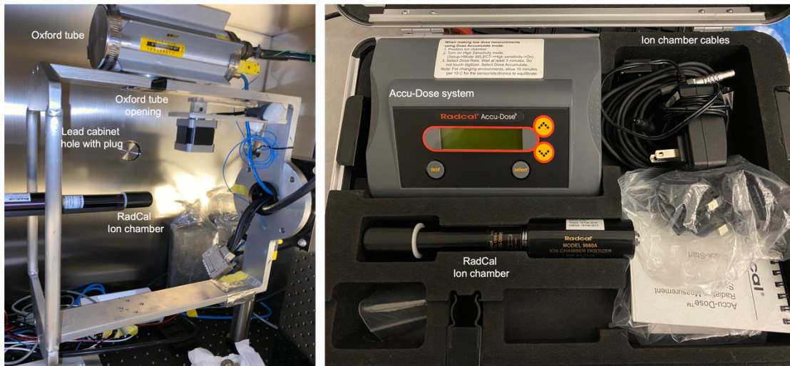
Figure 1: Experimental acquisition setup (left) and the Accu-Dose system (right). The Accu-Dose system was positioned outside of the lead cabinet for user control.
