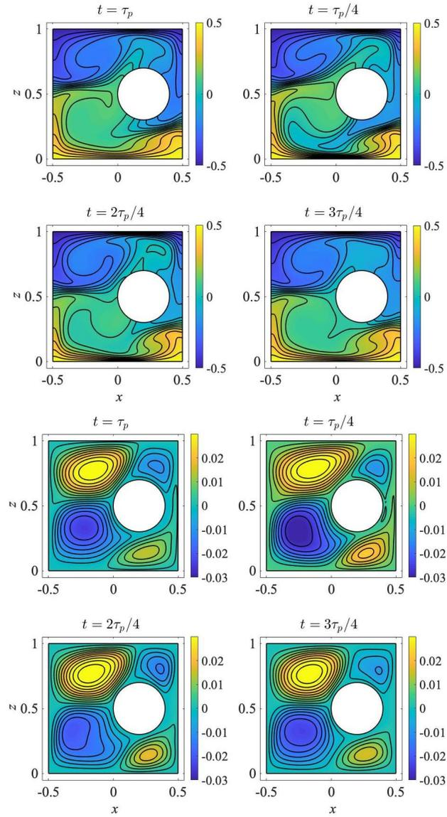
Figure 8: Top two rows: temperatures for side obstruction case with  $Ra = 10^6$  at intervals of one-period in the behavior. Bottom two rows: streamlines for side obstruction case with  $Ra = 10^6$  at the same time steps.
