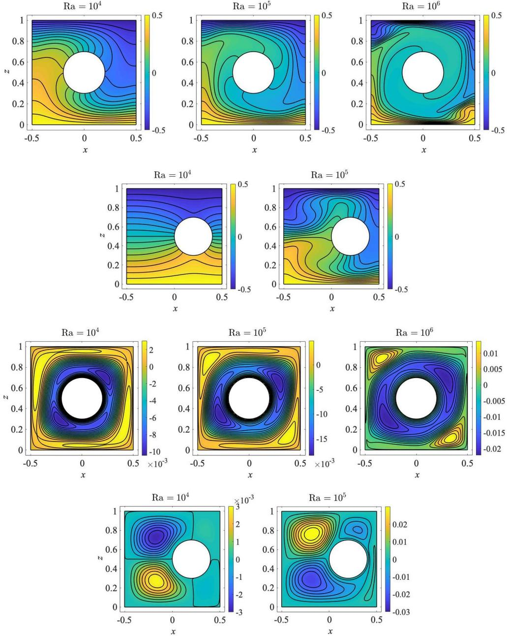
Figure 7: Top two rows: temperature profiles for a middle obstruction with  $Ra = 10^4$ ,  $10^5$ ,  $10^6$  at their steady-states, and the side obstruction cases with  $Ra = 10^4$  and  $Ra = 10^5$  only. Bottom two rows: streamline contours for the same simulations.
