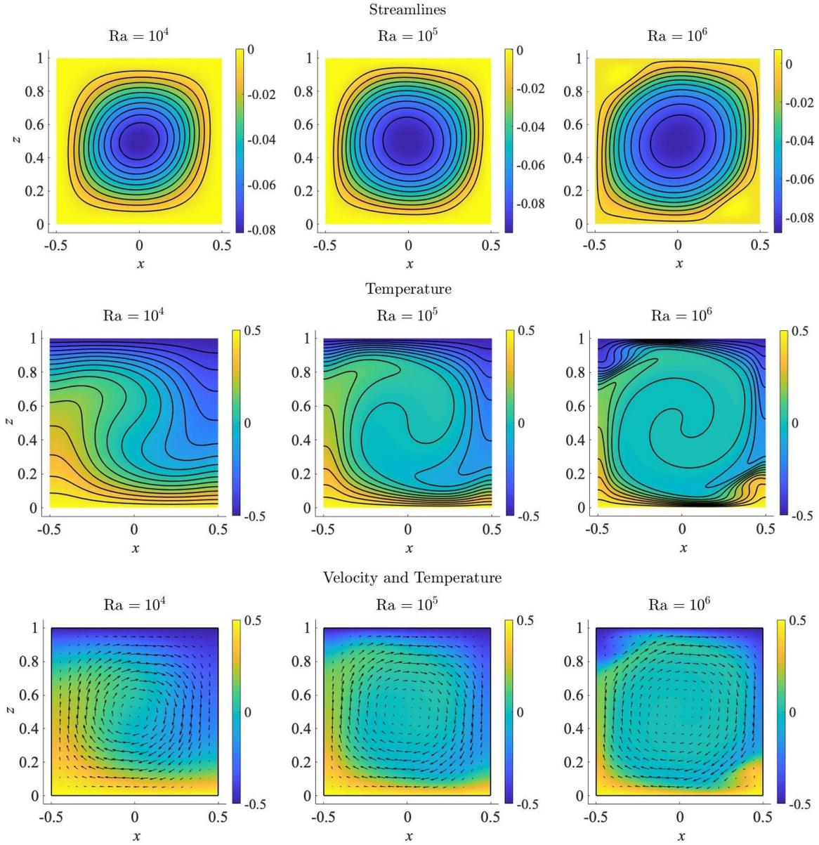
Figure 4: Top row: streamline contours, middle row: temperature profile contours, bottom row: velocity field and temperature fields. Each column represents a different Rayleigh number, with  $Ra = 10^4$ ,  $Ra = 10^5$ , and  $Ra = 10^6$  as the three columns, respectively.
