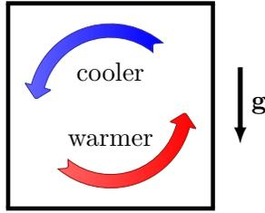
Figure 1: Schematic of a Rayleigh-Bénard convection cell.
