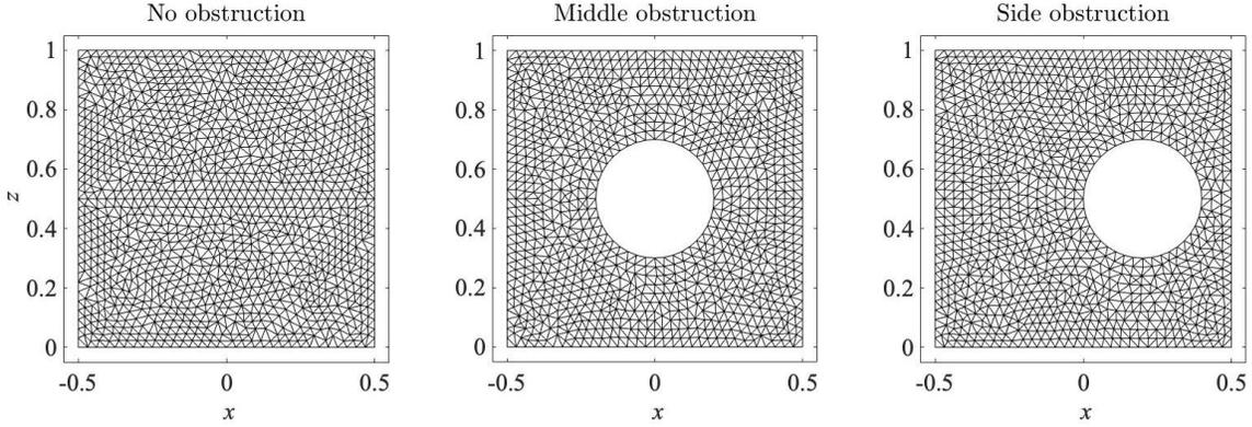
Figure 2: Schematic of meshes for domains with no obstruction, middle obstruction, and side obstruction, respectively.
