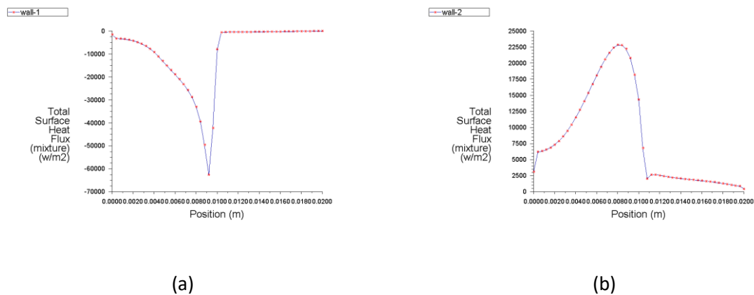
Figure 15: Figure 14: Wall heat flux at Ma = 1 \times 10^5 for (a) left wall (b) right wall
