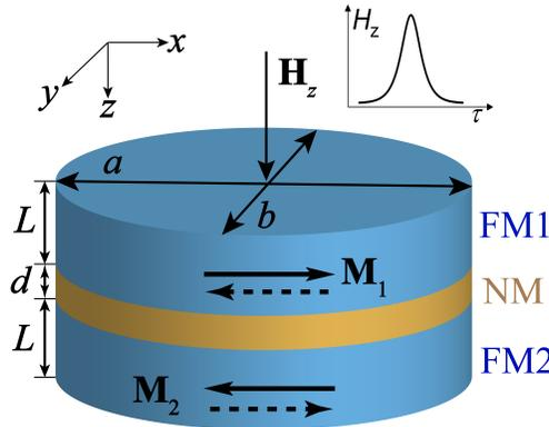
**Figure 1.** Schematic of SAF cell. Two ferromagnetic layers with magnetizations  $\mathbf{M}_1$  and  $\mathbf{M}_2$  and thickness  $L$  are separated by nonmagnetic spacer with thickness  $d$ . A pulse of out-of-plane exciting magnetic field  $\mathbf{H}_z$  of certain duration and amplitude is produced either by external field coil or circularly polarized laser pulse (see Section: Switching SAF optically).
