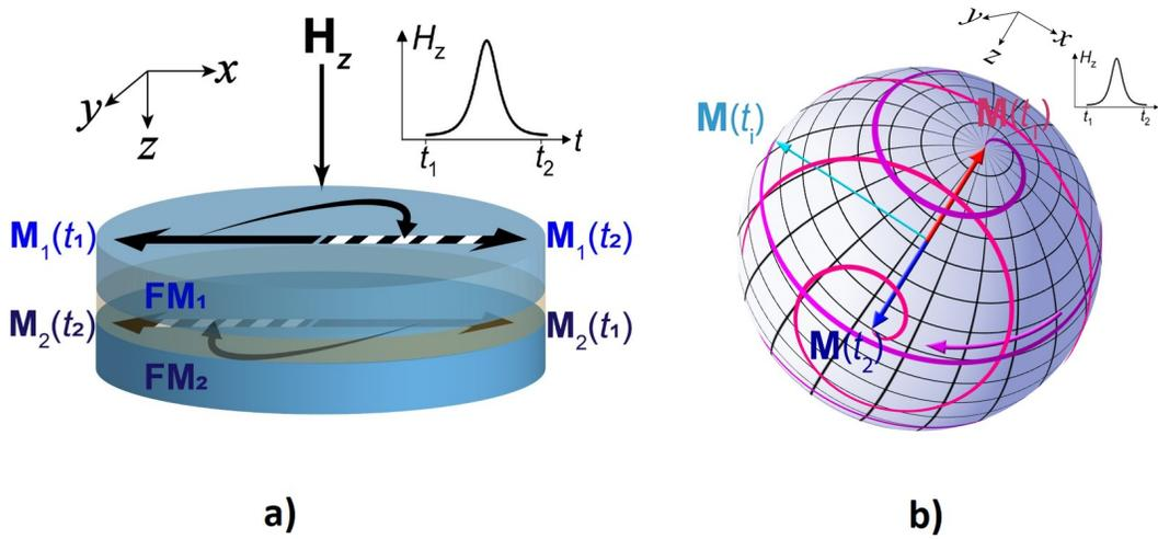
**Figure 3.** Illustration of barrier-free and relaxation-free switching in SAF, coinciding in time with half-period of in-phase in-plane rotation (a), which is much faster than conventional out-of-phase switching of a ferromagnetic particle with subsequent precessional relaxation (b).
