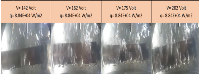
Fig. 8. Developing boiling steps for distilled water and aqueous SiO 2 solutions of different concentrations, using smooth tube surface
