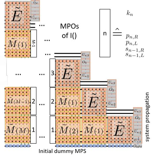
Figure 3. TN for  $\langle T_{\leftarrow} A_1(t_1) \dots A_N(t_N) \rangle$ . On the right edge of the TN the MPS decomposed system propagators  $U_{s,m-1/2}$  (cf. Eq.(2)) are connected to the indices  $s$  and  $p$ . The majority of network is constructed from the decomposed  $\tilde{M}$  and  $\tilde{E}$  tensors. An initial MPS is at the bottom.
