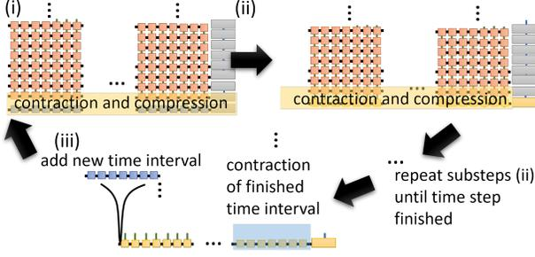
Figure 4. (i) Application of next MPO to the current MPS (initially a dummy MPS) (ii) repeated until all tensors of  $\Delta T$  are contracted, then (iii) removal of the current interval, and extension for future intervals. (i) Repeated, until finished.
