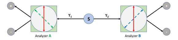
Figure 4: Schematic representation of Aspect's experiment, as described in [1]. The red line indicates the initial orientation of A and B. The green dashed line indicates A is oriented in the counter-clockwise direction while the blue dashed line indicates B is oriented in the clockwise direction. The angle between A and B is used to calculate the probability of the outcome.
