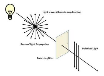
Figure 2: Light source producing unpolarized light which passes through a polarizer to produce a polarized light wave. Web Reference: https://www.researchgate.net/publication/ 328100369\_Polarised\_infrared\_light\_enables\_enhancement\_of\_histo-morphological\_ diagnosis\_of\_prostate\_cancer
