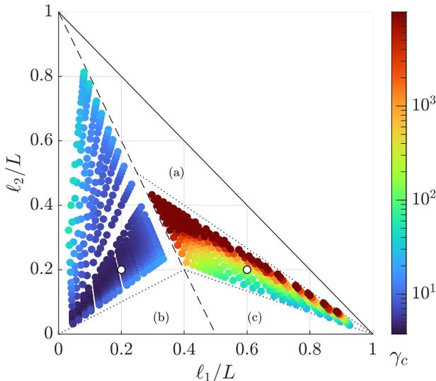
FIG. 4. Bifurcation value  $\gamma_c$  with respect to the ratios  $l_1/L$  and  $l_2/L$ . The dashed line separates the  $l_1 < l_3$  region on the left (puller case) from the  $l_1 > l_3$  region on the right (pusher case). In areas (a), (b), and (c), delineated by indicative dotted lines, no bifurcation can be observed. White dots represent the values used in Fig. 2.
