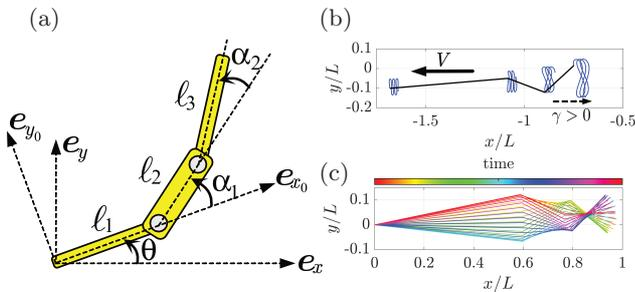
FIG. 1. (a) Schematic of Purcell's three-link swimmer. (b) An example trajectory of each end of the three rods in self-organized swimming (in the  $-x$  direction) for a pusher swimmer with  $\gamma > \gamma_c$ . (c) Rod shape of the same swimmer as (b) superimposed with its left-most rod end being translated to the origin. The colors indicate the time increment over one beat period.
