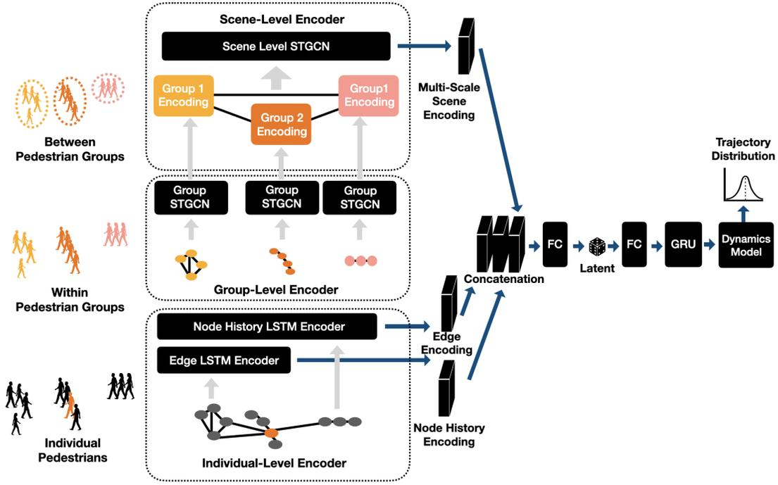
Fig. 2. The diagram of the Grouptron model, which creates spatio-temporal graphs for different levels and encodes these graphs using different networks. Combining encodings for the individual level, the group level, and the scene level, Grouptron then uses a GRU decoder to output the predictions.
