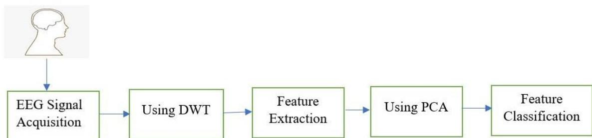
**Figure 1.** Block diagram of EEG signal to feature classification.
