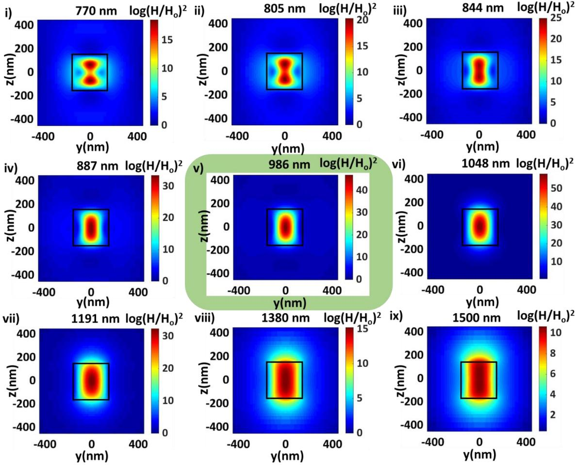
**Figure S4b (I).** FDTD-simulated spatial distribution of enhancement in magnetic field intensity  $[H^2/H_0^2]$  in YZ plane at different wavelengths across the lowest energy Mie resonance peak wavelength (i.e., 986 nm) for  $\text{Cu}_2\text{O}$  cube of 286 nm edge length.
