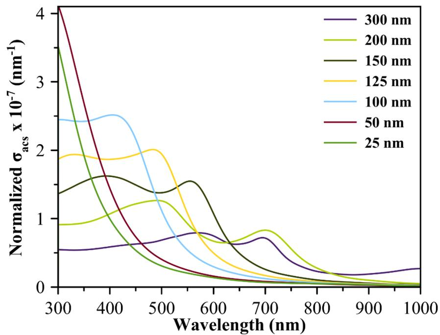
**Figure S5b.** FDTD-simulated volume-normalized absorption cross section ( $\sigma_{acs}$ ) as a function of incident light wavelength for  $\text{Cu}_2\text{O}$  nanocubes of different sizes.
