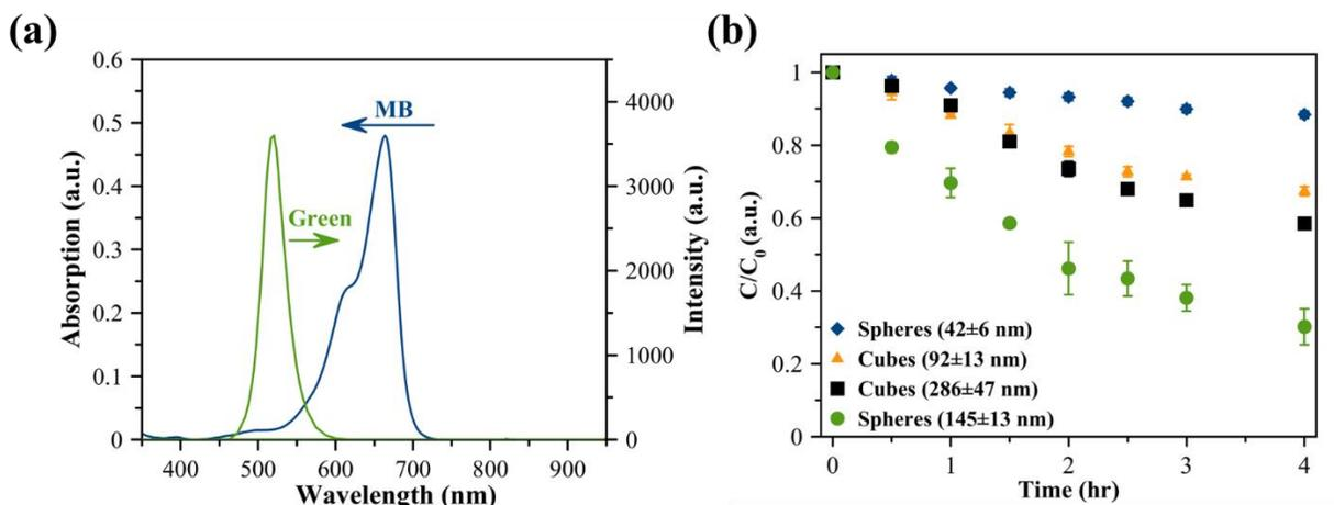
**Figure 3.** (a) Absorption spectrum of MB (left ordinate) and spectrum of green LED light source used for photocatalytic degradation of MB (right ordinate). (b) Plot of  $C/C_0$  versus irradiation time for photocatalytic degradation of MB using 42-nm  $\text{Cu}_2\text{O}$  nanospheres (blue diamonds), 92-nm  $\text{Cu}_2\text{O}$  nanocubes (orange triangles), 286-nm  $\text{Cu}_2\text{O}$  nanocubes (black squares), and 145-nm  $\text{Cu}_2\text{O}$  nanospheres (green circles).
