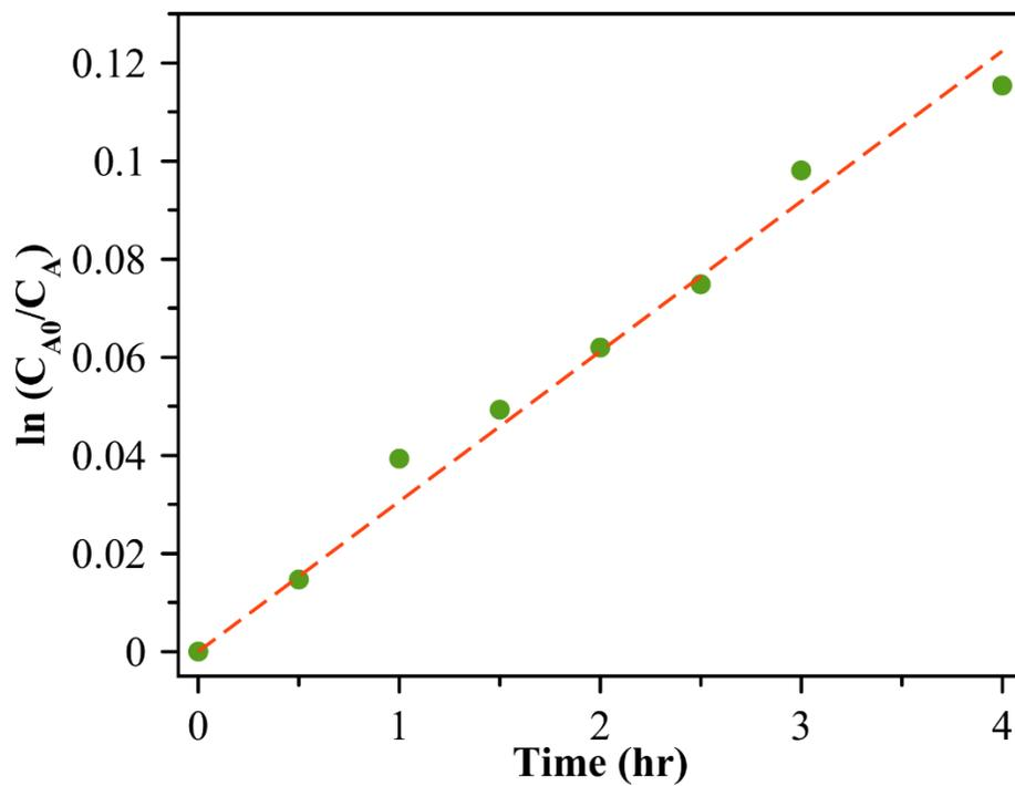
**Figure S5c.** Representative plot of empirical fit with first-order  $\ln(C_{A0}/C_A)$  versus irradiation time for photocatalytic degradation of MB under green light illumination using  $\text{Cu}_2\text{O}$  nanospheres of  $42 \pm 6$  nm diameter.
