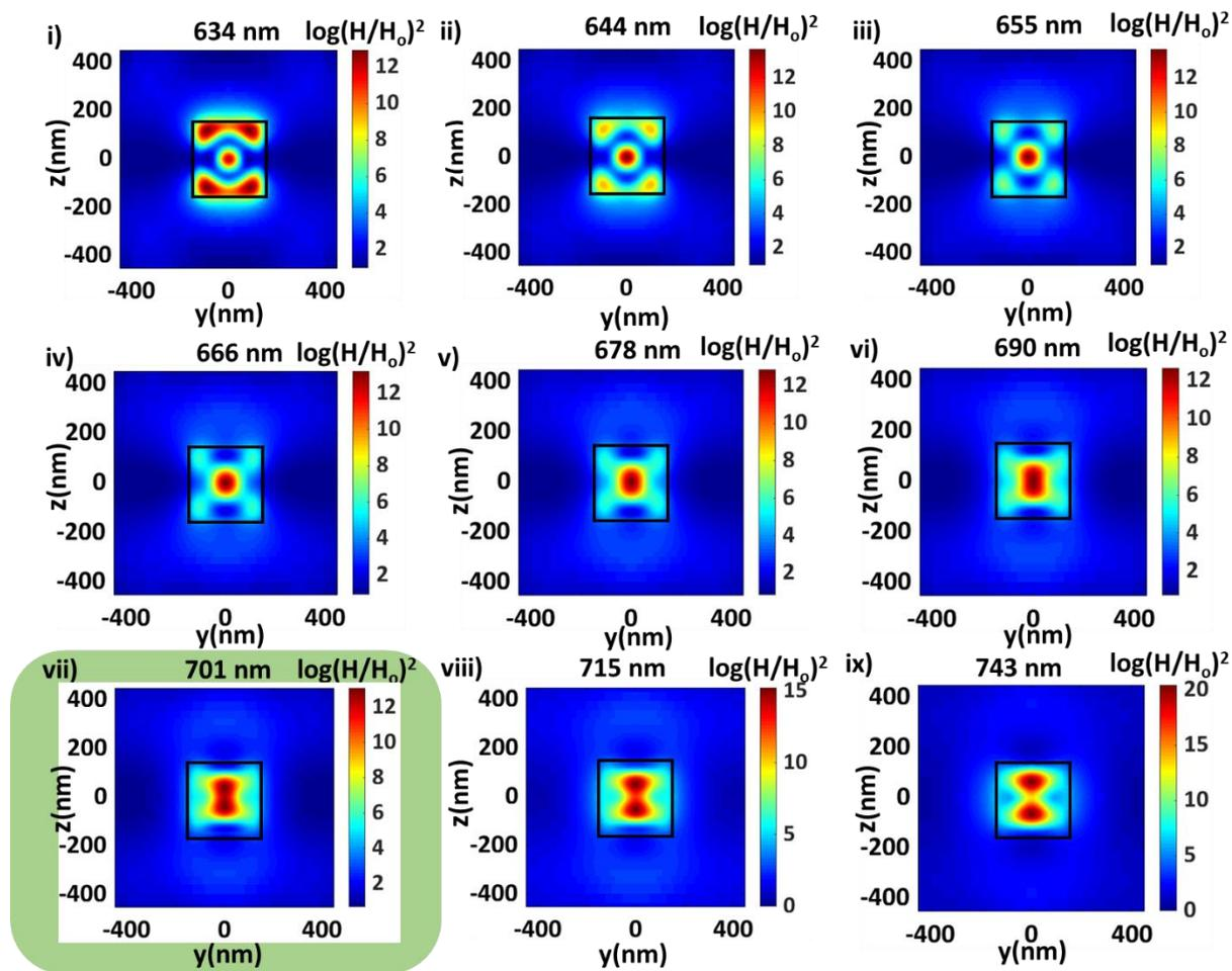
**Figure S4b (II).** FDTD-simulated spatial distribution of enhancement in magnetic field intensity  $[H^2/H_0^2]$  in YZ plane at different wavelengths across the second lowest energy Mie resonance peak wavelength (i.e., 701 nm) for  $\text{Cu}_2\text{O}$  cube of 286 nm edge length.
