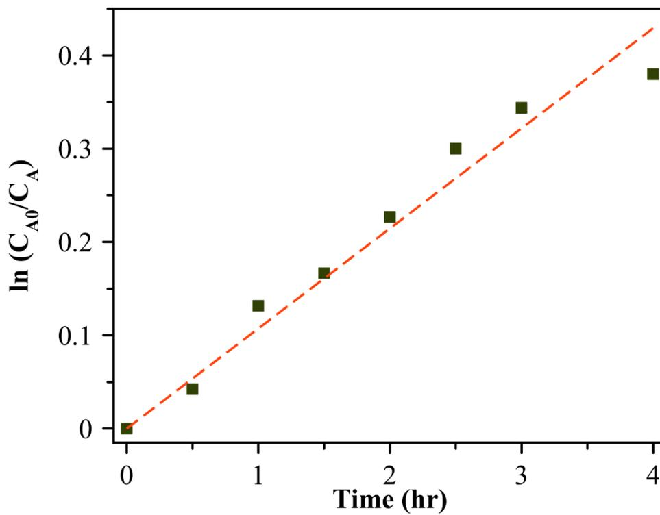
**Figure S5f.** Representative plot of empirical fit with first-order  $\ln(C_{A0}/C_A)$  versus irradiation time for photocatalytic degradation of MB under green light illumination using  $\text{Cu}_2\text{O}$  nanocubes of  $92 \pm 13$  nm edge length.
