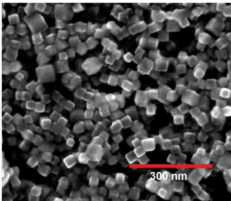
**Figure S6a.** Representative transmission electron microscopy image of  $\text{Cu}_2\text{O}$  nanocubes of  $33 \pm 6$  nm edge length.
