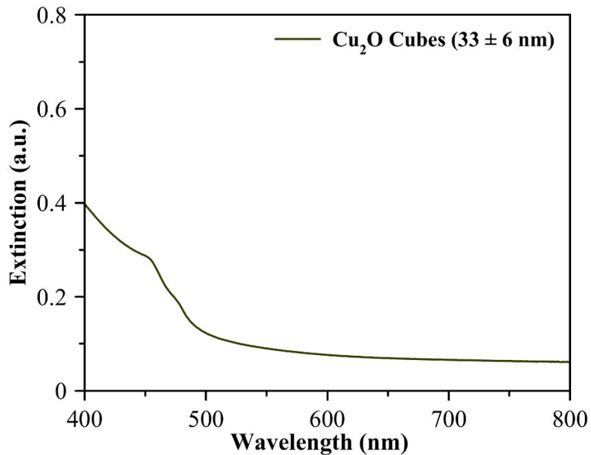
**Figure S6c.** UV-Vis extinction spectra of Cu<sub>2</sub>O nanocubes of 33 ± 6 nm edge length.
