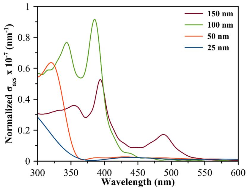
**Figure S7c.** FDTD-simulated volume-normalized absorption cross section ( $\sigma_{acs}$ ) as a function of incident light wavelength for  $\text{TiO}_2$  spherical nanoparticles of different sizes.
