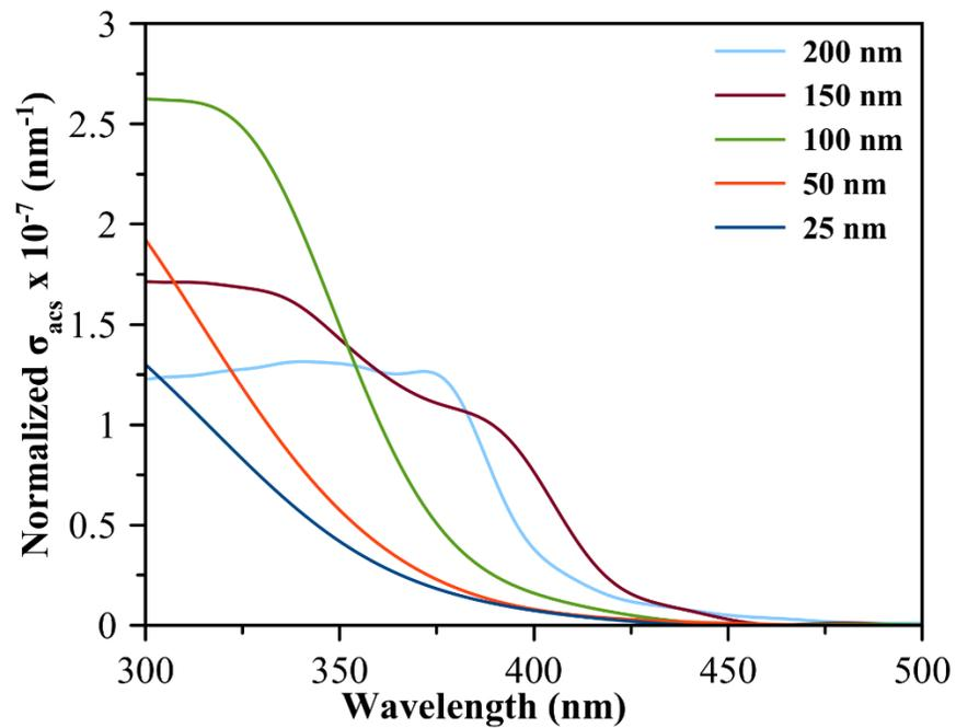
**Figure S7b.** FDTD-simulated volume-normalized absorption cross section ( $\sigma_{acs}$ ) as a function of incident light wavelength for  $\text{CeO}_2$  spherical nanoparticles of different sizes.
