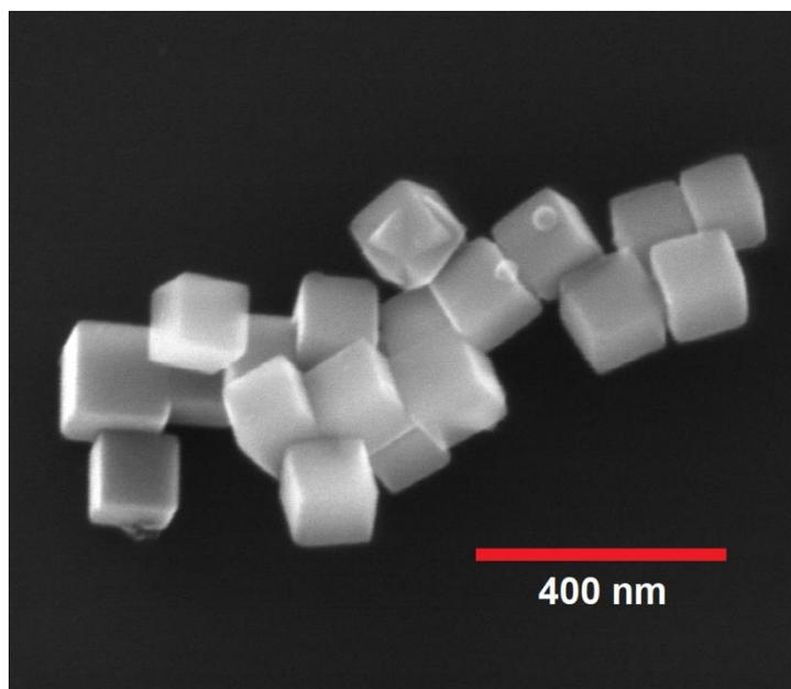
**Figure S6b.** Representative transmission electron microscopy image of  $\text{Cu}_2\text{O}$  nanocubes of  $118 \pm 21$  nm edge length.
