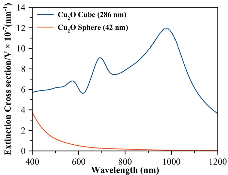
**Figure S4a.** FDTD-simulated volume-normalized extinction cross section of large  $\text{Cu}_2\text{O}$  nanocube of 286 nm edge length and small  $\text{Cu}_2\text{O}$  nanospheres of 42 nm diameter.
