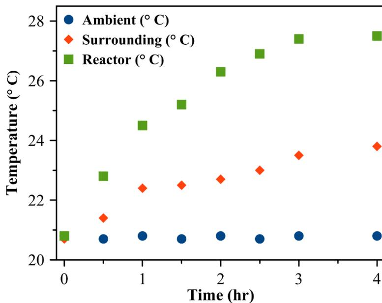
**Figure S3a.** Temperature profile measured as a function of irradiation time during photocatalytic degradation of MB under blank conditions in the absence of photocatalyst. The data represented by green squares, red diamonds, and blue circles show the temperature of the sample in the photoreactor, temperature of the reactor surrounding, and ambient room temperature of the laboratory, respectively.
