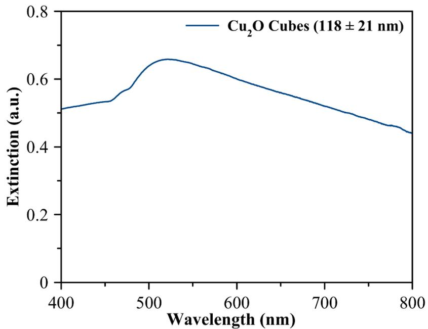
**Figure S6d.** UV-Vis extinction spectra of Cu<sub>2</sub>O nanocubes of 118 ± 21 nm edge length.
