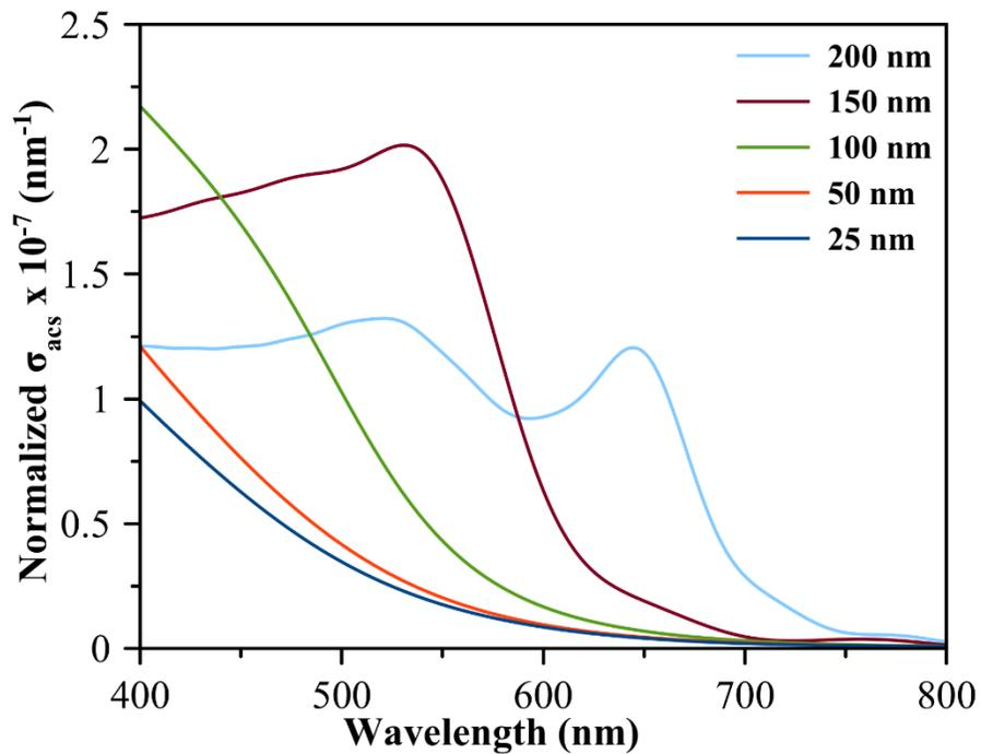
**Figure S7a.** FDTD-simulated volume-normalized absorption cross section ( $\sigma_{acs}$ ) as a function of incident light wavelength for  $\alpha$ - $\text{Fe}_2\text{O}_3$  nanospherical particles of different sizes.
