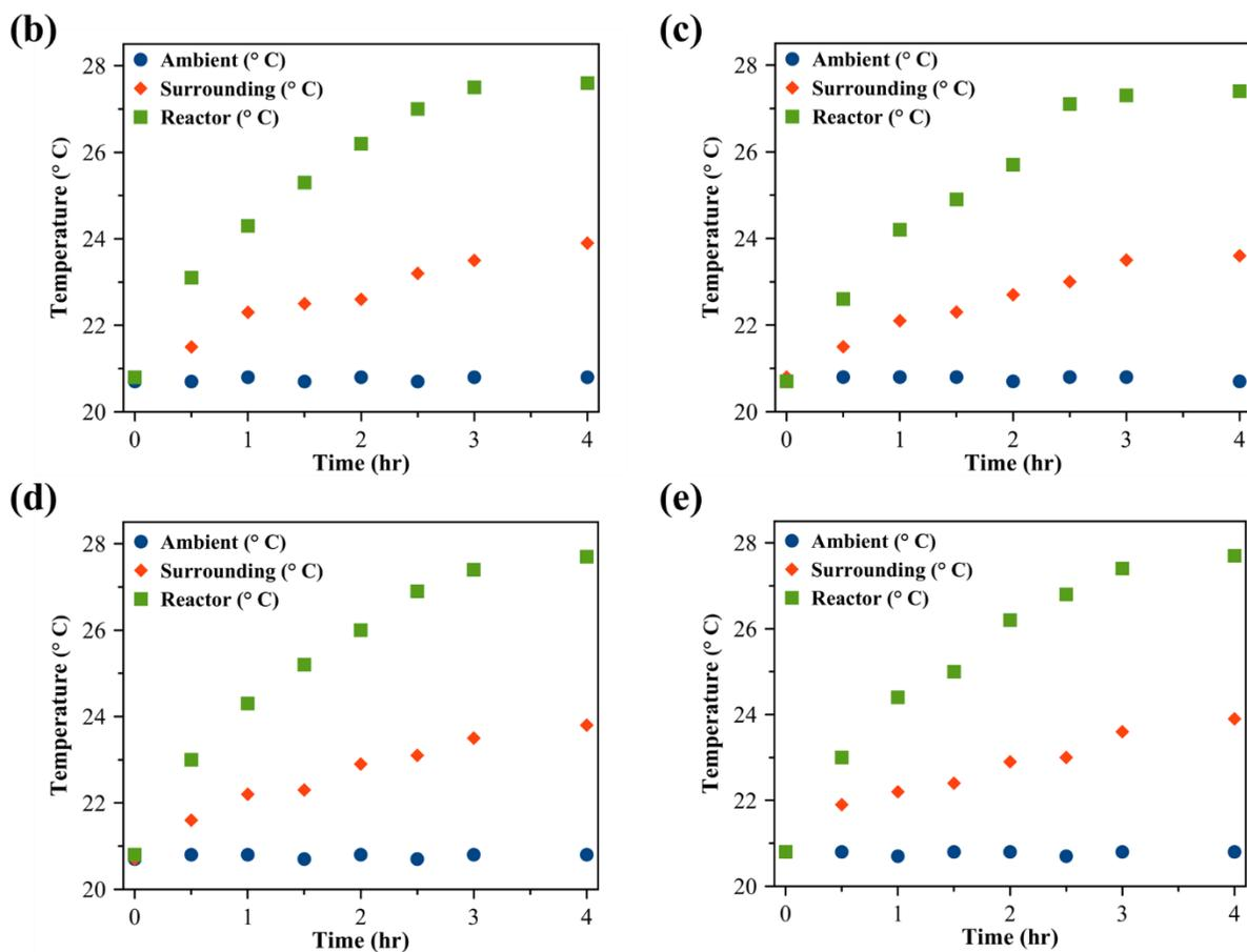
**Figure S3b-e.** Temperature profile measured as a function of irradiation time during photocatalytic degradation of MB for different conditions: **(b)** using  $\text{Cu}_2\text{O}$  nanospheres of  $42 \pm 6$  nm diameter, **(c)**  $\text{Cu}_2\text{O}$  nanocubes of  $92 \pm 13$  nm edge length. **(d)**  $\text{Cu}_2\text{O}$  nanocubes of  $286 \pm 47$  nm edge length. **(e)** using  $\text{Cu}_2\text{O}$  nanospheres of  $145 \pm 13$  nm diameter.
