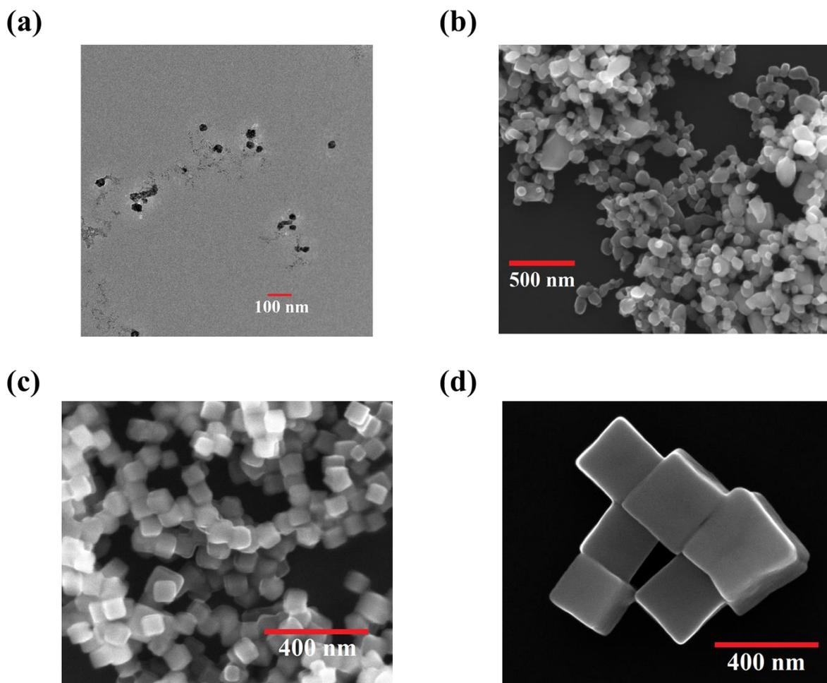
**Figure 2.** (a) Representative TEM image of smaller  $\text{Cu}_2\text{O}$  quasi-spherical nanoparticles of  $42 \pm 6$  nm diameter. (b-d) Representative SEM images of (b) larger  $\text{Cu}_2\text{O}$  quasi-spherical nanoparticles of  $145 \pm 13$  nm diameter, (c)  $\text{Cu}_2\text{O}$  nanocubes of  $92 \pm 13$  nm edge length, and (d)  $\text{Cu}_2\text{O}$  nanocubes of  $286 \pm 47$  nm edge length.
