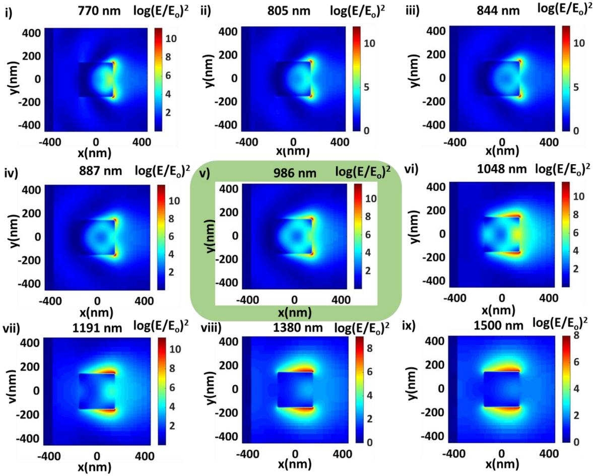
**Figure S4c (I).** FDTD-simulated spatial distribution of enhancement in electric field intensity  $[E^2/E_0^2]$  in XY plane at different wavelengths across the lowest energy Mie resonance peak wavelength (i.e., 986 nm) for  $\text{Cu}_2\text{O}$  cube of 286 nm edge length.
