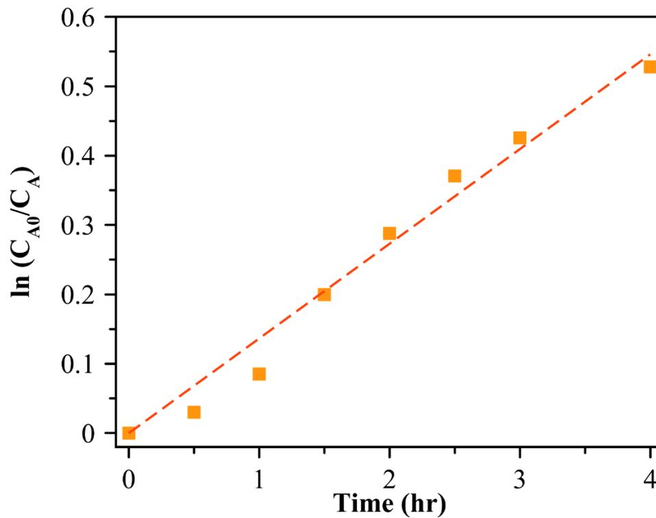
**Figure S5d.** Representative plot of empirical fit with first-order  $\ln(C_{A0}/C_A)$  versus irradiation time for photocatalytic degradation of MB under green light illumination using  $\text{Cu}_2\text{O}$  nanocubes of  $286 \pm 47$  nm edge length.
