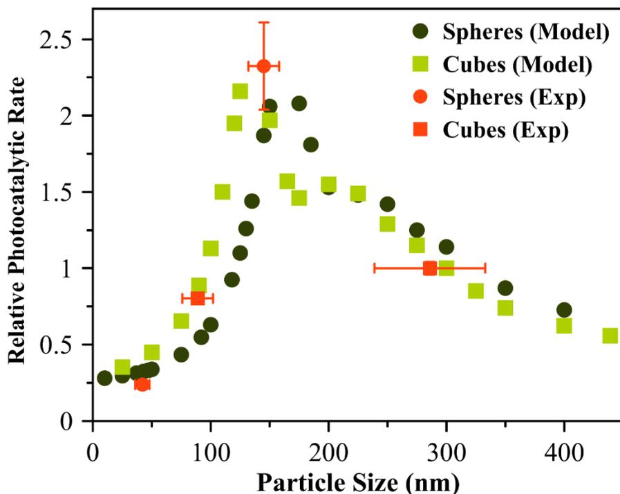
**Figure 5.** Volcano plot showing the predicted and experimentally measured relative photocatalytic rate as a function of size of Cu<sub>2</sub>O nanospheres and nanocubes. The photocatalytic rate on Cu<sub>2</sub>O nanocubes of 286 nm average edge length is used as a reference.
