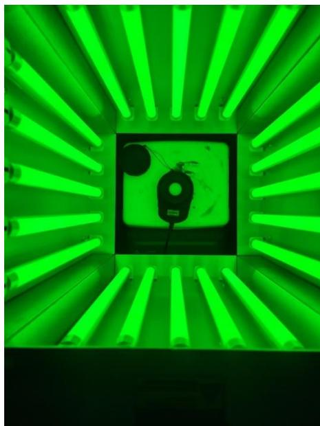
**Figure S2.** Photoreactor reactor set up of Luzchem Exposure Panels connected with green LED lamps.
