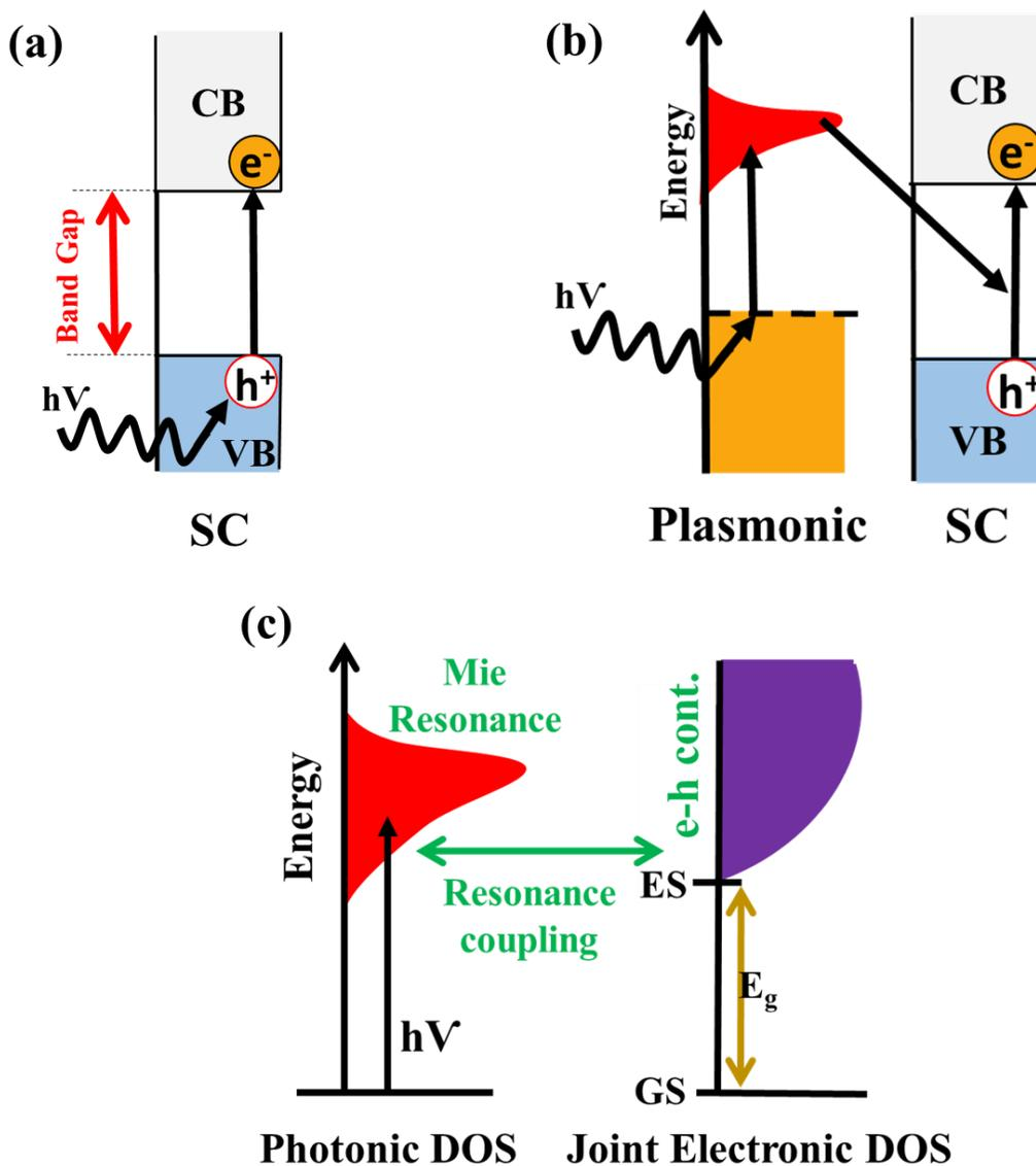
**Figure 1.** Schematic diagram illustrating (a) generation of a photoexcited electron-hole pair ( $e^-h^+$ ) in a semiconductor (SC), (b) plasmonic resonance-mediated generation of excited electrons and holes in a SC, and (c) the proposed dielectric resonance-mediated generation of excited electrons and holes in a SC. In (a), (b), and (c), excited electrons in the conduction band (CB) and excited holes in the valence band (VB) of SC can drive reduction and oxidation reactions.
