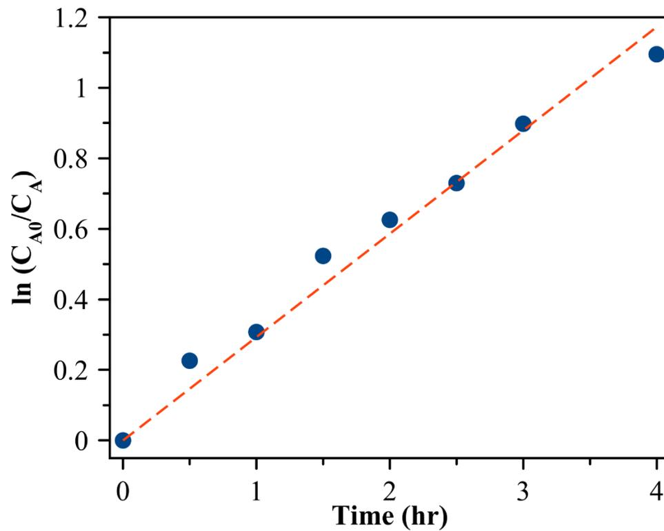
**Figure S5e.** Representative plot of empirical fit with first-order  $\ln(C_{A0}/C_A)$  versus irradiation time for photocatalytic degradation of MB under green light illumination using  $\text{Cu}_2\text{O}$  nanospheres of  $145 \pm 30$  nm diameter.
