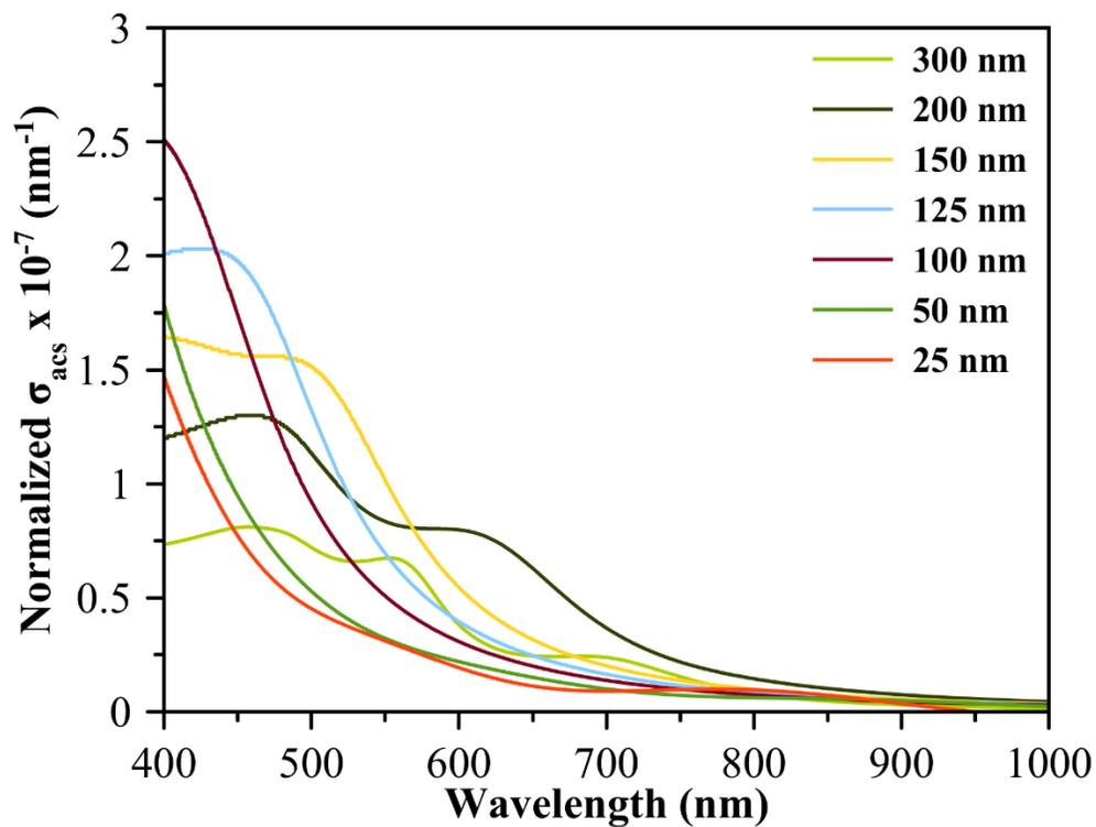
**Figure S5a.** FDTD-simulated volume-normalized absorption cross section ( $\sigma_{acs}$ ) as a function of incident light wavelength for  $\text{Cu}_2\text{O}$  spherical nanoparticles of different sizes.
