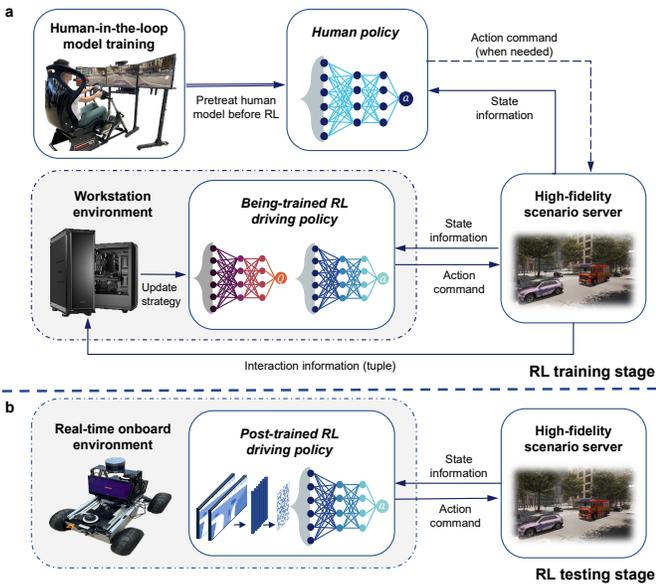
Fig. 6. Experimental workflow. a, the experimental workflow in the RL training stage. The dotted line represents the human policy model that is not always sending commands. b, the experimental workflow in the RL testing stage.
