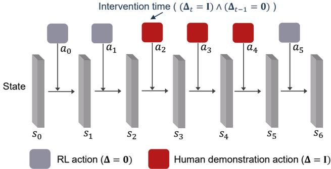
Fig. 2. Illustration of the intervention time step. In a time-sequential MDP, the first time step which is controlled by human demonstration is taken as the intervention time.
