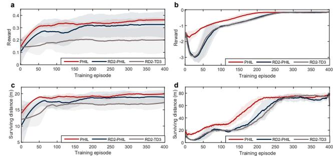
Fig. 13. Learning efforts of experience replay mechanism with different buffer structure. a-b, the training rewards of algorithms with different experience replay structures in the left-turn scenario and congestion, respectively. c-d, the training surviving distances of algorithms with different experience replay structures in the left-turn and congestion scenario, respectively.
