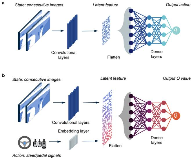
Fig. 5. Neural network approximator illustration. a, the policy function architecture achieved by the neural network, where the target value network owning the same structure is omitted for brevity. b, the value network architecture achieved by the neural network, where the target value network owning the same structure is omitted for brevity.
