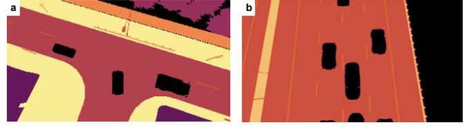
Fig. 4. State space illustration: bird's-eye-view semantic graph. a, the left-turn scenario, b, the congestion scenario.
