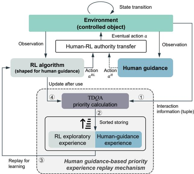
Fig. 1. Framework of the proposed human-guided reinforcement learning. The RL algorithm in this report is shaped in multiple aspects to adapt to human guidance. In the proposed human guidance-based priority experience replay mechanism, TDQA represents the proposed priority calculation scheme, and the number 1-4 indicates the flow sequence of data. The dotted line of the action signal represents that the framework allows intermittent human-in-the-loop guidance.
