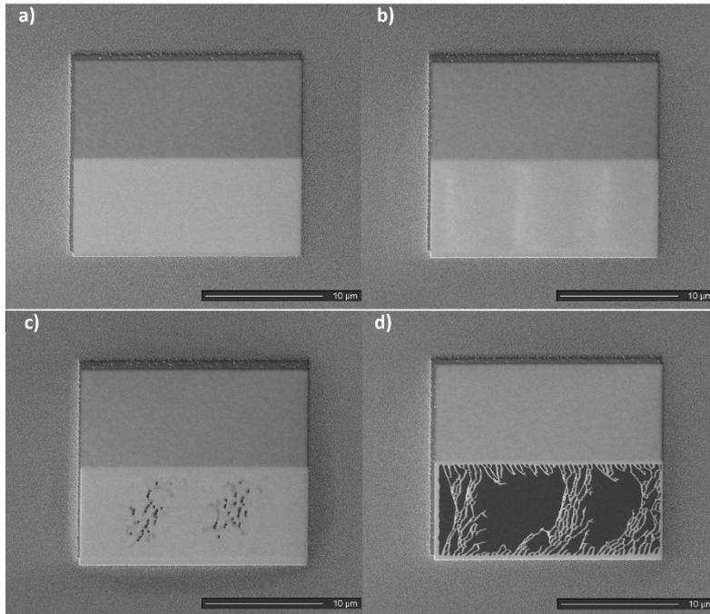
*Figure 16: SEM images illustrating fabrication of the pattern shown in Fig. 15 on a  $\text{Si}_3\text{N}_4$  membrane. From a) to d), the total milling time and number of repetitions were increased linearly. The pixel size was  $\sim 30$  nm, the ion current was  $\sim 104$  pA and the accelerating voltage was 30 kV. A low electron energy was used to enhance surface sensitivity during imaging.*
