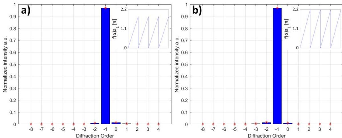
Figure 26: Diffraction intensity distributions for phase mismatches of a)  $-10\%$  and b)  $+10\%$ . The insets show the corresponding groove profiles.
