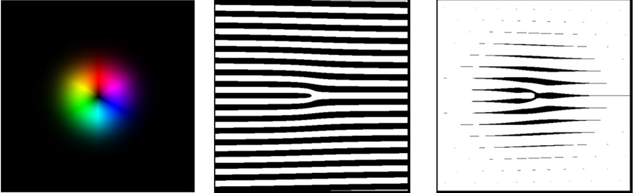
*Figure 14: Example of encoding the amplitude and phase of a Laguerre Gauss beam ( $\ell = 1$ ,  $p = 0$ ) in an amplitude hologram. The phase encoding gives the pitchfork, but the change in groove width gives the amplitude envelope.*
