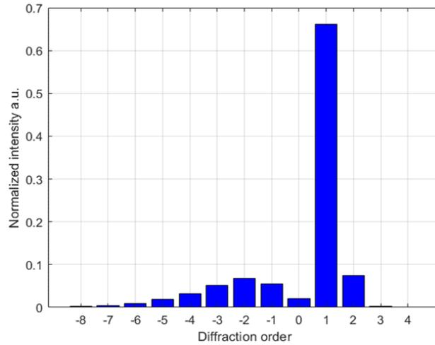
Figure 25: Experimental distribution of diffraction intensities in the best-performing sample, with the total intensity normalized to unity.
