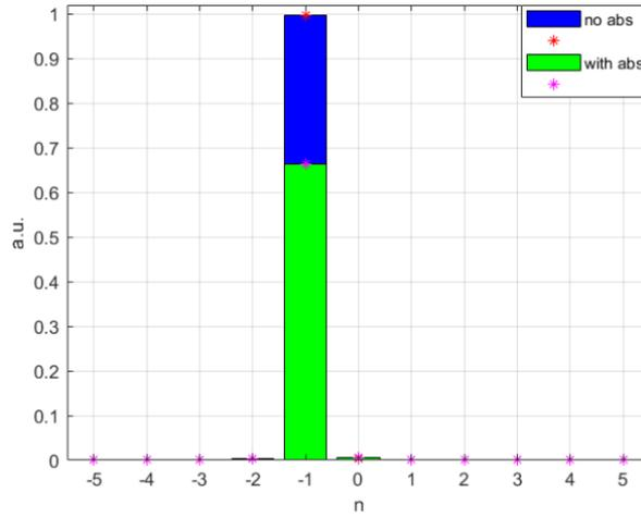
Figure 10: Comparison between  $|\tau_n|^2$  for different diffraction orders for the ideal case of a blazed phase S-CGH and a “real case” with absorption. In the ideal case, only the minus one order survives and all others ideally have zero intensity. If absorption is considered,  $\mathcal{T}$  is no longer unitary.
