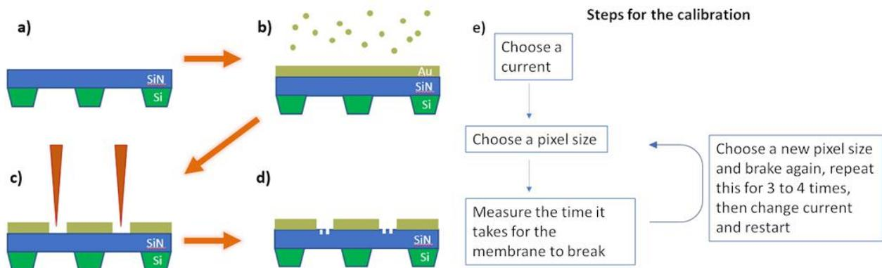
Figure 17: Schematic diagrams showing the typical steps in the fabrication of an S-CGH using FIB milling: (a) Fresh device; (b) Au evaporation; (c) Au removal and FIB patterning; (d) Grooves in the membranes; (e) Simple algorithm for the calibration process.
