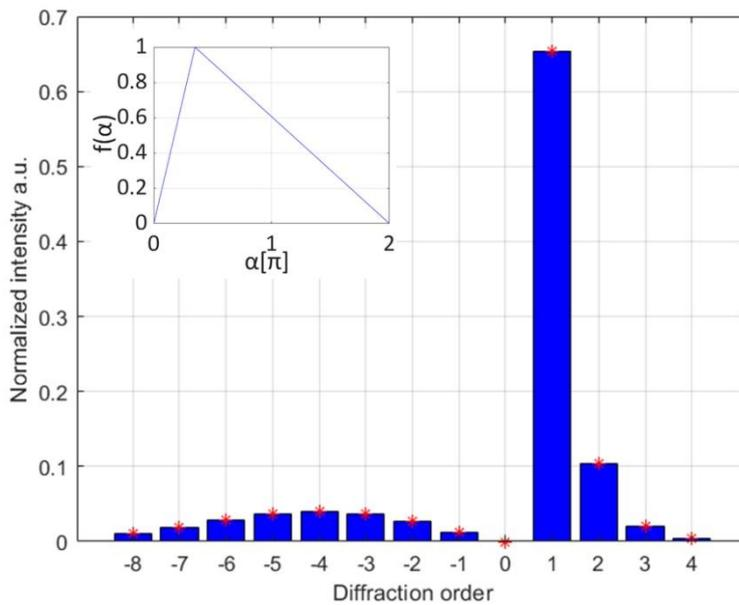
Figure 27: Diffraction intensity distribution for a scalene triangular profile for  $s=1.1$ .
