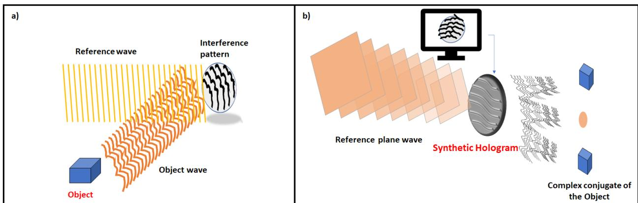
Figure 1: Schematic diagram of a) traditional “image” holography and b) “synthetic” holography.
