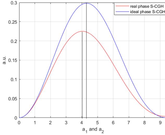
Figure 7:  $|\tau_1|^2$  for a triangular profile (Fig. 8) plotted for a phase S-CGH as a function of  $a_1$  and  $a_2$ .
