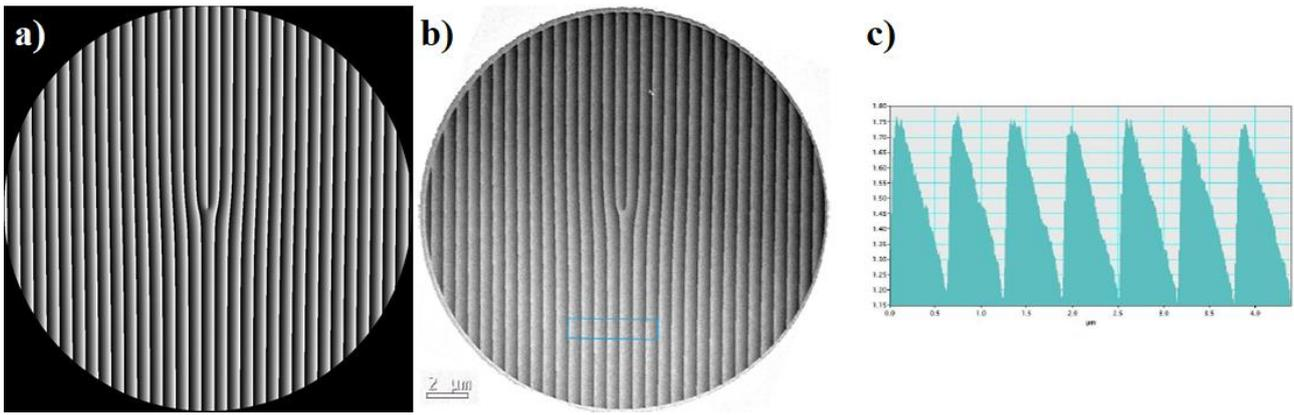
Figure 24: a) CGH for a blazed  $\ell = 1$  pitchfork; b) EFTEM thickness map of the fabricated S-CGH; c) Profile of the region marked by a blue rectangle in b).
