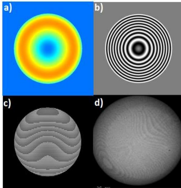
Figure 32: Design of a holographic  $C_s$  corrector. a) Desired phase plate; b) Inline S-CGH with a sinusoidal groove for  $\Delta f = 400$  nm; c) Off-axis S-CGH; d) Realization in silicon nitride.
