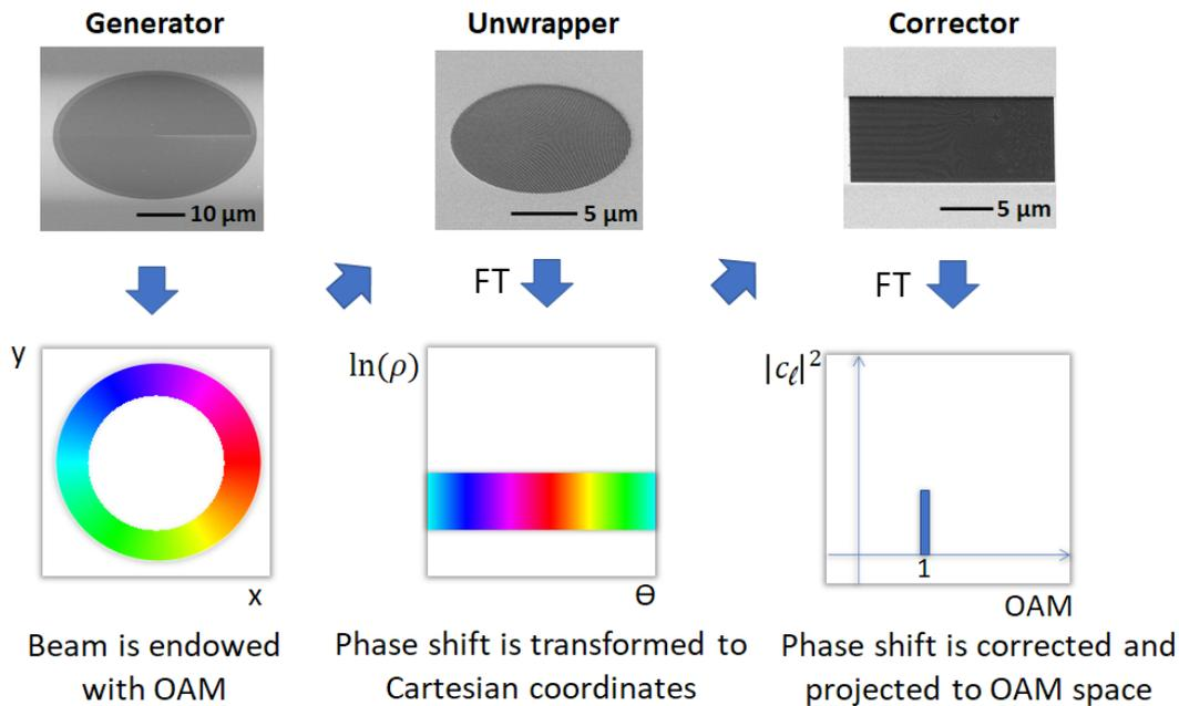
Figure 30: Sequence of holographic masks and transformations involved in the use of an OAM sorter.
