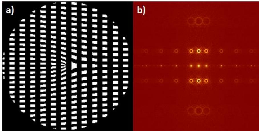
*Figure 21: a) Example of an amplitude S-CGH with a grid-like structure for improved mechanical stability; b) The resulting diffraction pattern, which forms a two-dimensional array of beams [36].*
