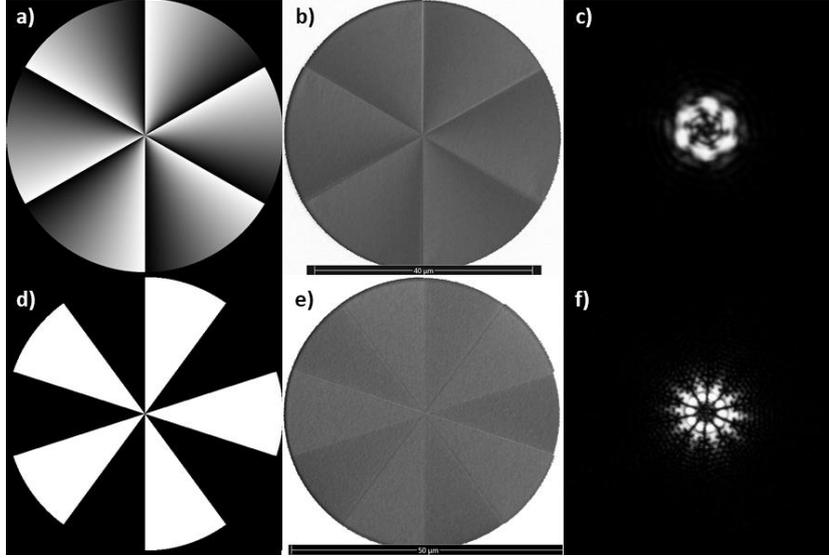
Figure 22: a) Phase of an EVB used to fabricate a phase-S-CGH with a spiral/ helical design for EVB generation for  $l = 6\hbar$ . The phase varies from 0 (black) to  $2\pi$  (white) and goes from 0 to  $12\pi$  over a complete revolution. (b) SEM image of a phase S-CGH corresponding to a). c) Experimental EVB in the Fraunhofer plane. d) Phase and e) phase S-CGH for an EVB with  $l = \pm 5\hbar$ . f) Experimental EVB.
