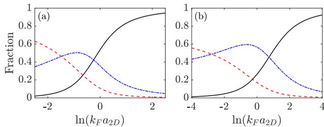
Figure 3. (Color online) The normalized contribution of polaron wave functions in the three different channels with (a)  $\eta = 1$  and (b)  $\eta = 6.64$ . Here the three lines for  $|\gamma|^2$  (solid black line),  $\sum_{\mathbf{q}} |\alpha_{\mathbf{q}}|^2$  (dashed red line) and  $\sum_{\mathbf{k}, \mathbf{q}} |\beta_{\mathbf{q}}|^2$  (dashed-dotted blue line) represent the bare impurity, molecule and particle-hole excitation, respectively.
