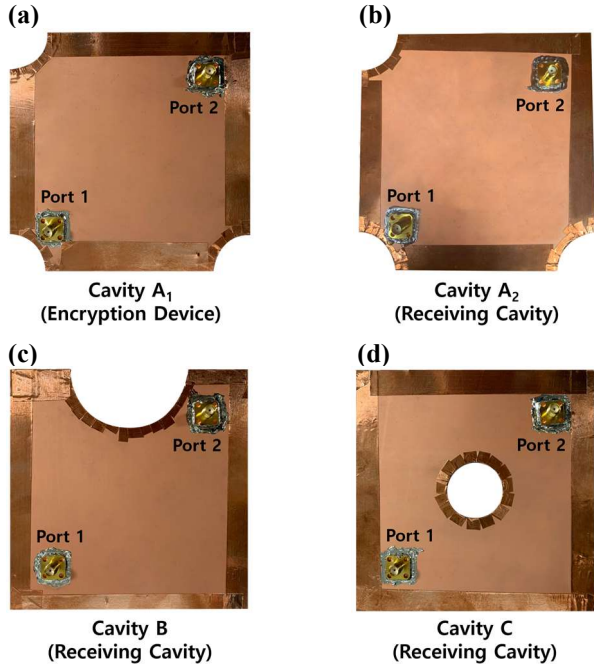
FIG. 2. Fabricated three different wave-chaotic cavities used in experiment: (a) Cavity A 1 for encryption on the transmit side (Alice). (b) Cavity A 2 for legitimate decryption (Bob). (c) Cavity B and (d) Cavity C for decryption in eavesdropping (Mallory).
