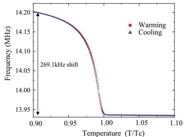
FIG. 3. Frequency response measured for the magnetic susceptibility of high-temperature superconductor  $\text{MgB}_2$ . The fractional change in frequency corresponds to a filling factor of 3.8%.
