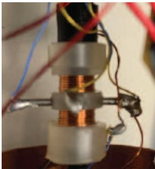
FIG. 2. Picture of Kel-F sample cell showing the Helmholtz coil pair (5 mm diameter) and the electrodes for generating an electric field across the sample (typically 1 mm in lateral dimension). The sample is thermalized by applying Apiezon N-grease which makes contact with the thermal board.
